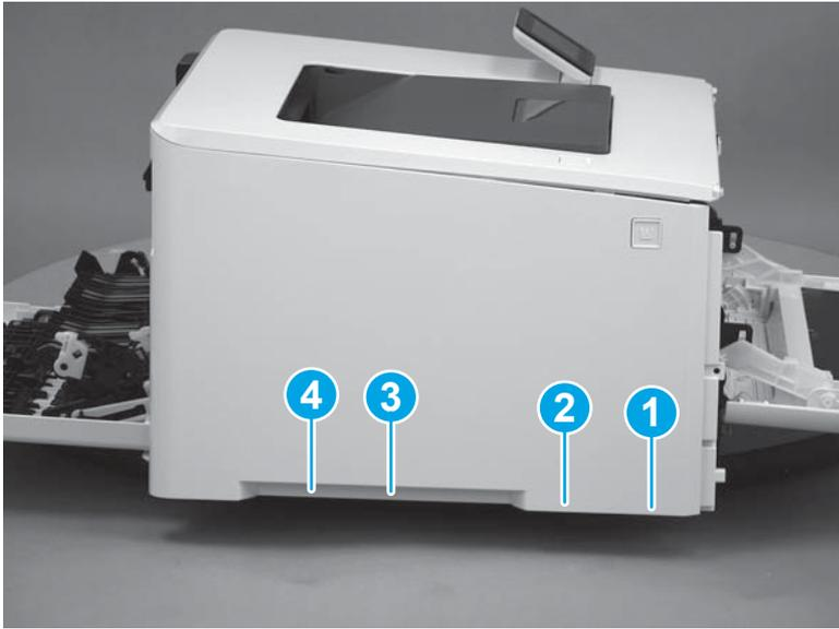
5. Release three tabs at the top of the cover (callout 1), and then slide the cover toward the rear of the printer to remove it.
