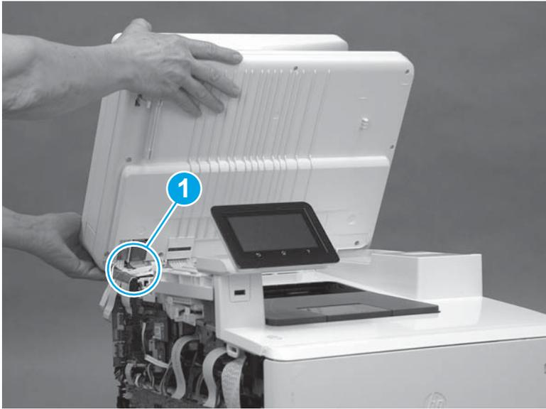
3. Install the tabs (callout 1) on the front of the scanner cable cover in the slots (callout 2) on the top cover.
