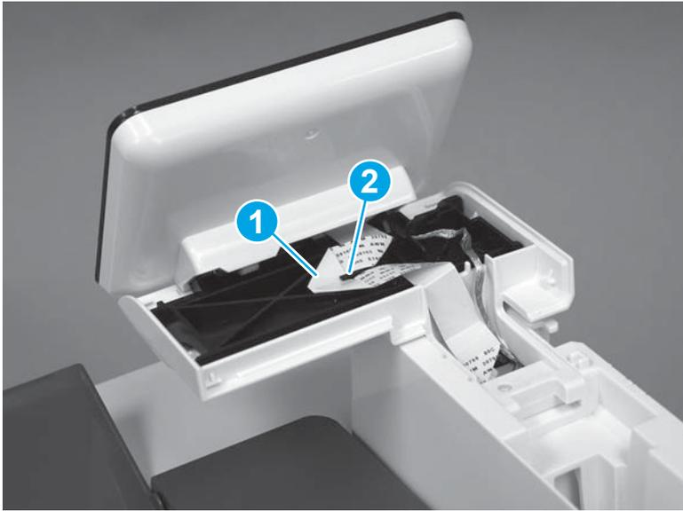
9. Remove two screws (callout 1), and then remove one screw (callout 2) and release one ground wire.
