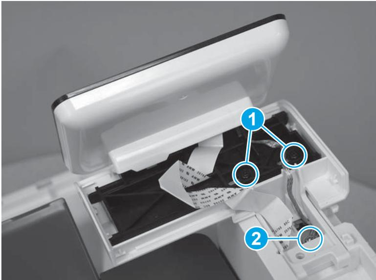
10. Carefully lift the control panel away and rest it on the top cover, and then remove one screw (callout 1).
