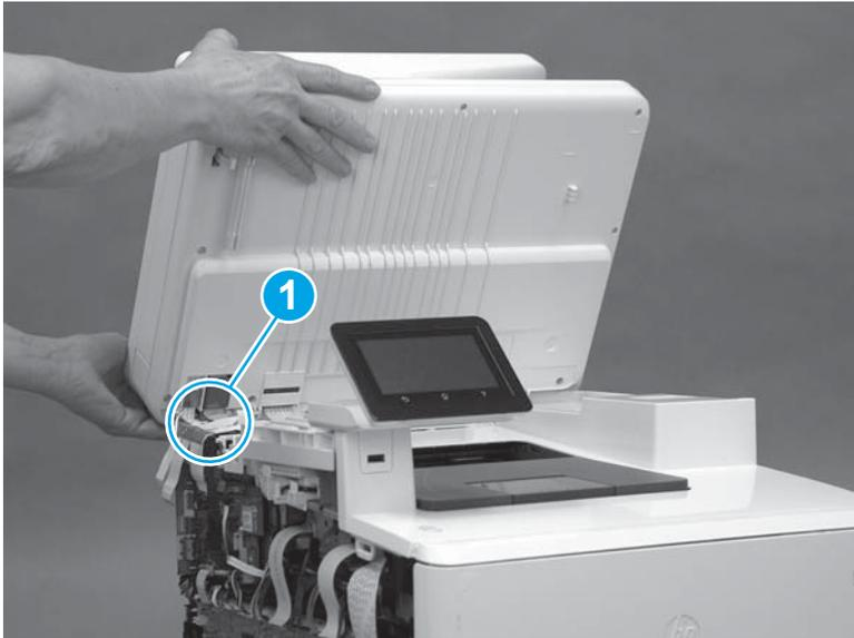
9. Open the scanner assembly fully, slide the assembly toward the right side of the printer, and then lift the assembly off of the printer.
