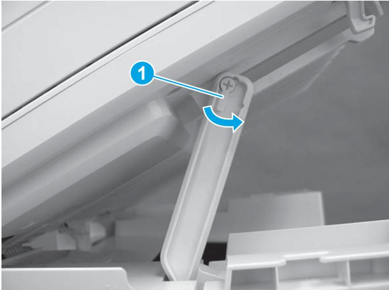
5. Remove the scanner arm pin.
