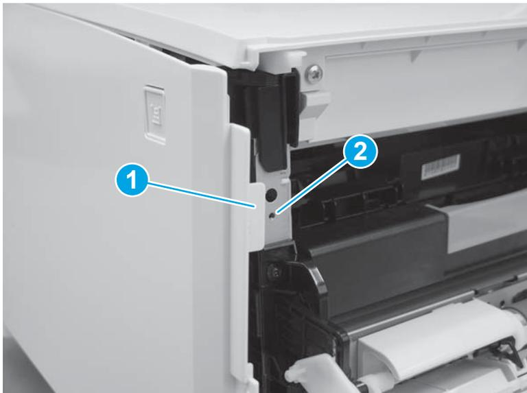
4. Slide the printer to the edge of a work surface in order to access the tabs on the bottom of the cover. Beginning from the back of the cover, install four tabs (callouts 1-4) on the lower edge of the cover.
