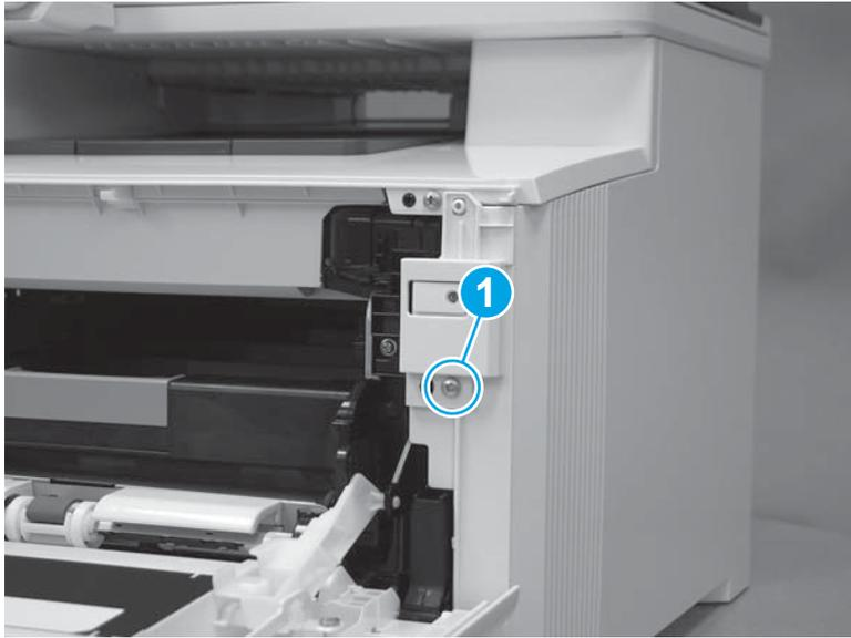
10. At the back of the printer, install one screw (callout 1).
