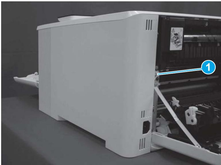
2. At the front of the printer, remove one screw (callout 1).
