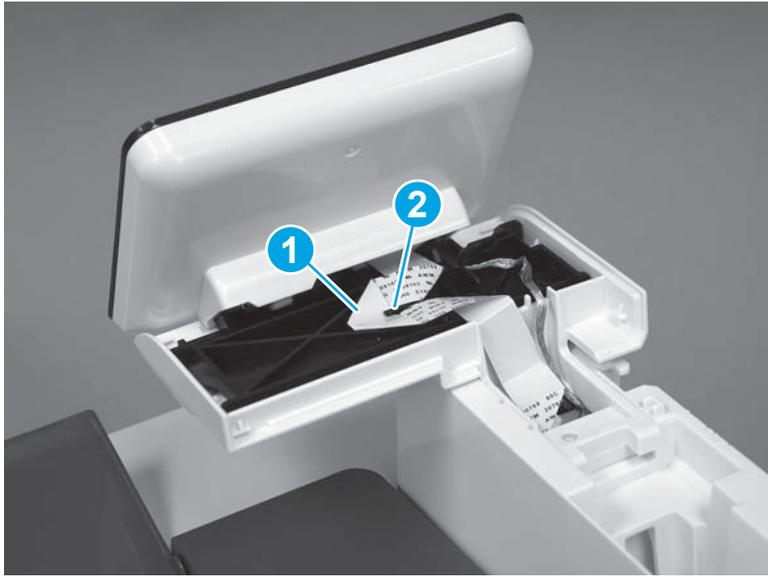
9. Install the control panel cover (callout 1) behind the control panel.
