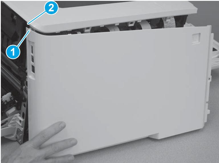
3. Slide the cover toward the front of the printer (callout 1), and then engage three tabs (callout 2) on the top of the cover.
