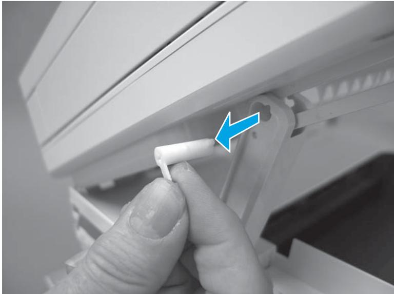
6. On the top of the printer, use a flat-blade screwdriver to release one tab (callout 1).
