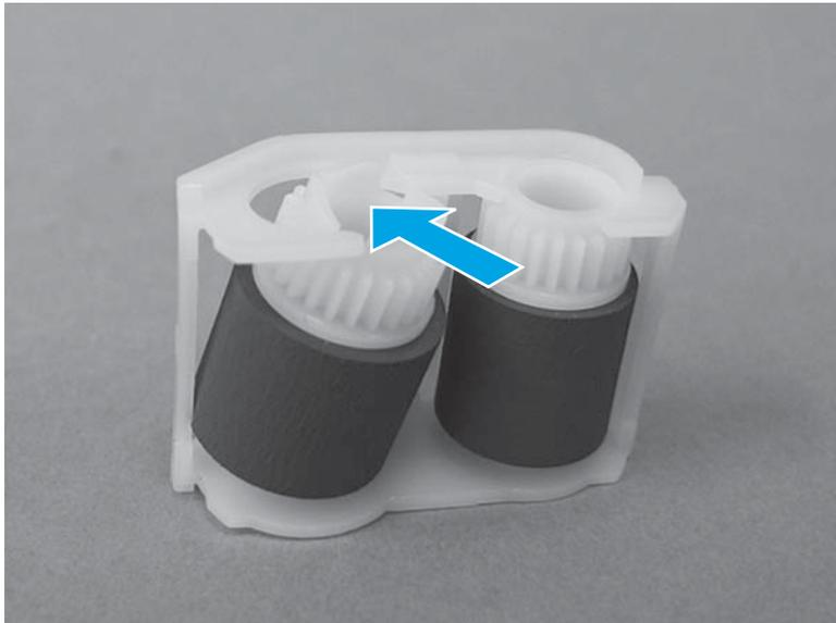
3. Install the ends of the rollers (callout 1) in the roller case over the shafts (callout 2) on the printer.
