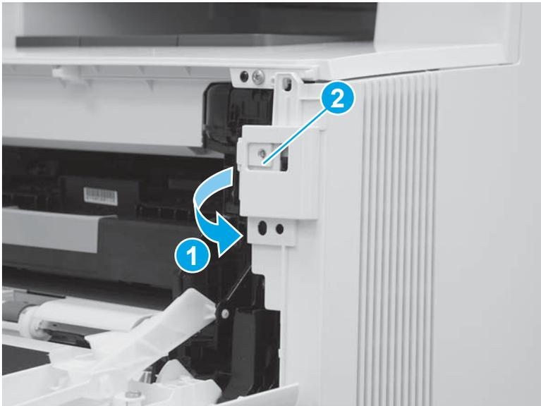
9. Slightly pull the front of the cover away from the printer (callout 1) to release one tab (callout 2).
