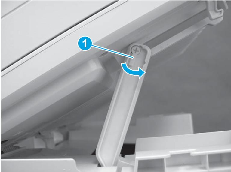
5. Remove the scanner arm pin.
