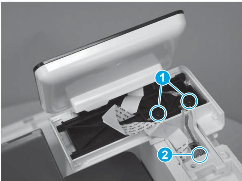
8. Install the flat cable (callout 1) under the retaining guide (callout 2).
