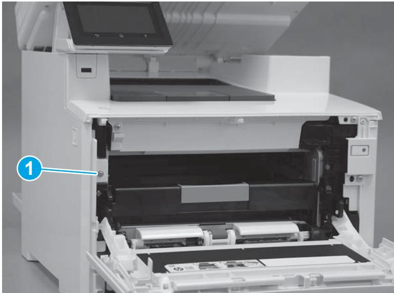
3. Release two tabs (callout 1) at the front of the cover. Hold the cover open to prevent the tabs from re-engaging.
