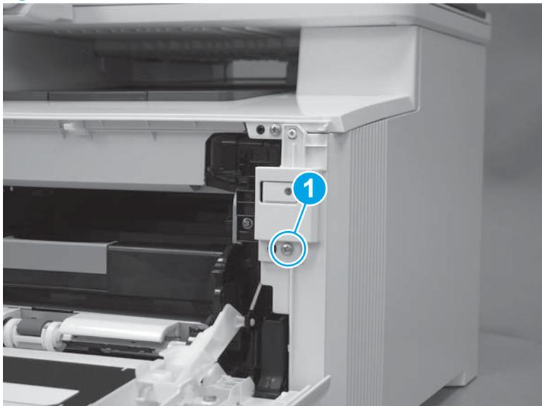
4. Slide the printer to the edge of a work surface. Note the location of the tabs on the lower edge of the cover (callout 1).
