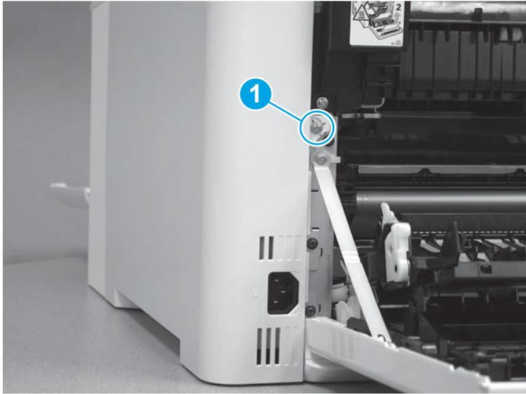
3. At the front of the printer, remove one screw (callout 1).
