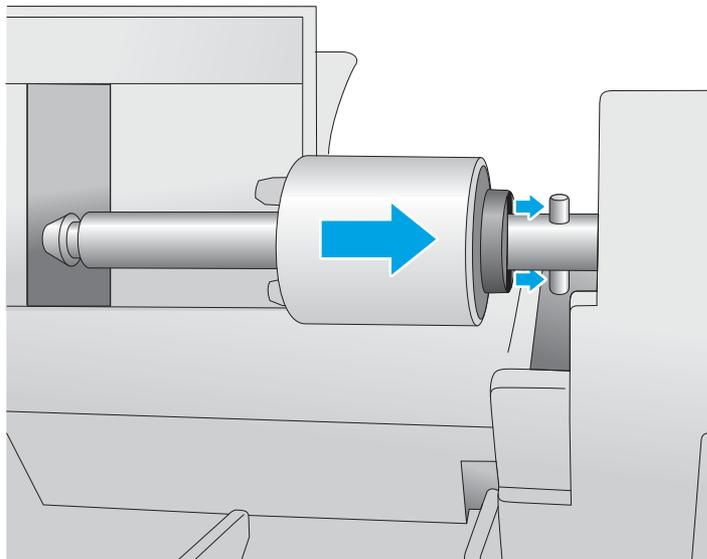
5. Slide the feed roller onto the shaft. You might have to rotate the roller while sliding it onto the shaft to make sure it clicks into place.
