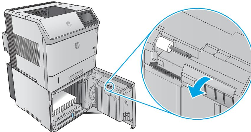
4. Before installing the feed roller, make sure that the torque limiter (the white plastic roller on the shaft next to the feed roller) is correctly positioned against the locking pins on the shaft.
