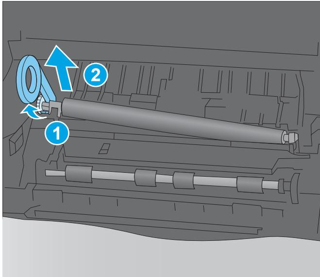
3. Slide the transfer roller to the left, and then lift up to remove it.
