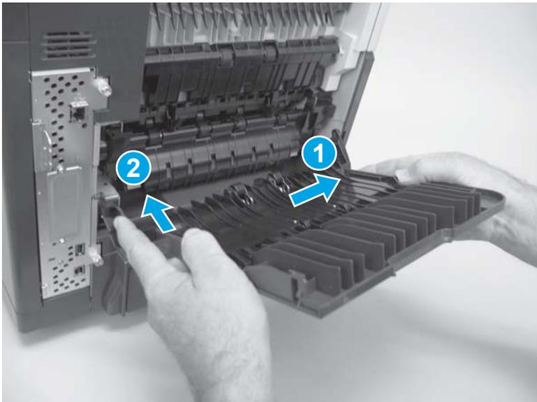
2. Make sure that the left hinge pin is installed in the mounting hole.
