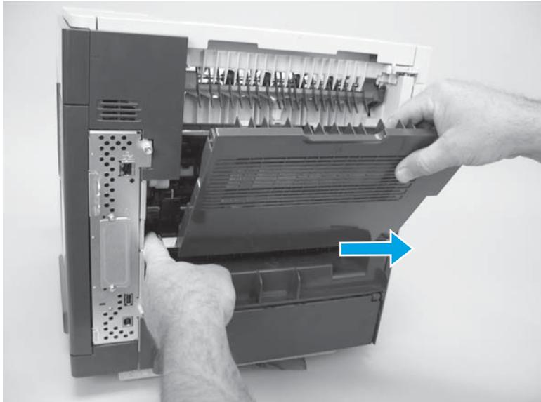
2. Rotate the output bin away from the printer (callout 1) until the right hinge pin is released, and then slide the output bin to the left (callout 2) to remove it.
