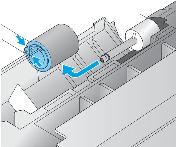
3. Inside the tray cavity, pinch the blue tab that is on the left side of the upper feed roller (callout 1), and then slide the roller off of the shaft (callout 2).
