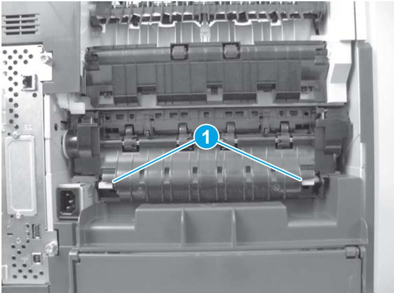
2. Pull the fuser straight back and out of the printer.
