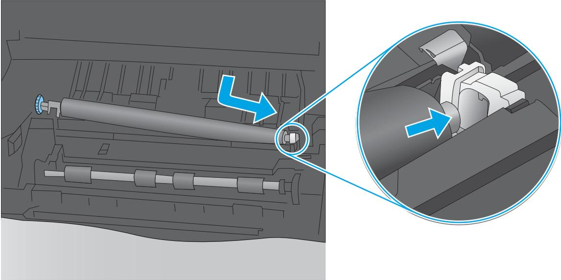
3. Lower the transfer roller into position on the left. Make sure that the collar on the left side is oriented correctly, with the open end face-down (the solid end is face-up).
