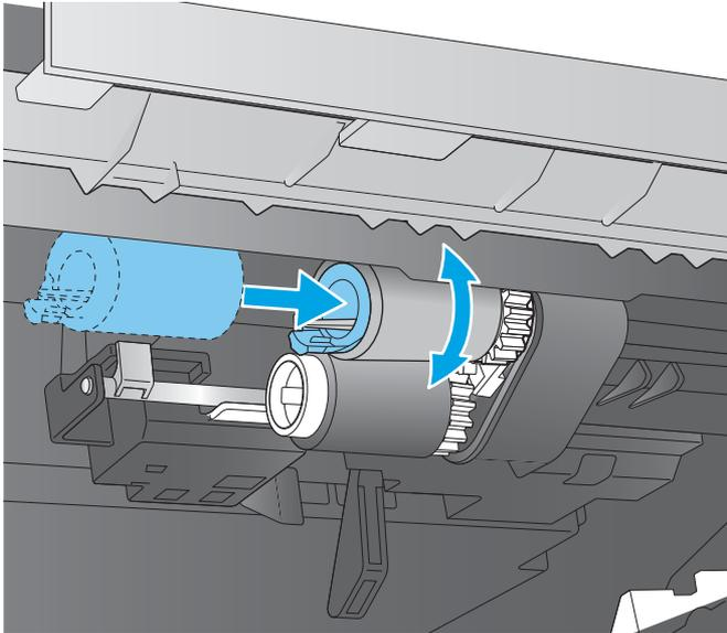
3. Open the spring-loaded cover that is next to the roller in the tray.
