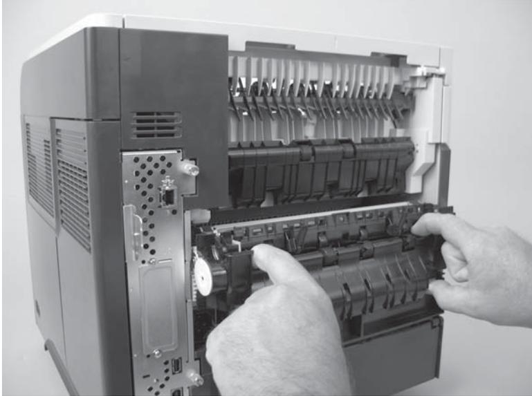
**Step 7: Install the rear output bin**
