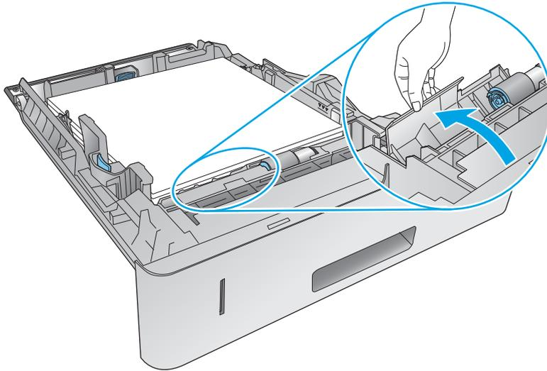
4. Before installing the feed roller, make sure that the torque limiter (the white roller on the shaft next to the feed roller) is correctly positioned against the locking pins on the shaft.
