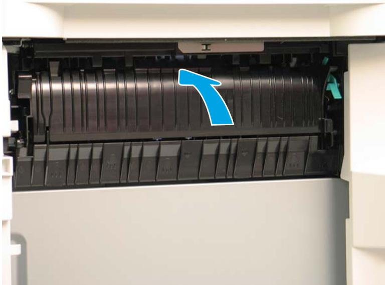
15. **M631z/M632fht/Flow M632z/FlowM633z printers only:** Close the right door of the paper feeder.
