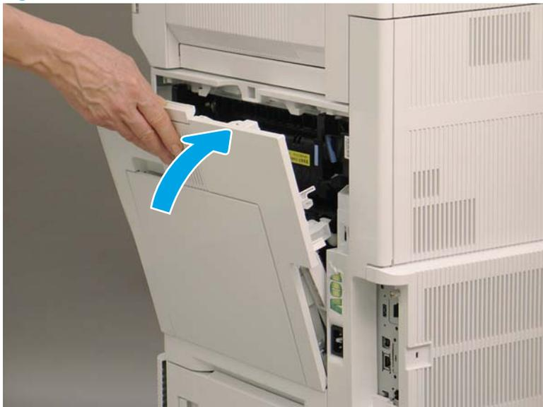
20. Close the paper tray for which the rollers were replaced.
