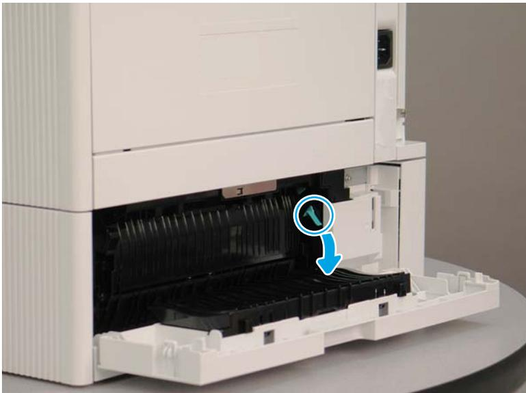
7. **M631z/M632fht/Flow M632z/FlowM633z printers only:** Open the right door of the paper feeder.
