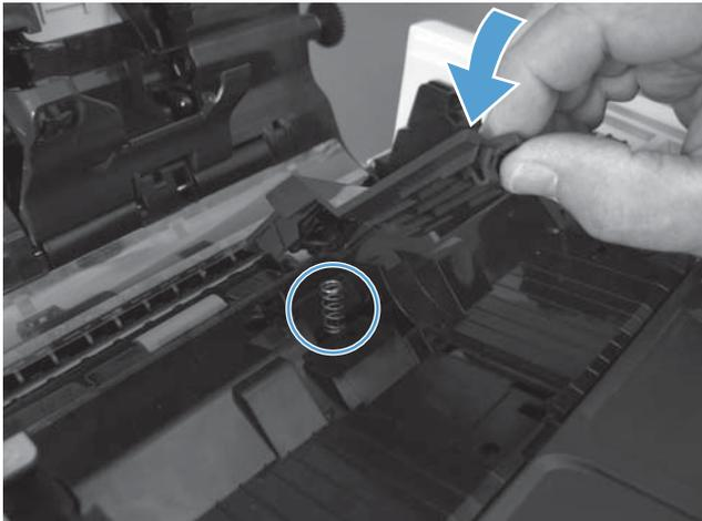
2. When the separation pad and holder is installed, make sure that the separation-pad spring (callout 1) is positioned under and behind the ridge (callout 2) on the bottom of the holder.
