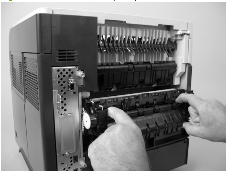
Figure 6-24 Remove the fuser (2 of 2)
