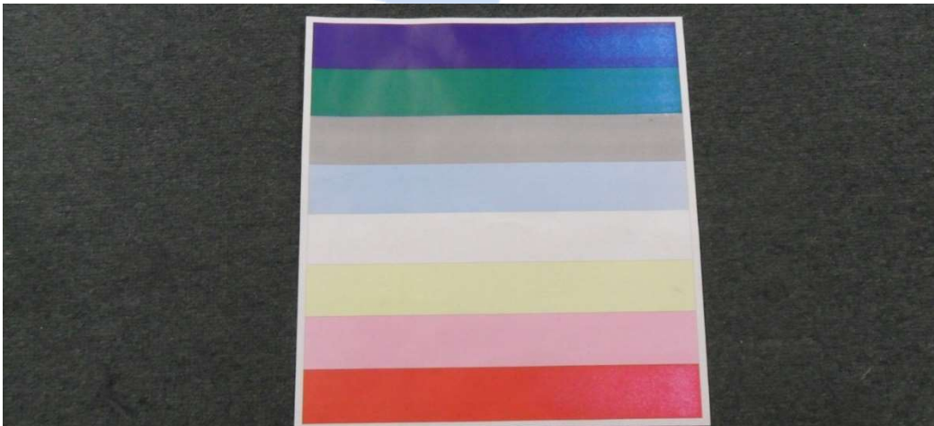
Figure 2: Example of “color band test” shown faded down right side from a printer that had the front tab broken.
