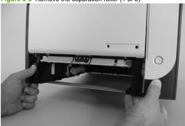
Figure 6-6 Remove the separation roller (1 of 3)
