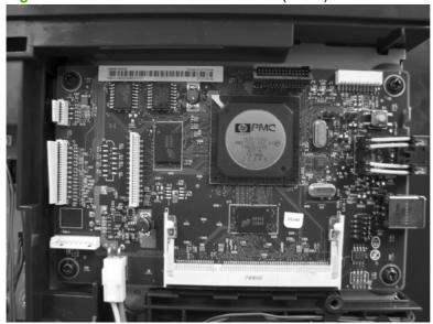
Remove four screws (callout 1), and then remove the formatter PCA.
