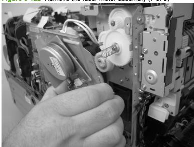
9. Remove three screws (callout 12), and then remove the fuser motor assembly.
