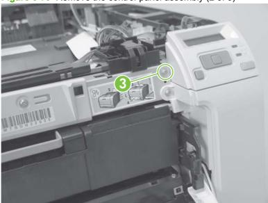
Remove the control-panel assembly.
