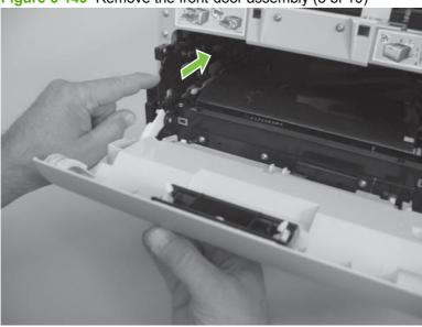
**10**. Support the door assembly, and carefully release the lower pin on the left-side link.
