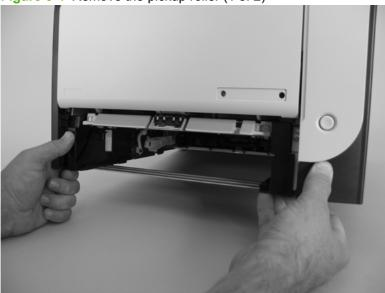
3. Release the two white plastic locking tabs and remove the pickup roller.
