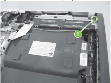
3. Slightly lift up on the cover, and then rotate the top of the cover away from the product.
