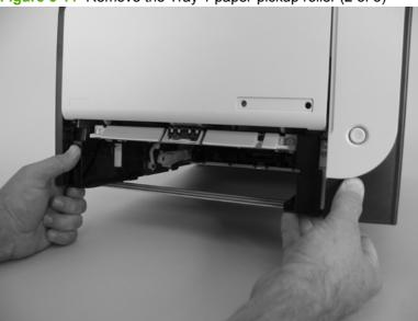
4. Release two tabs, and then rotate the roller away from the product to remove it.
