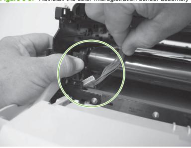
Use a small flat blade screwdriver to guide the connector through the hole.
