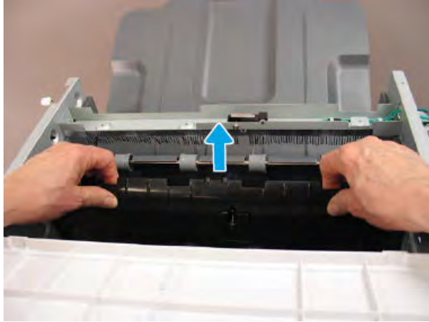
Figure 5-398 Remove the top lower feed assembly
