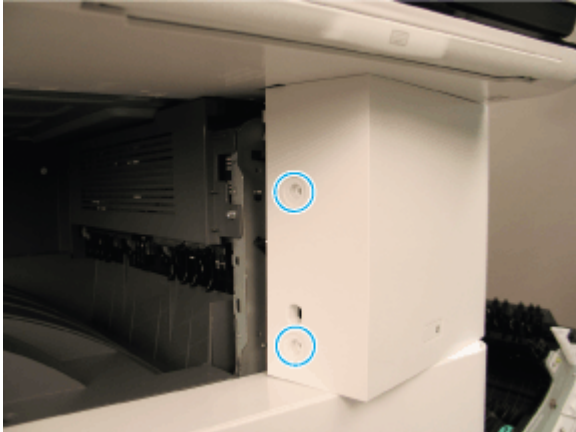
Figure 2-120 Remove the power-switch cover
