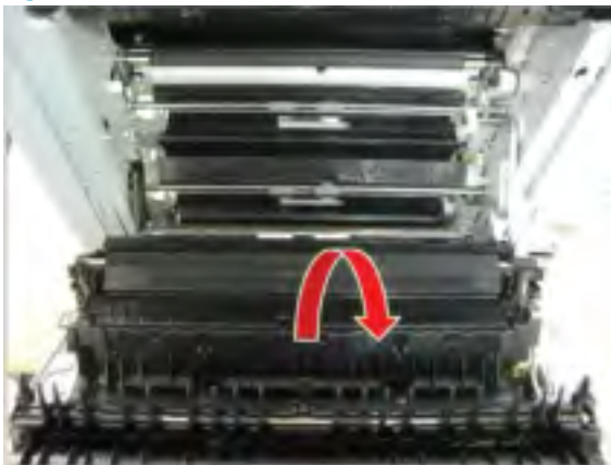
Figure 2-275 Remove right door
