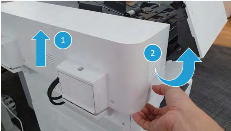
Figure 2-351 Release the top back cover.
