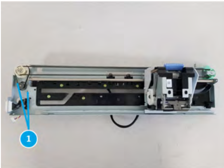
Figure 5-938 Remove two screws
