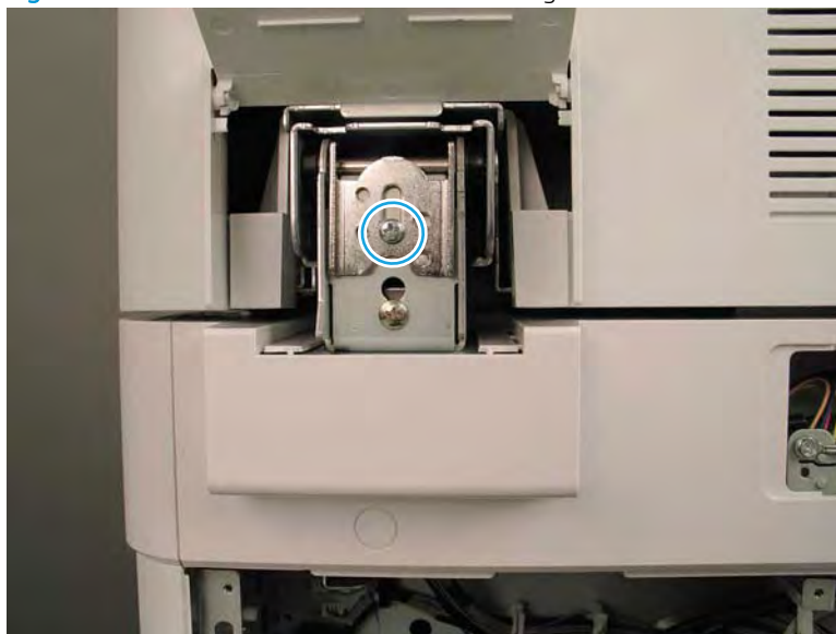
Figure 2-23 Release the document feeder hinge screws
