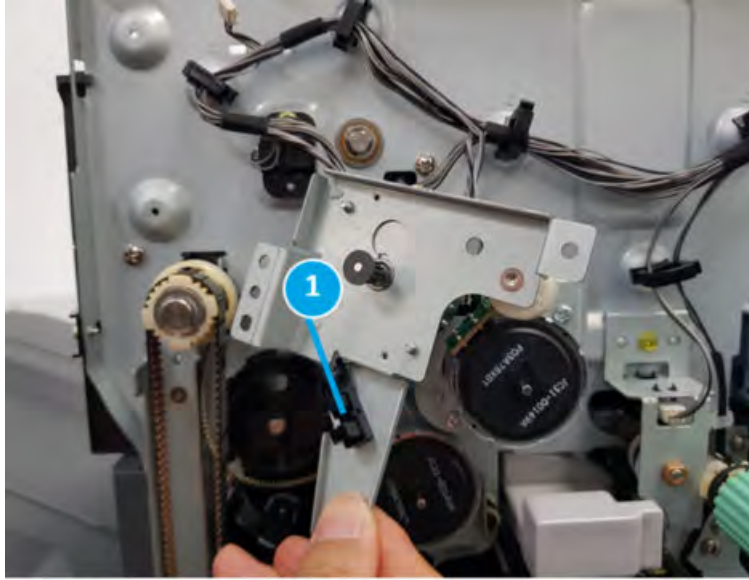
Figure 5-456 Remove paddle home sensor
