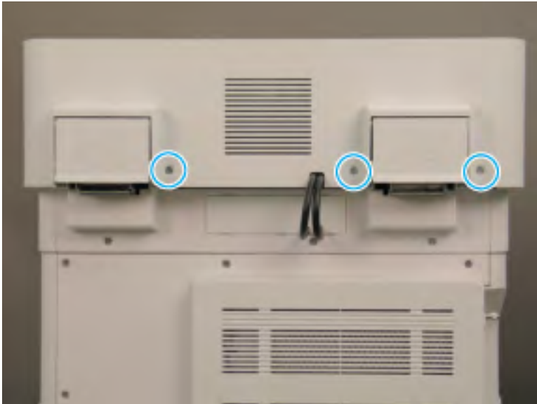
Figure 2-475 Remove the document feeder back cover bottom screws
