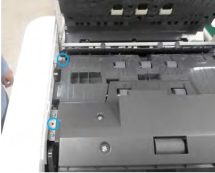
Figure 2-412 Remove the document feeder front cover top screws
