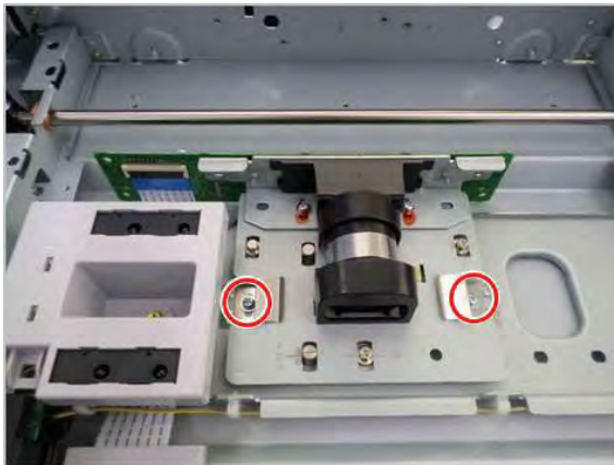
Figure 2-502 Remove screws and release scanner imaging unit
