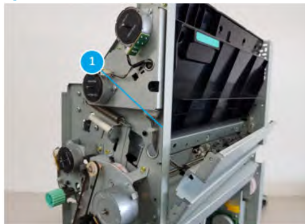
Figure 5-1760 Disconnect one connector
