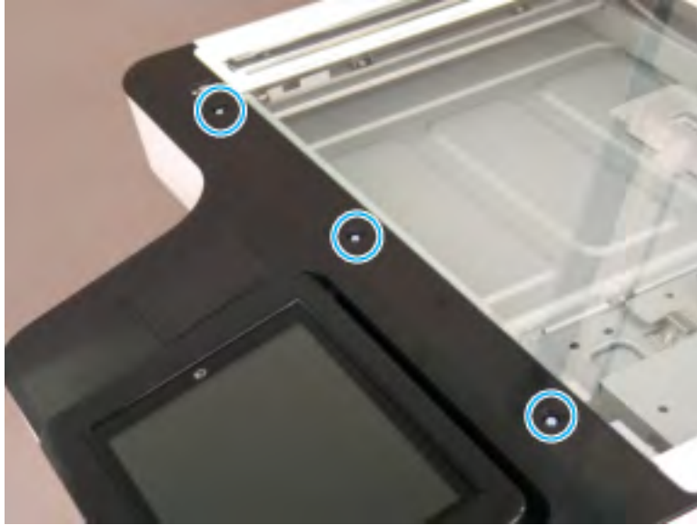
Figure 2-39 Remove three screws
