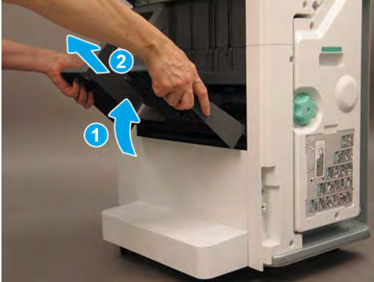
Figure 5-1322 Remove the booklet output tray
