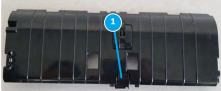
Figure 5-356 Remove one screw and then top lower feed assembly
