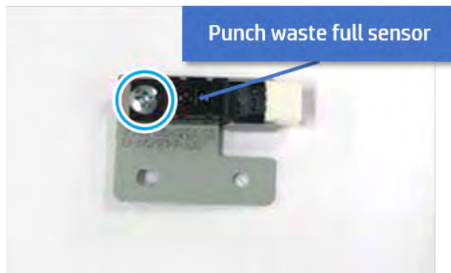
Figure 6-788 Remove the punch waste full sensor
