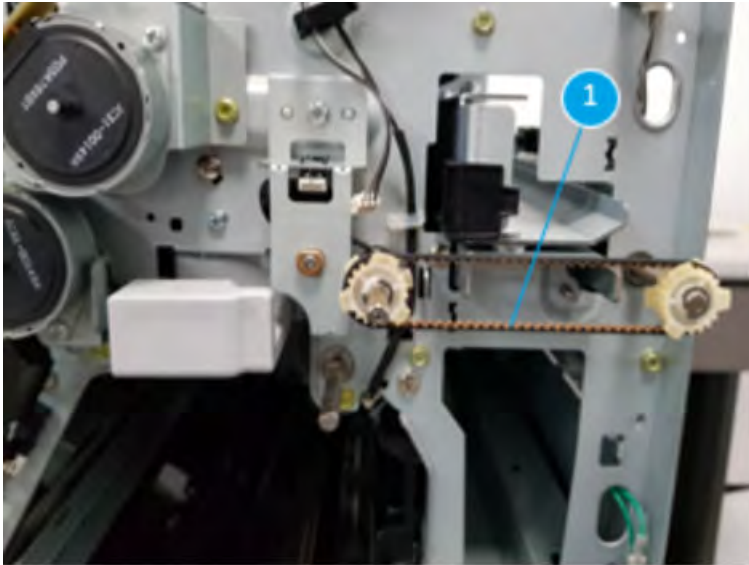
Figure 5-309 Remove the belt
