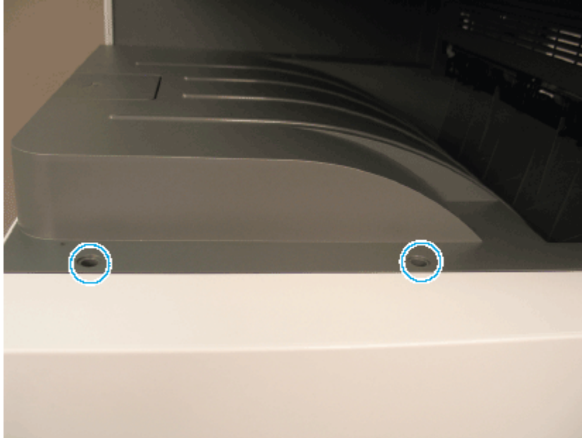
Figure 2-268 Remove screw-caps and screws
