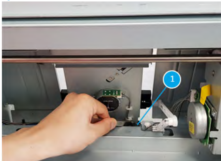
Figure 5-1521 Remove the Booklet end fence home sensor
