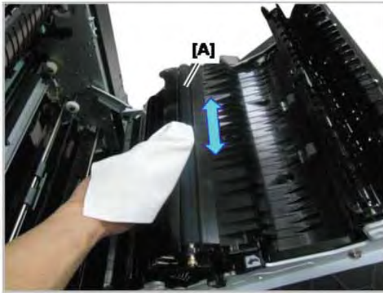
Figure 2-12 Transfer roller cleaning
