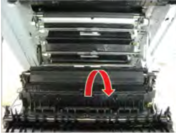
Figure 2-202 Remove right door
