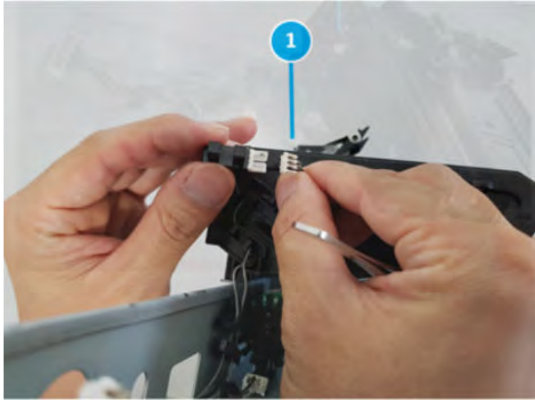
Figure 5-1119 Disconnect the connector from ejector2 home sensor
