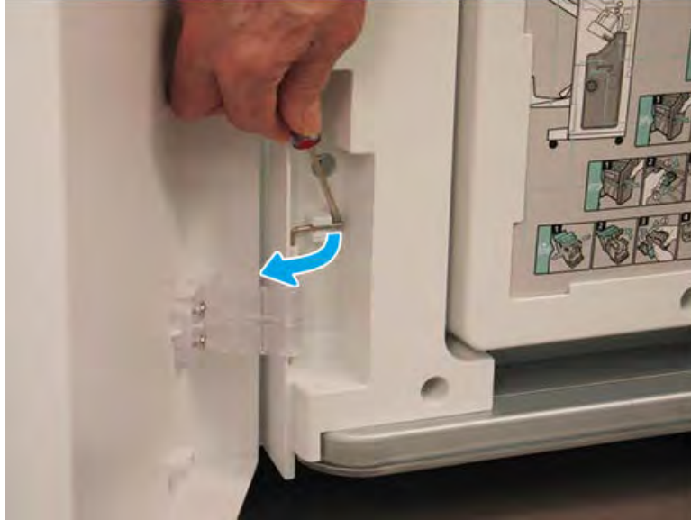
Figure 5-946 Release the lower hinge pin
