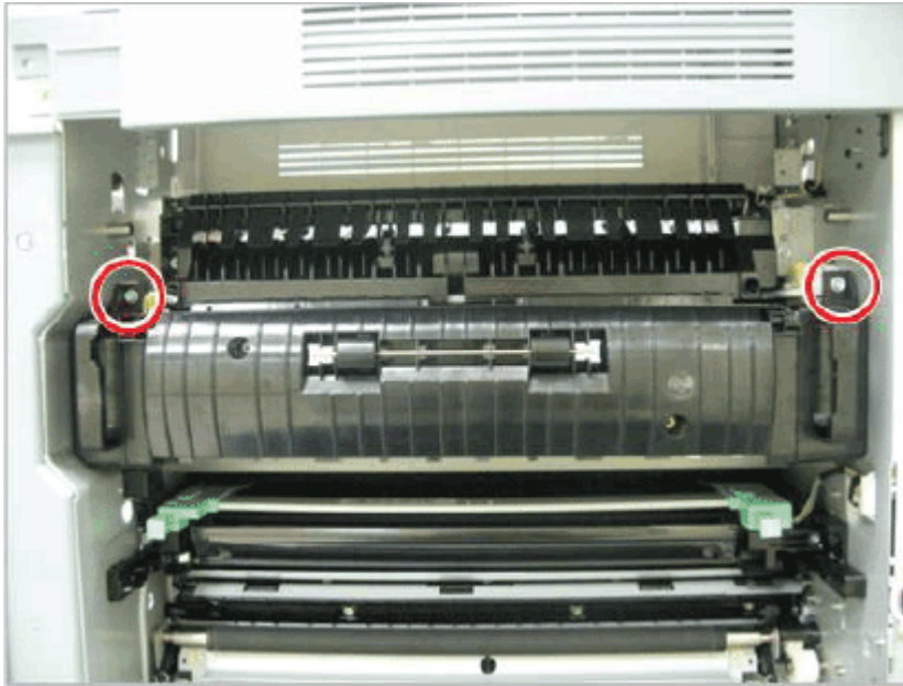
Figure 2-51 Remove two fuser unit screws
