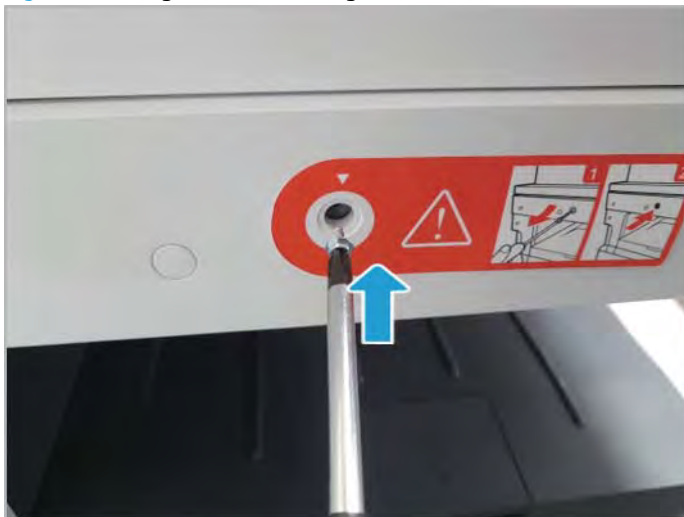
Figure 1-49 Tighten scan locking screw
