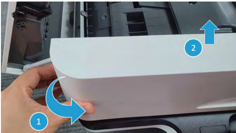
Figure 2-356 Remove the document feeder front cover
