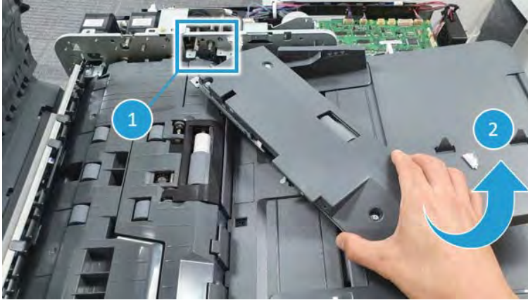
Figure 2-483 Remove the pickup roller assembly
