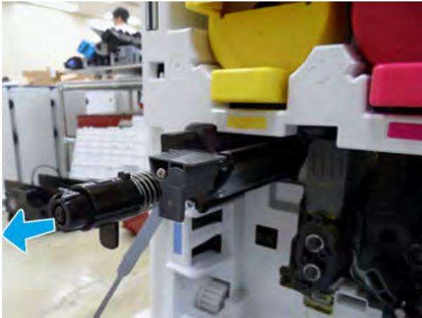
Figure 2-270 Release ITB cleaner
