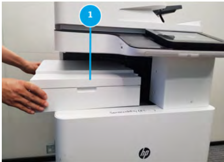
Figure 5-125 Pull out the bridge unit
