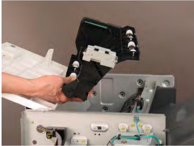
Figure 5-394 Remove the top jam access cover
