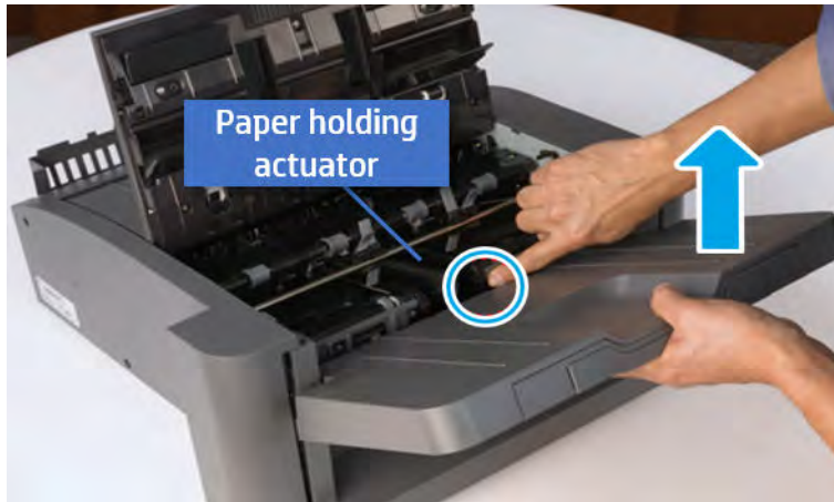
Figure 6-352 Remove the output tray.
