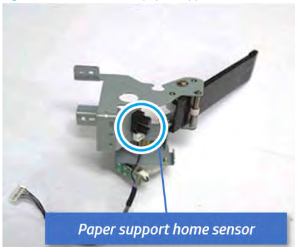
Figure 6-236 Remove the paper support home sensor
