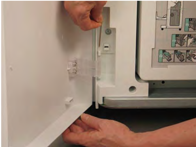
Figure 5-366 Remove the lower hinge pin
