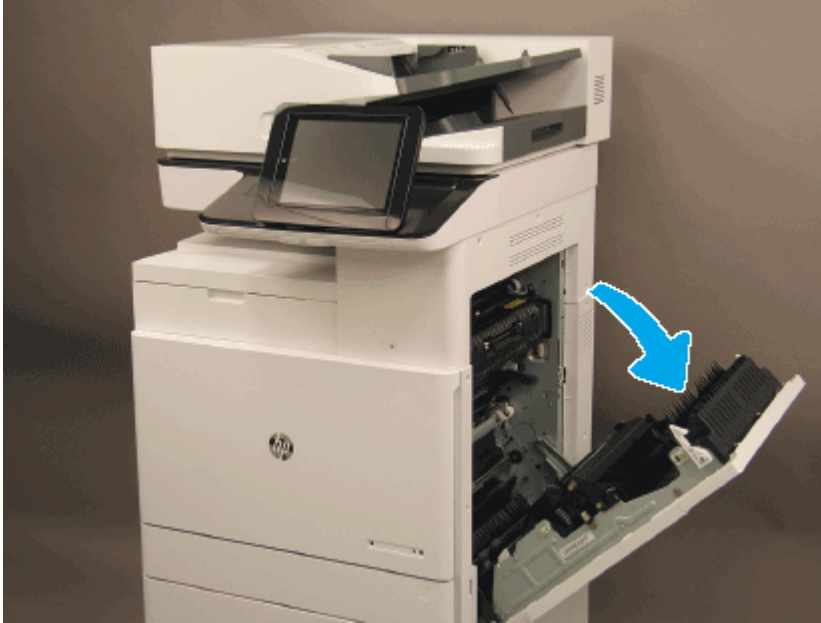
Figure 2-289 Open right door
