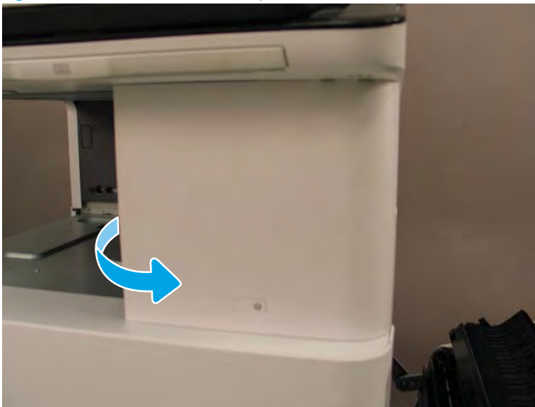
Figure 2-294 Remove the front top cover
