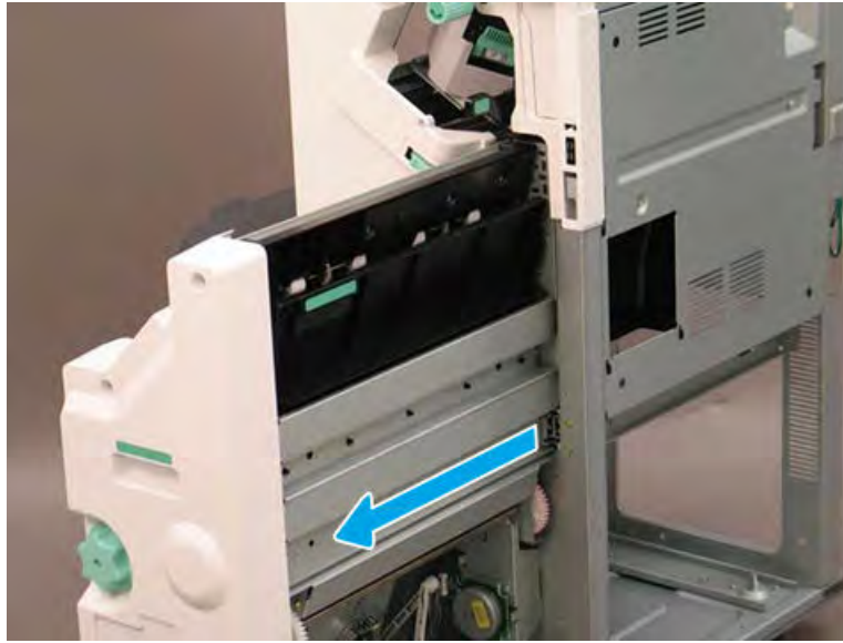
Figure 5-1443 Extend the right rail
