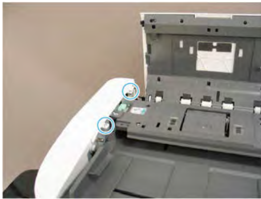
Figure 2-361 Remove the document feeder front cover top screws
