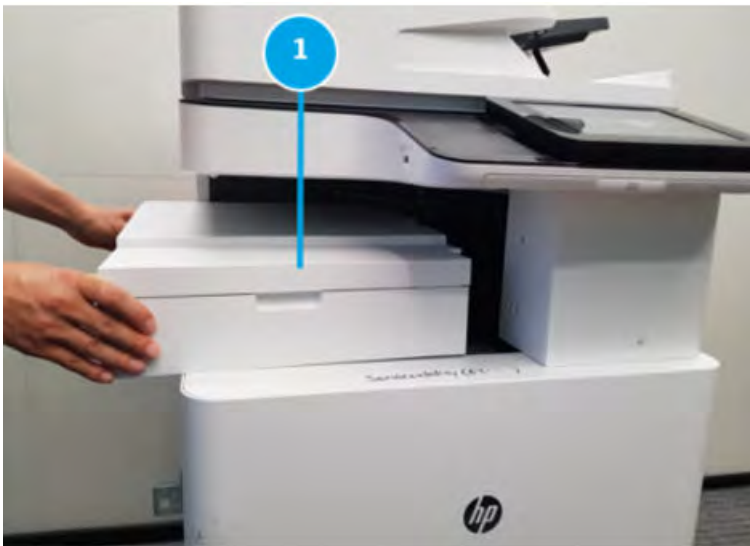
Figure 5-144 Pull out the bridge unit
