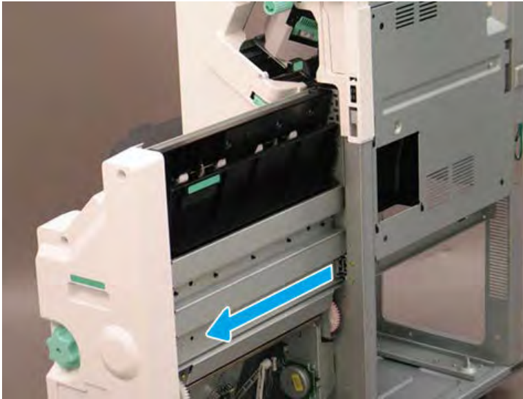
Figure 5-1932 Extend the right rail
