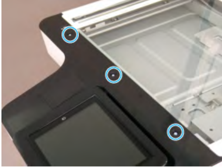
Figure 2-125 Remove the document feeder bezel
