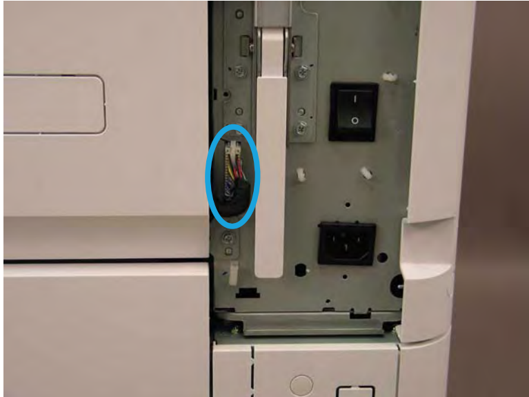
Figure 2-60 Disconnect right door connector
