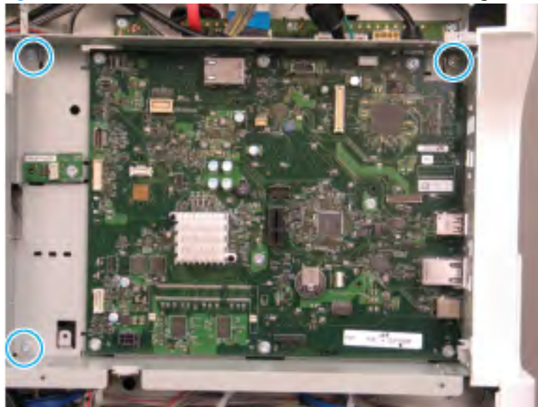
Figure 2-160 Remove three screws to remove the formatter cage
