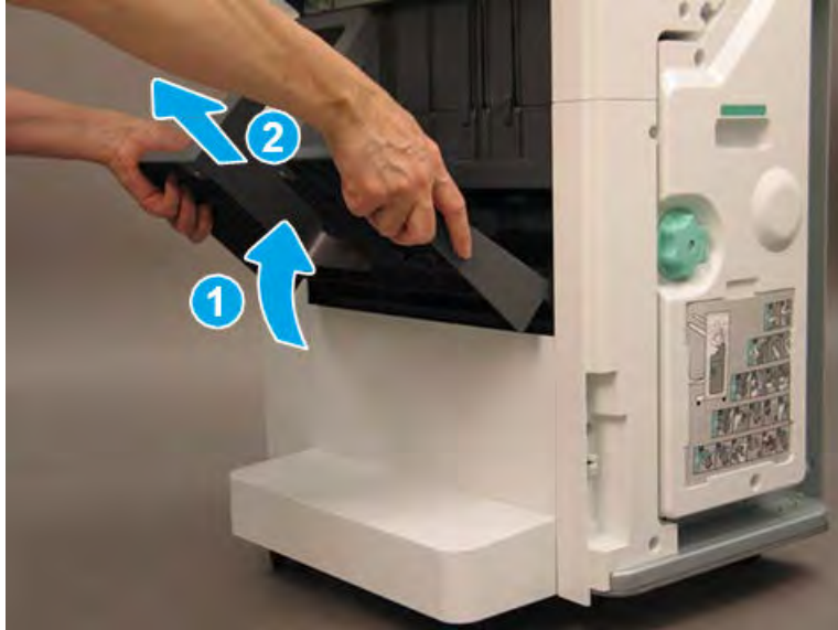
Figure 5-725 Remove the booklet output tray
