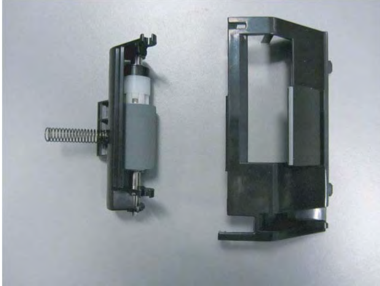
Figure 2-403 Document feeder separation roller cover and roller assembly
