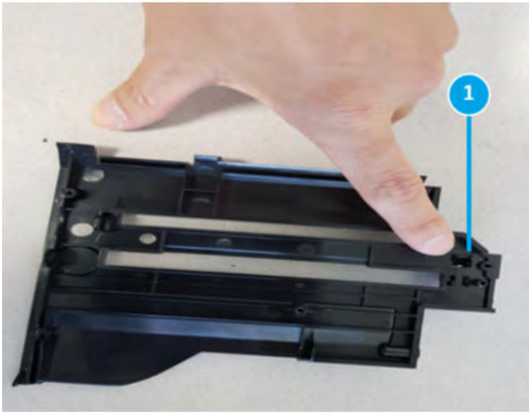
Figure 5-757 Remove rear tamper home sensor
