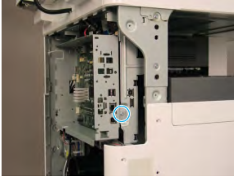
Figure 2-97 Remove the formatter cage side screw
