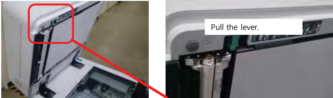
Figure 1-68 Flow document feeder dual sensor cleaning method (2 of 2)
