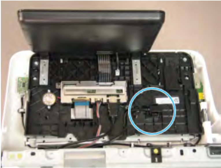
Figure 2-127 Remove the USB interconnect cable
