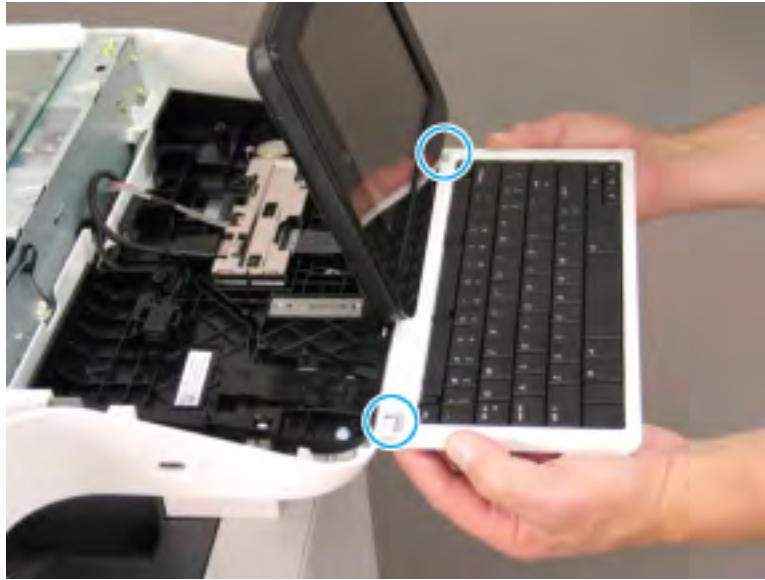
Figure 2-130 Remove the control-panel keyboard
