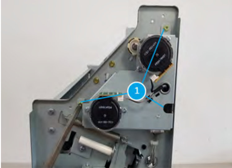
Figure 5-1544 Remove three screws
