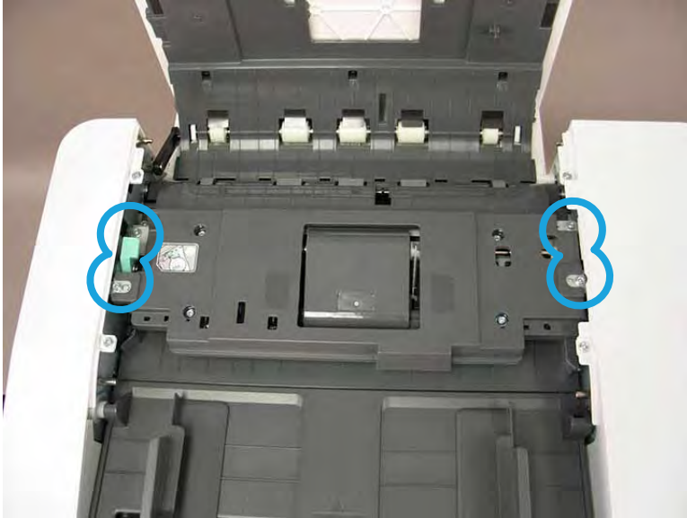
Figure 2-367 Remove four screws
