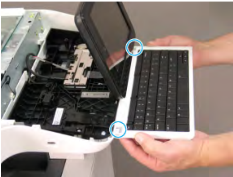
Figure 2-42 Remove the keyboard
