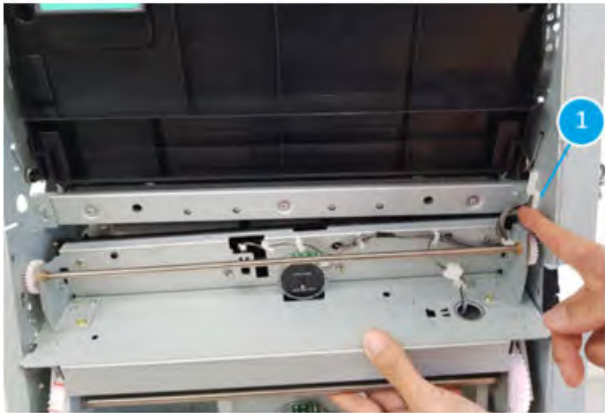
Figure 5-1659 Disconnect one connector
