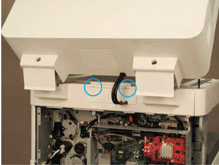
Figure 2-27 Remove document feeder connector cover
