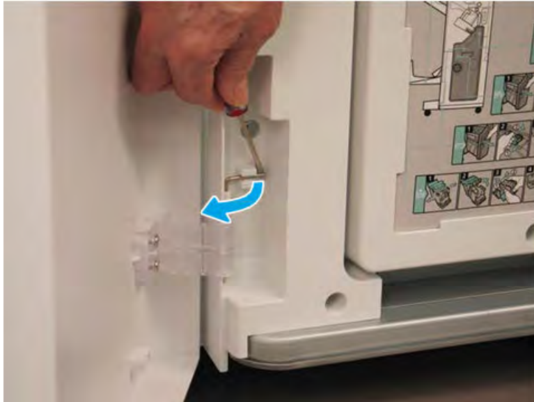
Figure 5-1081 Release the lower hinge pin
