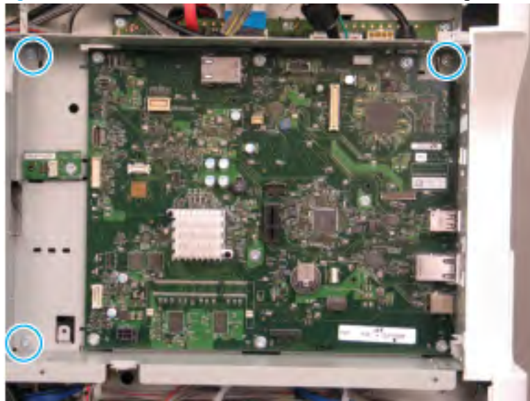
Figure 2-89 Remove three screws to remove the formatter cage
