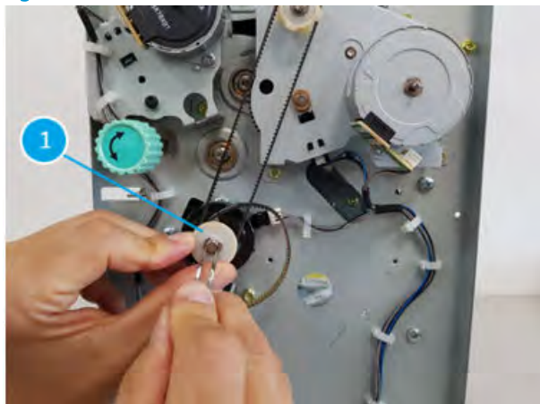
Figure 5-1486 Remove white washer
