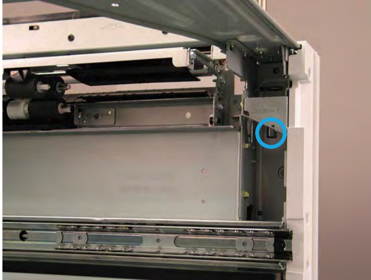
Figure 2-575 Release one tab
