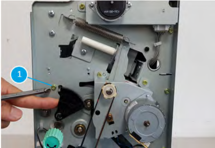
Figure 5-1800 Remove one screw at the front of the booklet maker
