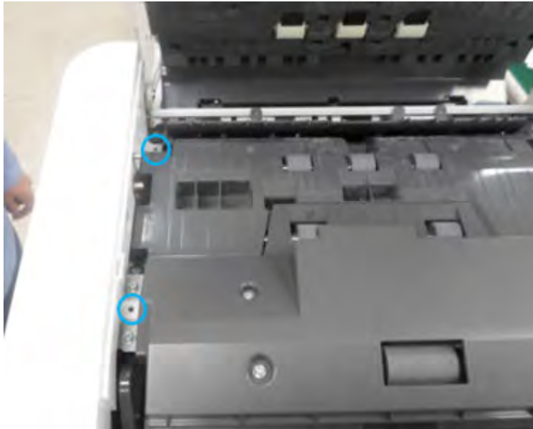
Figure 2-354 Remove the document feeder front cover top screws
