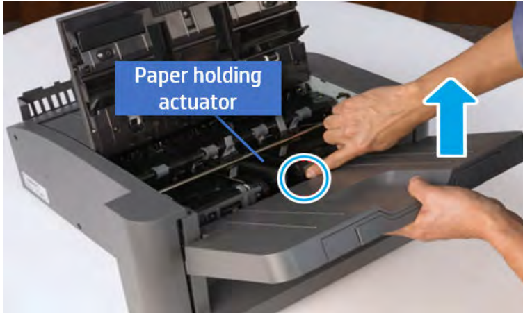
Figure 6-407 Remove the output tray.
