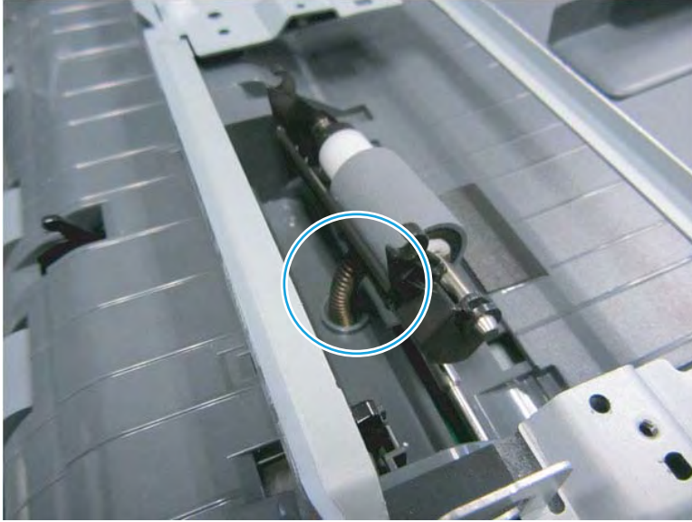
Figure 2-405 Separation roller assembly spring
