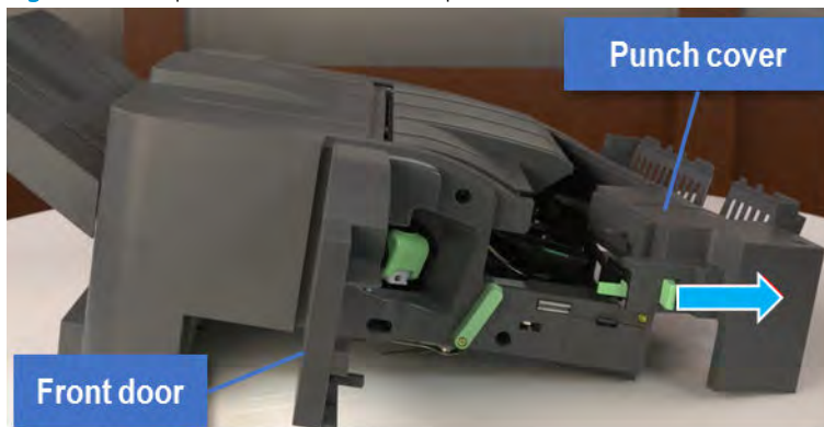
Figure 6-91 Open the front door and punch cover
