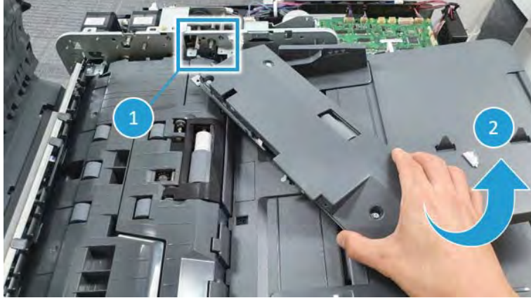
Figure 2-427 Remove the pickup roller assembly
