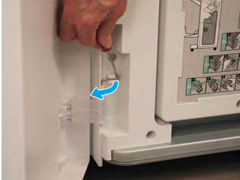
Figure 5-870 Release the lower hinge pin
