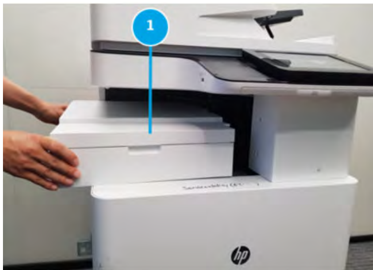
Figure 5-151 Pull out the bridge unit
