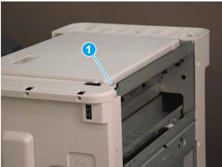
Figure 5-540 Remove one screw
