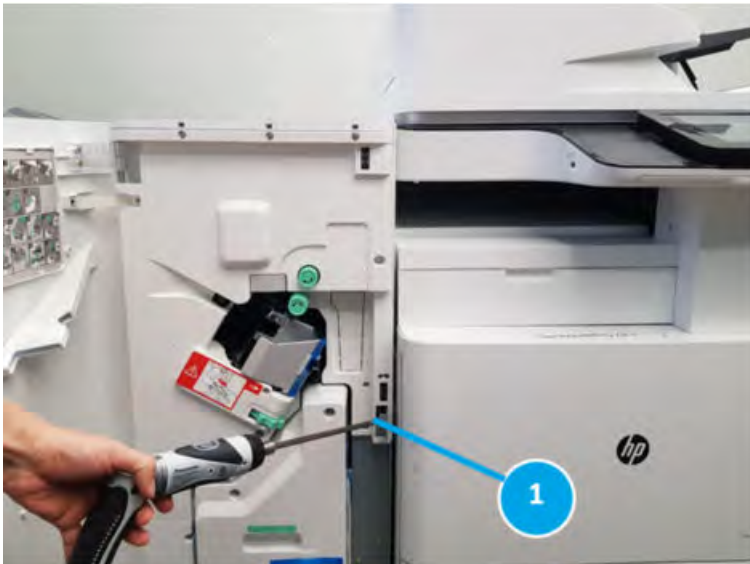
Figure 5-149 Pull the locker out
