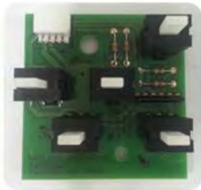
Figure 1-88 Paper size sensor PCA
