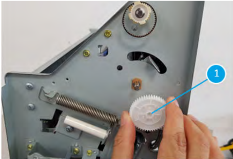
Figure 5-1546 Remove one e-clip on top of the white gear then remove the white gear
