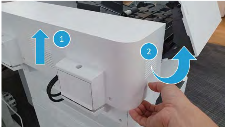
Figure 2-408 Release the top back cover.
