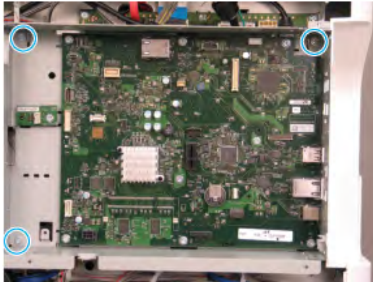
Figure 2-98 Remove three screws to remove the formatter cage
