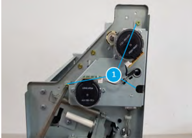
Figure 5-1554 Remove the booklet presser motor
