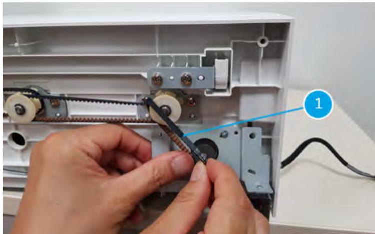
Figure 5-139 Remove the belt
