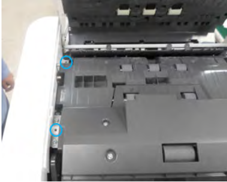
Figure 2-432 Remove the document feeder front cover top screws
