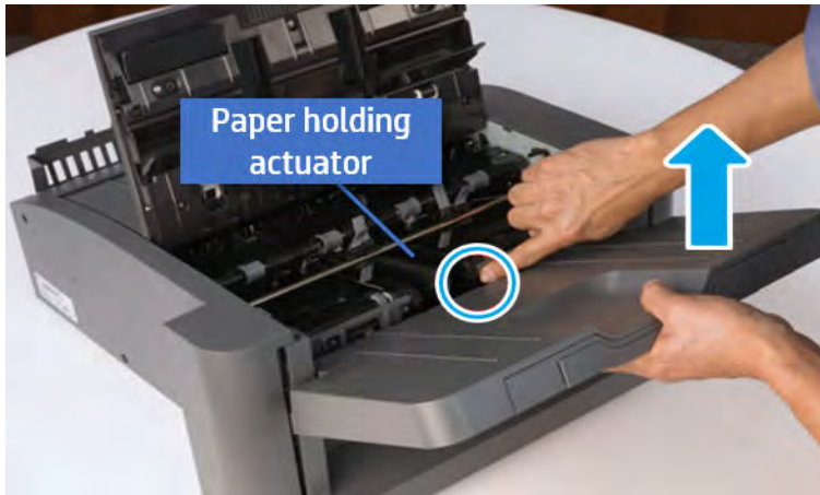
Figure 6-435 Remove the output tray.
