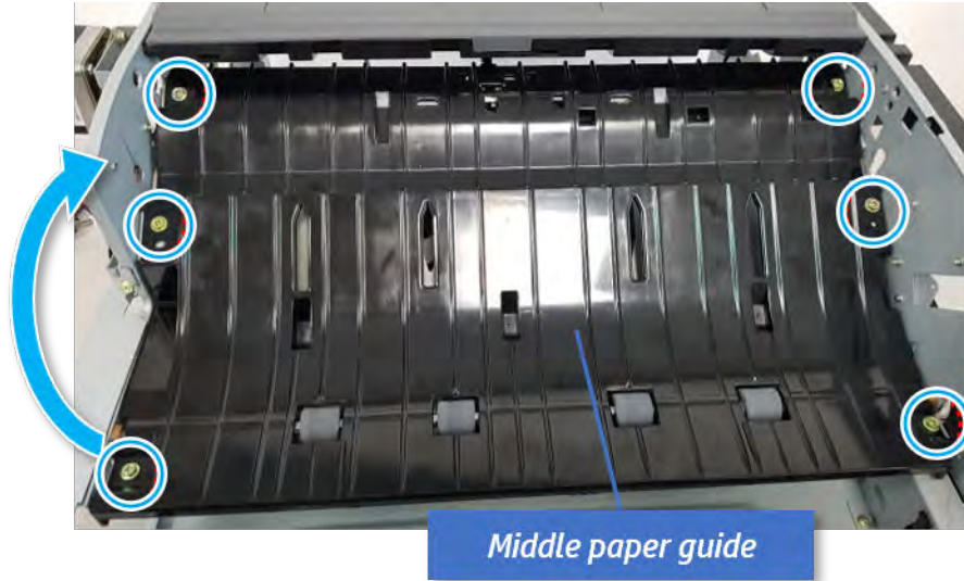
Figure 6-126 Open the middle paper guide
