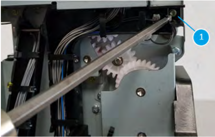
Figure 5-1861 Remove one screw at the rear of the booklet maker
