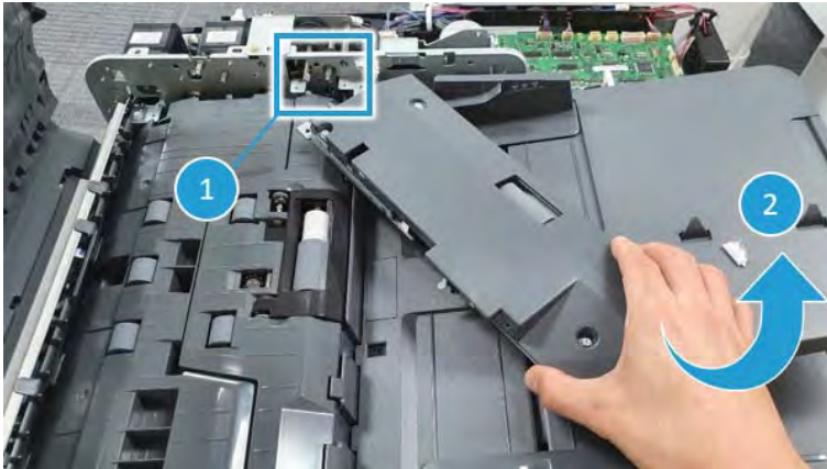
Figure 2-419 Remove the pickup roller assembly
