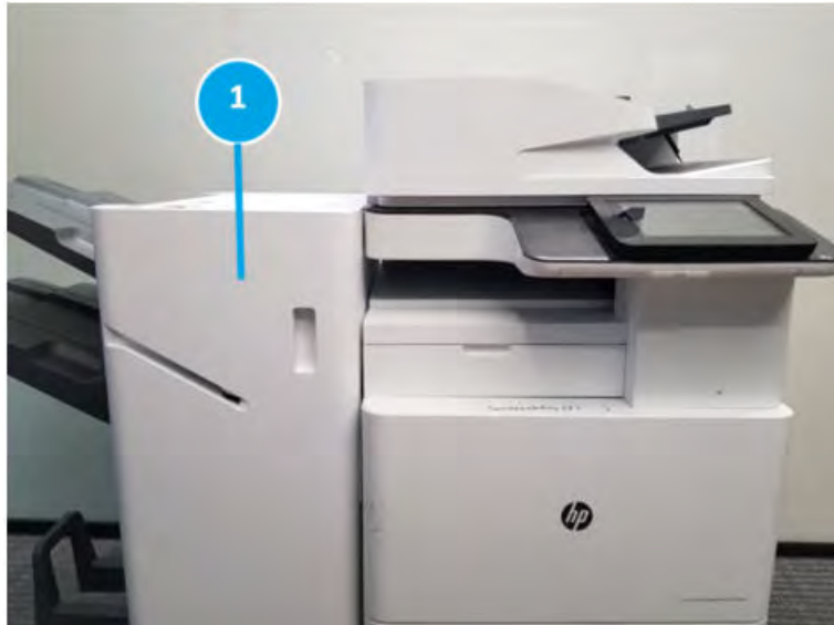
Figure 5-141 Open the front door
