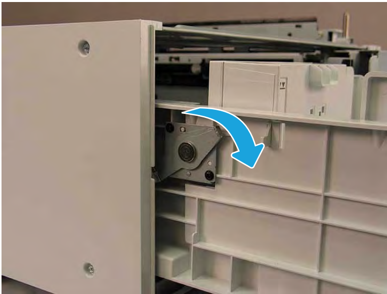
Figure 2-636 Release the tray left side hook lever
