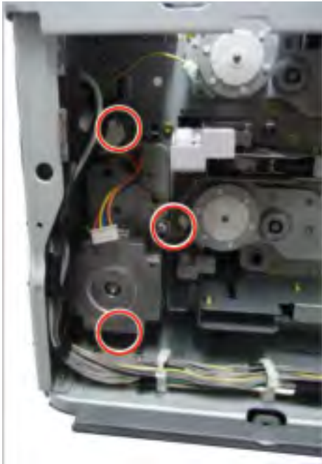
Figure 2-530 Remove the feed drive unit
