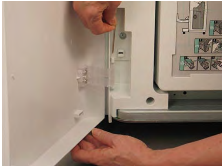
Figure 5-319 Remove the lower hinge pin
