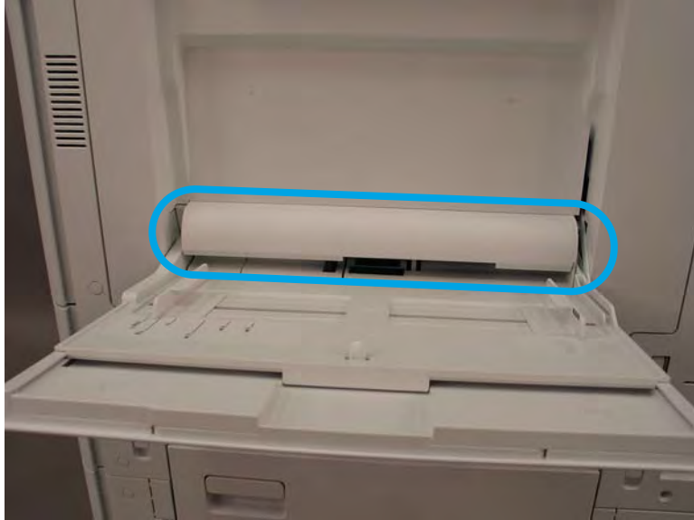
Figure 2-317 Remove the cover
