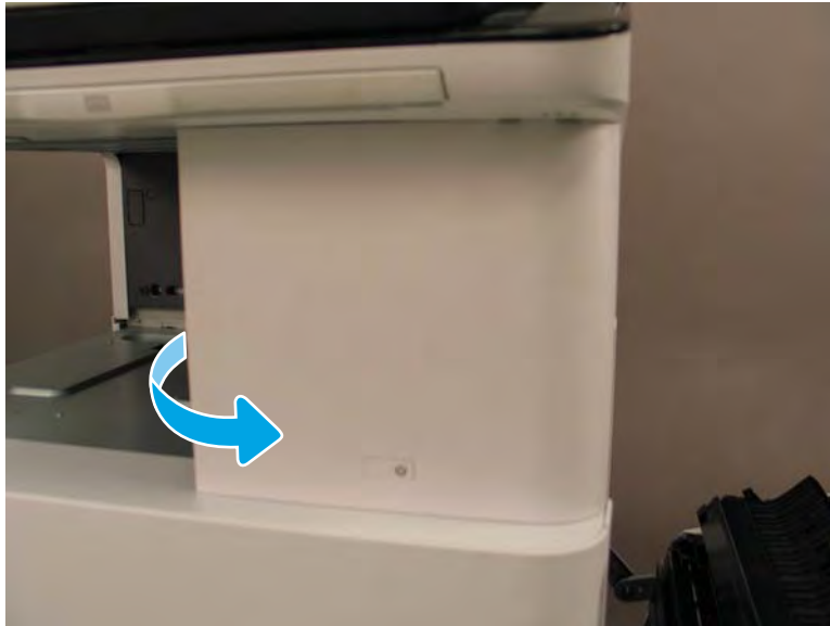
Figure 2-115 Remove the front top cover
