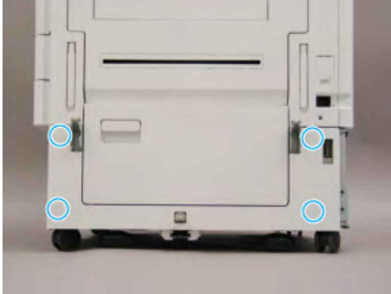
Figure 2-523 Remove the lower right cover
