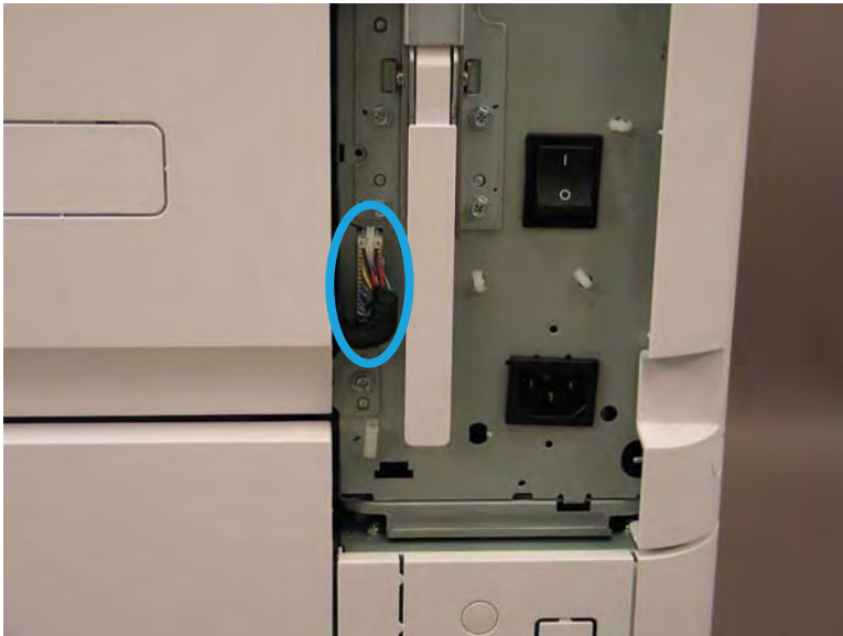
Figure 2-53 Disconnect right door connector
