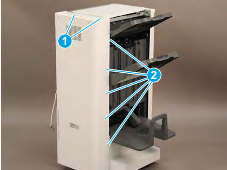
Figure 5-1087 Remove seven screws
