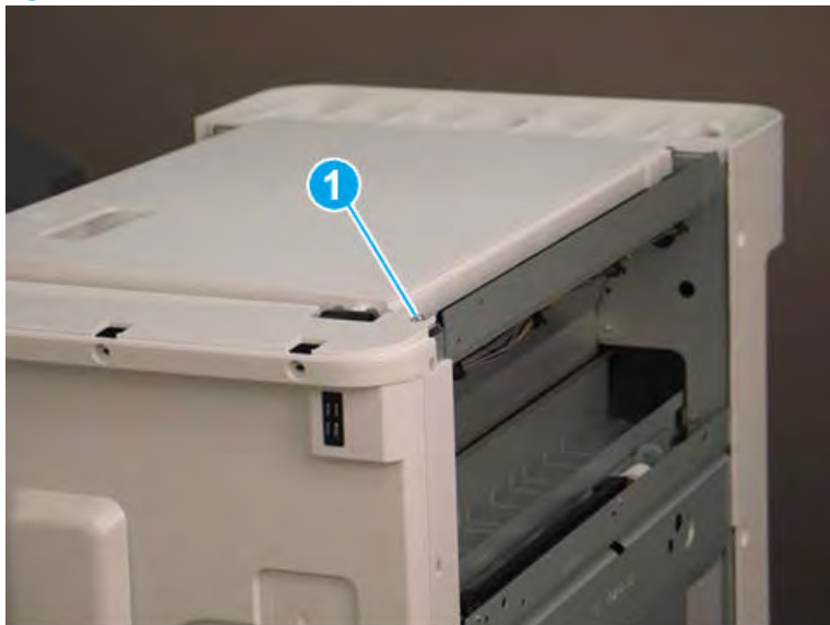
Figure 5-214 Remove one screw
