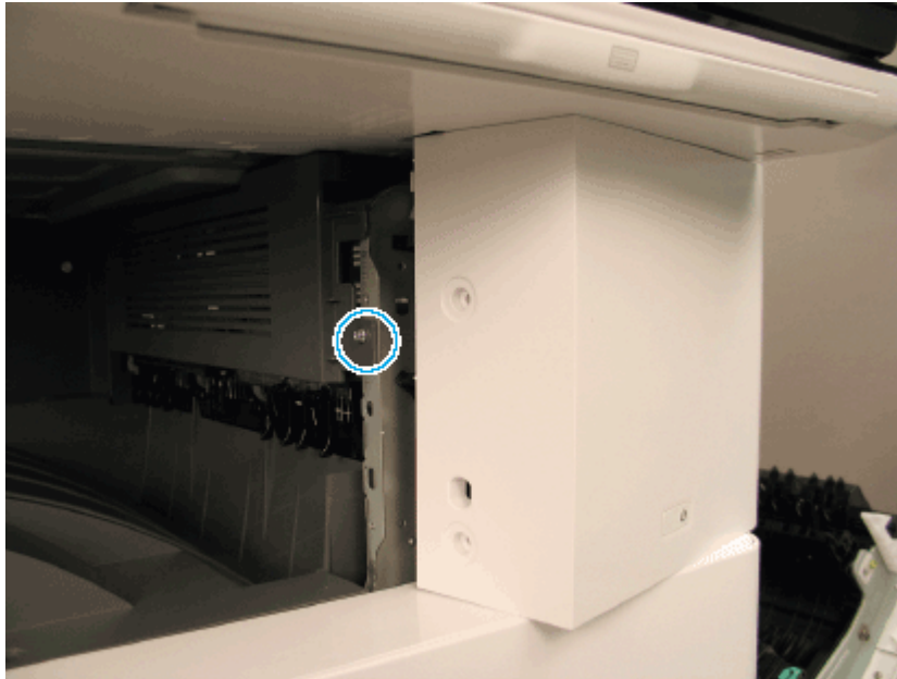
Figure 2-122 Remove the cover exit right
