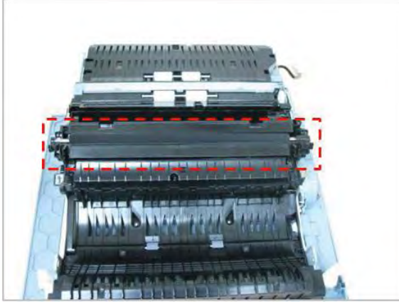
Figure 2-209 Remove transfer roller assembly
