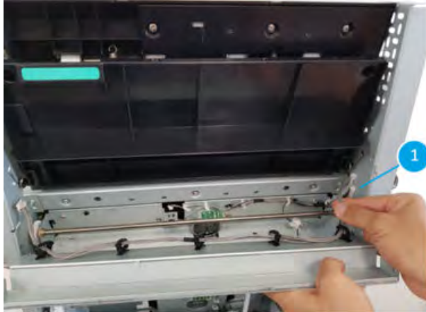
Figure 5-1726 Disconnect one connector
