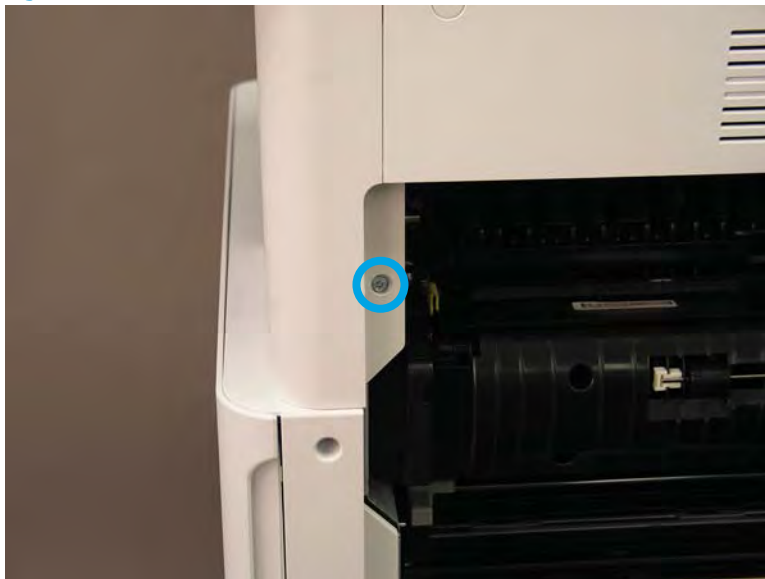
Figure 2-292 Remove one screw
