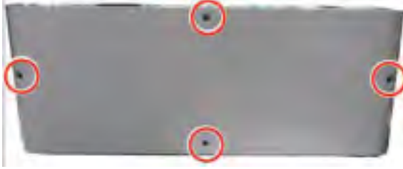
Figure 2-526 Remove the DCF rear cover
