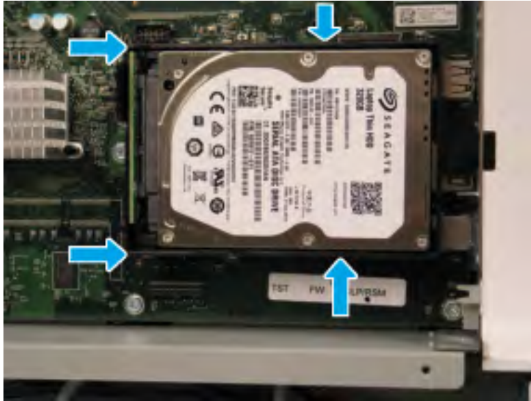
Figure 2-84 Remove the hard-disk drive (HDD)
