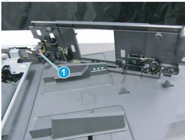
Figure 2-391 Turn the cover over and disconnect connector
