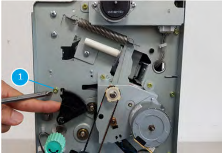
Figure 5-1893 Remove one screw at the front of the booklet maker
