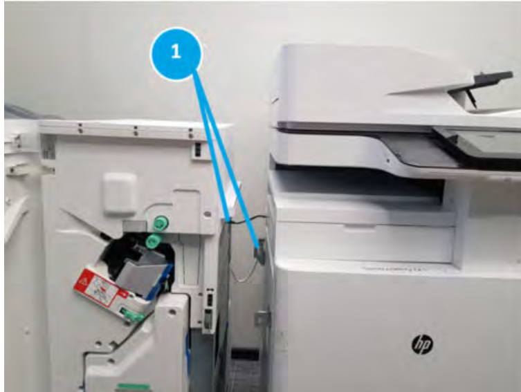
Figure 5-150 Separate the finisher from the printer and disconnect the two connectors
