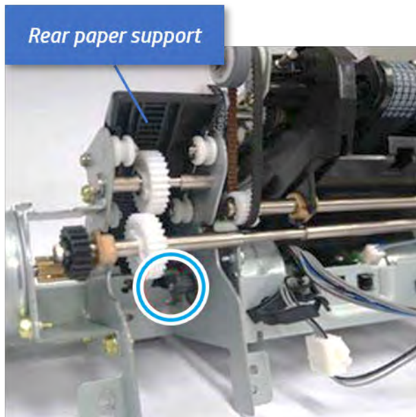
Figure 6-235 Remove the rear paper support
