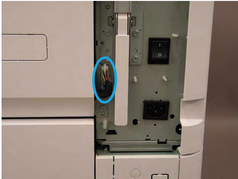
Figure 2-184 Disconnect right door connector
