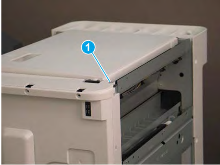
Figure 5-322 Remove one screw
