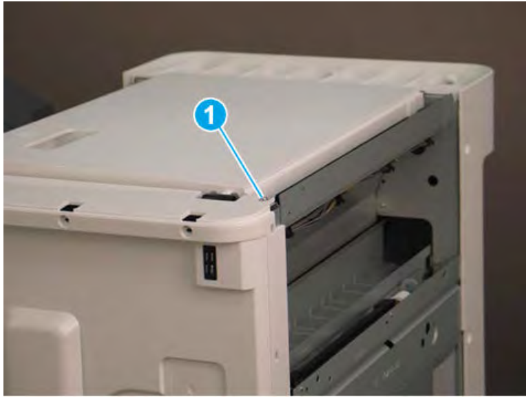
Figure 5-526 Remove one screw
