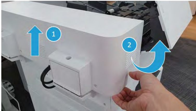
Figure 2-366 Release the top back cover.
