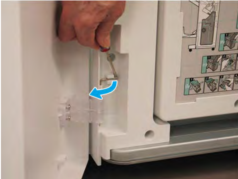
Figure 5-1314 Release the lower hinge pin
