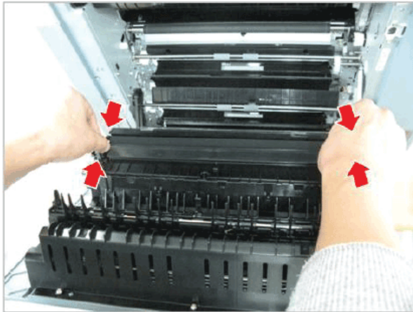
Figure 2-347 Remove HP LaserJet Transfer Roller (T2)
