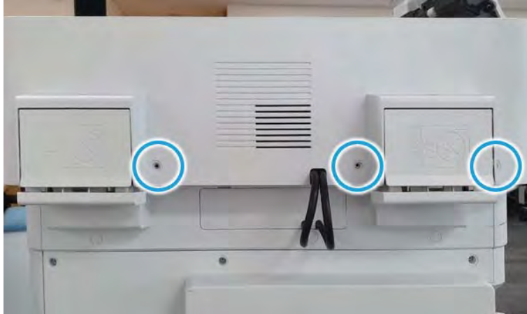
Figure 2-365 Remove 3 caps and 3 screws.
