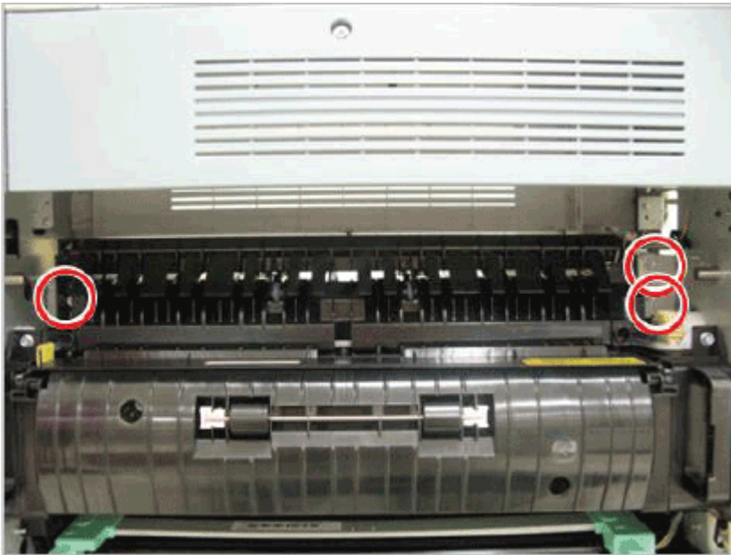
Figure 2-50 Remove screws and exit unit
