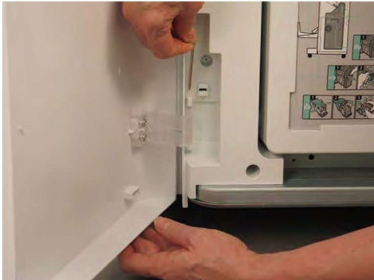
Figure 5-1389 Remove the lower hinge pin
