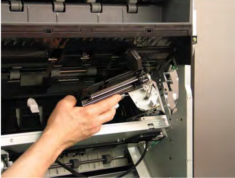
Figure 5-573 Remove the front tamper
