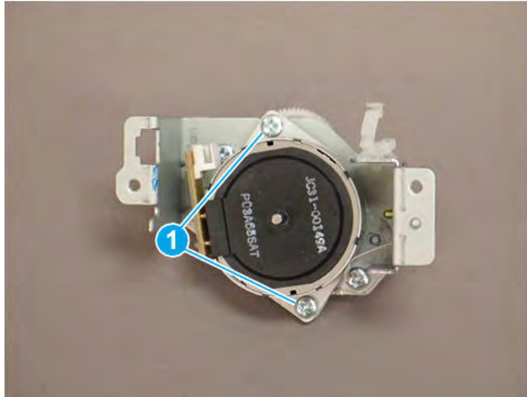
Figure 5-1406 Remove two screws and the motor
