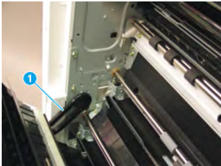
Figure 2-193 Release left dampener
