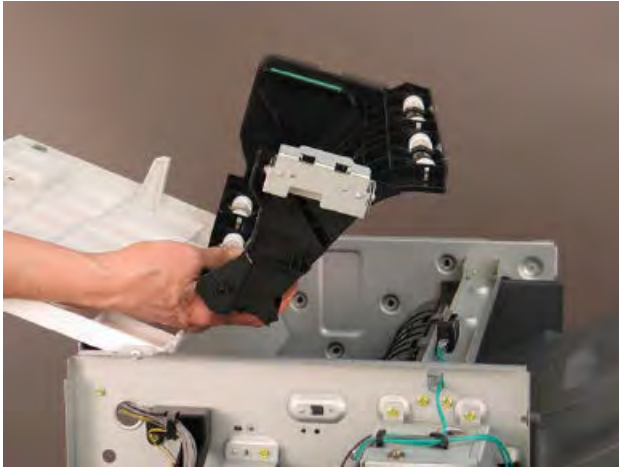
Figure 5-328 Remove the top jam access cover
