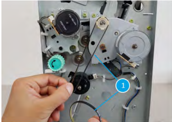
Figure 5-1487 Remove two belts
