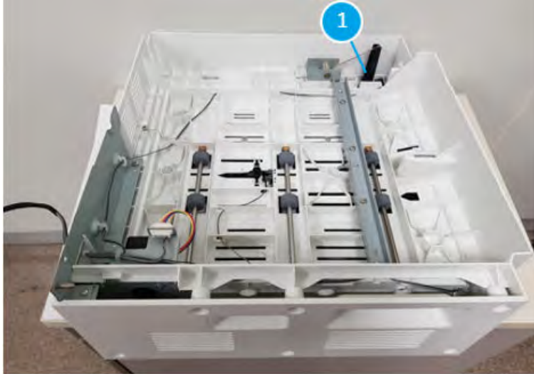
Figure 5-152 Location of the bridge door sensor
