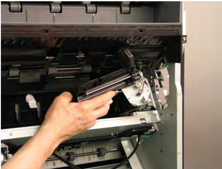
Figure 5-664 Remove the front tamper
