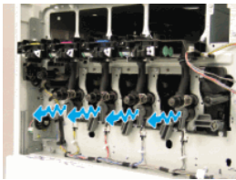
Figure 2-300 Release the toner supply pipes
