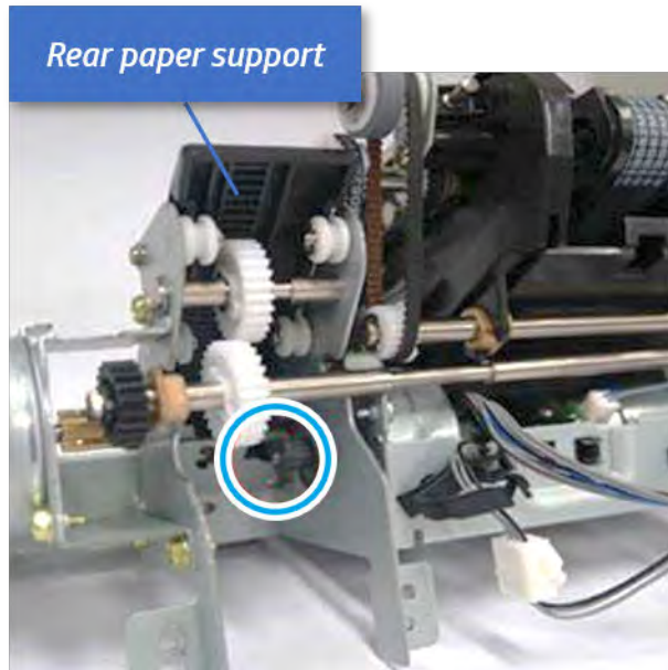
Figure 6-200 Remove the rear paper support
