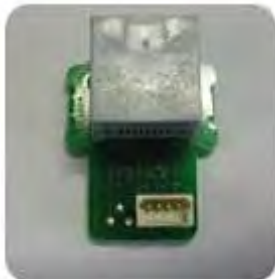
Figure 1-87 Toner CRUM joint PCA
