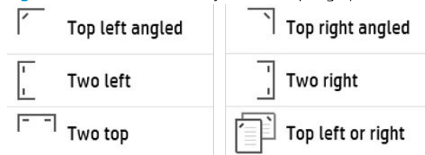
Figure 6-36 Inner finisher system - stapling options
