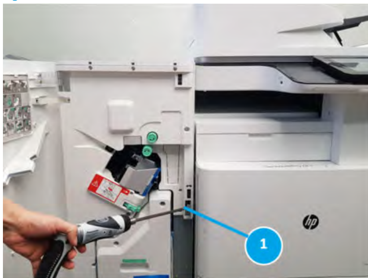
Figure 5-142 Pull the locker out
