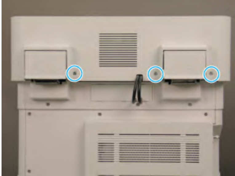
Figure 2-481 Remove the document feeder back cover bottom screws
