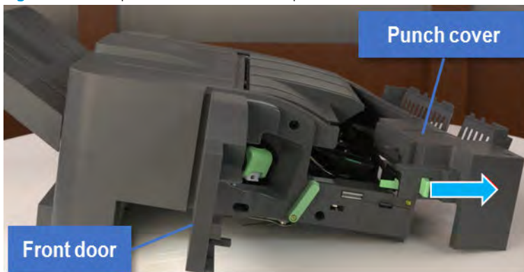
Figure 6-777 Open the front door and punch cover
