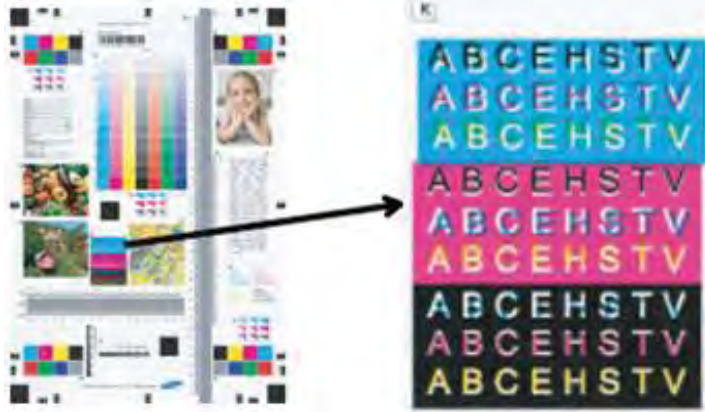
Figure 3-49 Typical faulty images
