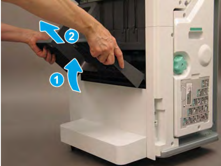
Figure 5-1043 Remove the booklet output tray
