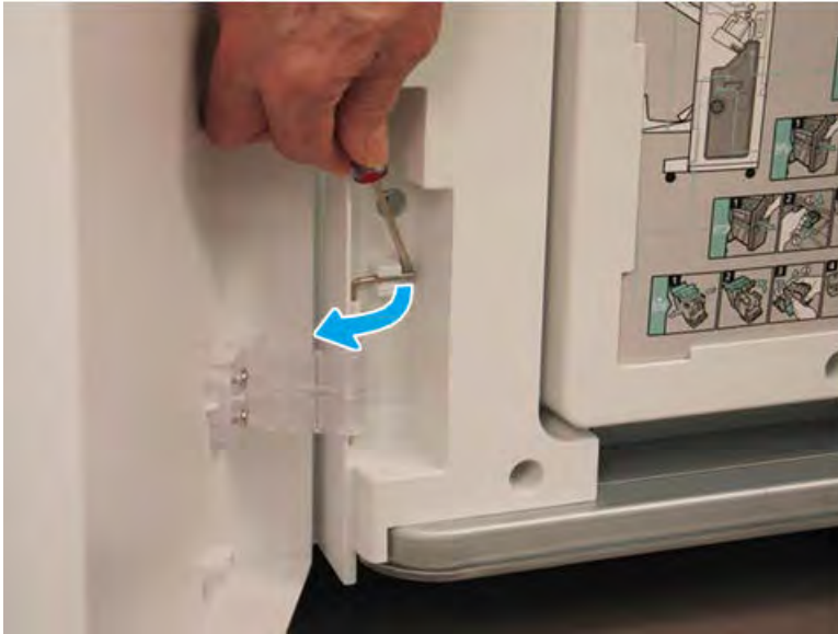
Figure 5-1035 Release the lower hinge pin
