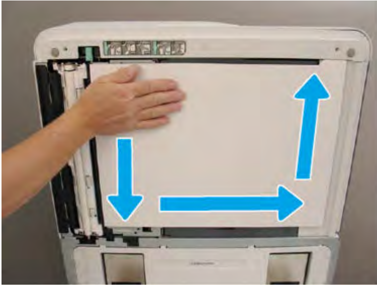
Figure 2-18 Smooth the white backing
