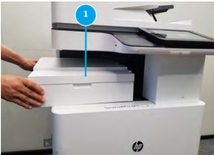
Figure 5-135 Pull out the bridge unit
