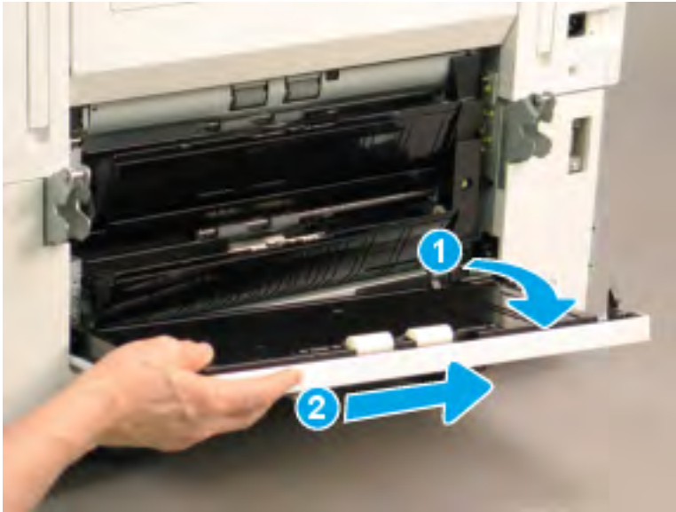
Figure 2-525 Remove the DCF right door
