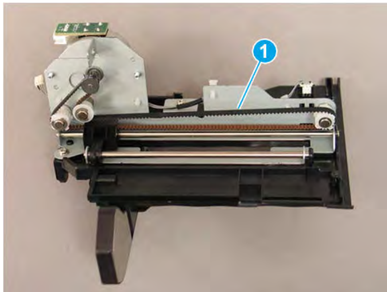
Figure 5-666 Release the belt and remove the motor
