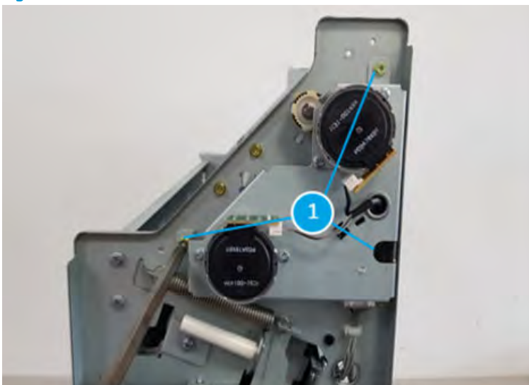
Figure 5-1550 Remove three screws
