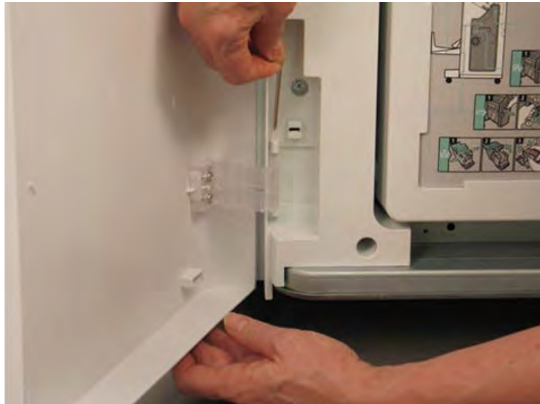
Figure 5-194 Remove the lower hinge pin
