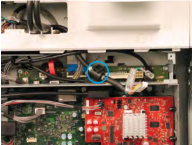
Figure 2-34 Remove the cable choke
