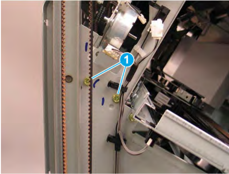
Figure 5-1115 Remove two screws
