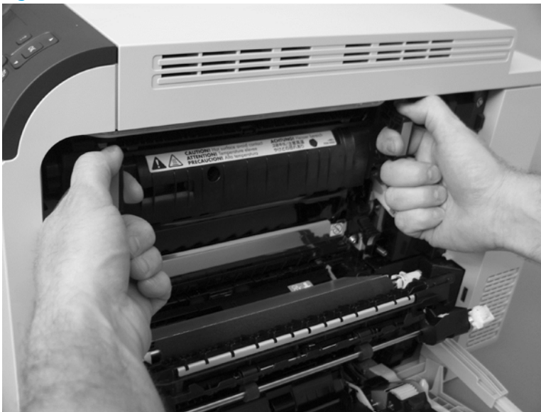
Figure 1-28 Remove the fuser (2 of 2)
