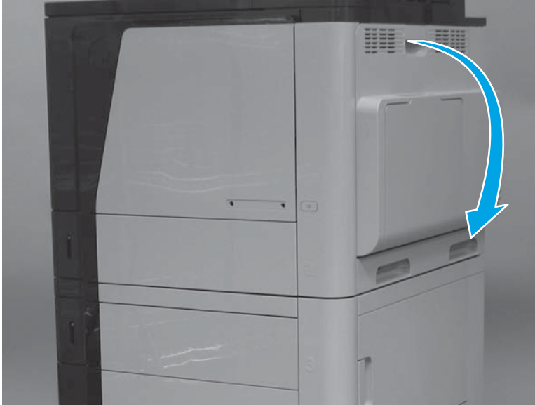
Figure 1-233 Remove the cassette feed guide (1 of 2)
