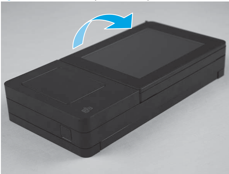
Figure 1-61 Reinstall the keyboard assembly (M680z; 4 of 7)
