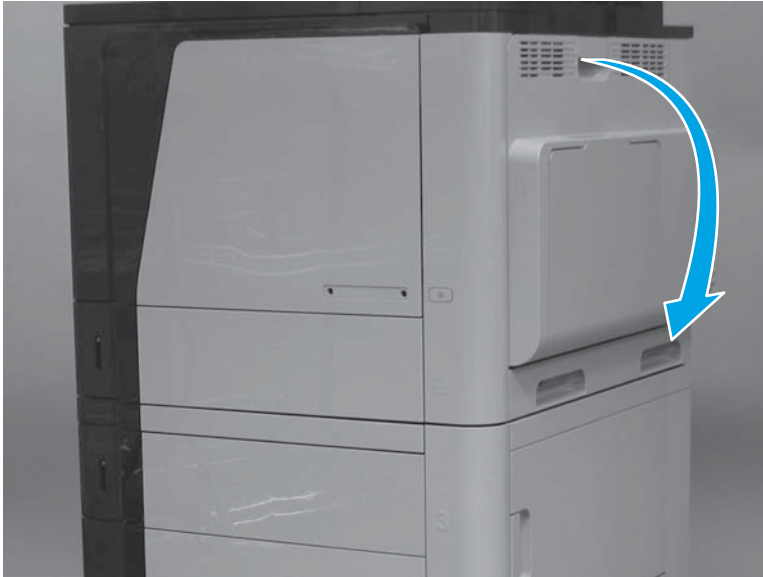
Figure 1-73 Remove the transfer roller (1 of 3)
