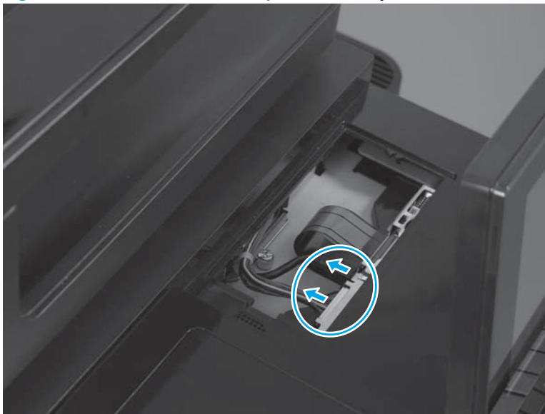
Figure 1-44 Remove the control-panel assembly (M680; 4 of 7)
