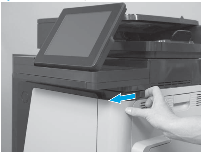
Figure 1-78 Remove the output bin bezel (1 of 2)
