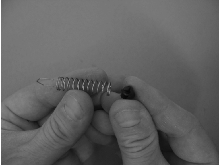
Figure 1-336 Reinstall the lifter base assembly (1 of 2)
