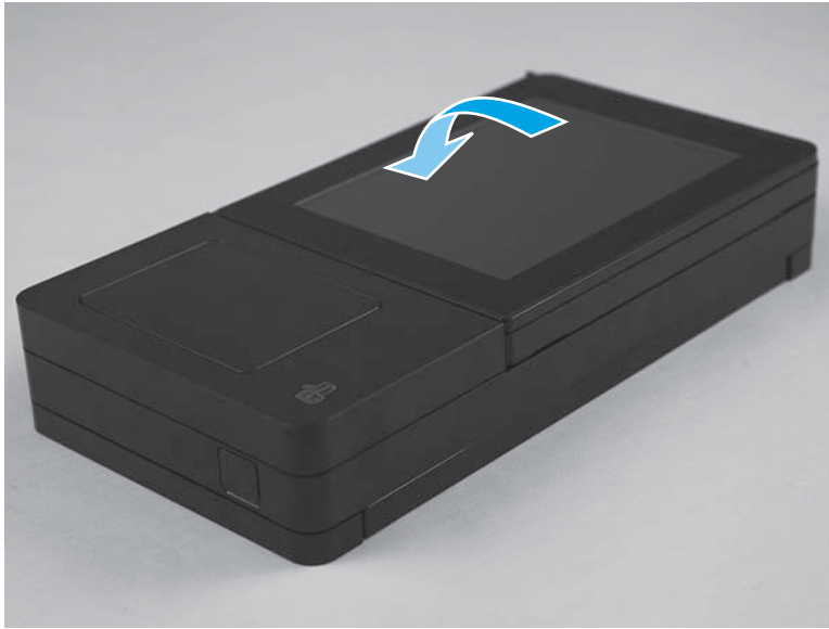
Figure 1-54 Remove the keyboard assembly (M680z; 4 of 7)
