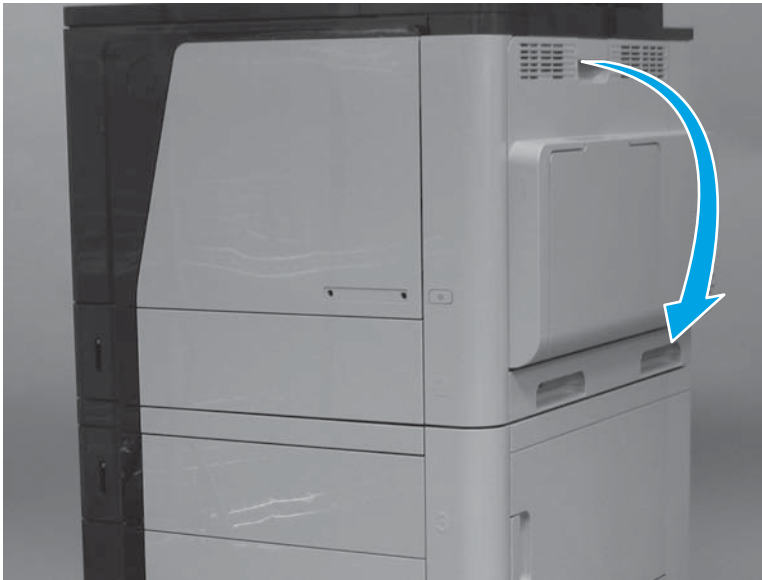
Figure 1-27 Remove the fuser (1 of 2)
