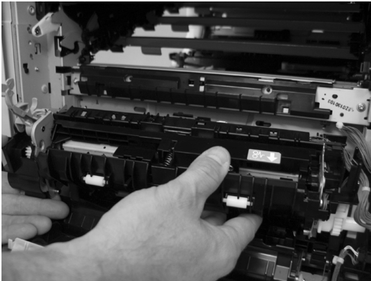
Figure 1-260 Remove the registration assembly (8 of 8)
