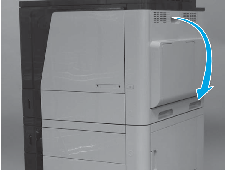
Figure 1-29 Remove the intermediate transfer belt (1 of 4)
