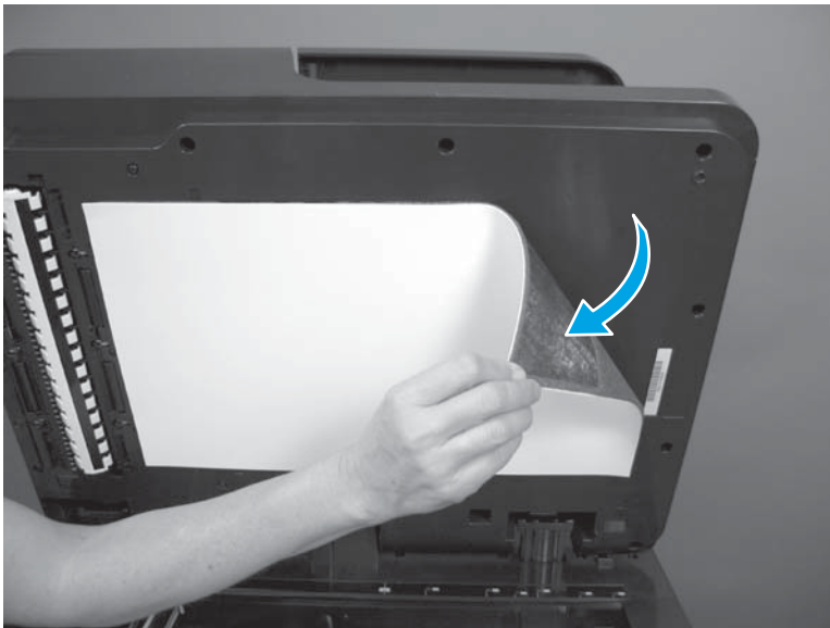
Figure 1-81 Remove the document feeder white backing (M680; 2 of 2)
