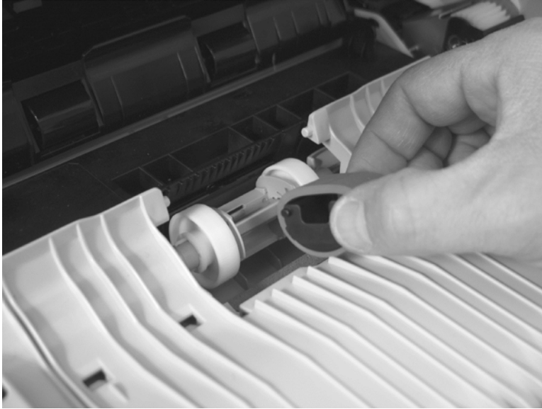
Figure 1-70 Remove the pickup roller (Tray 1; 5 of 5)
