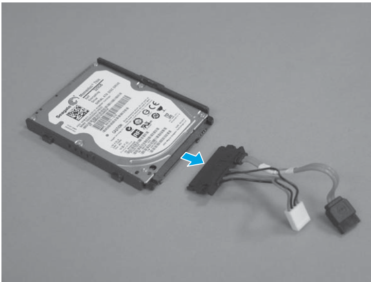
Figure 1-21 Remove the HDD (4 of 4)
