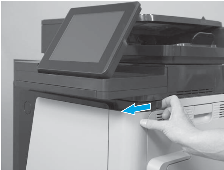
Figure 1-177 Remove the scissor hinge assemblies (1 of 4)
