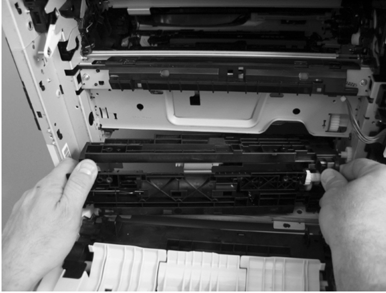
Figure 1-351 Remove the paper-pickup assembly (11 of 11)
