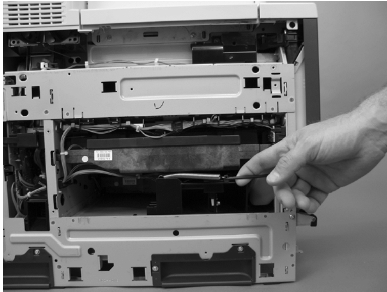
Figure 1-271 Remove the cartridge fan and environmental sensor (2 of 7)
