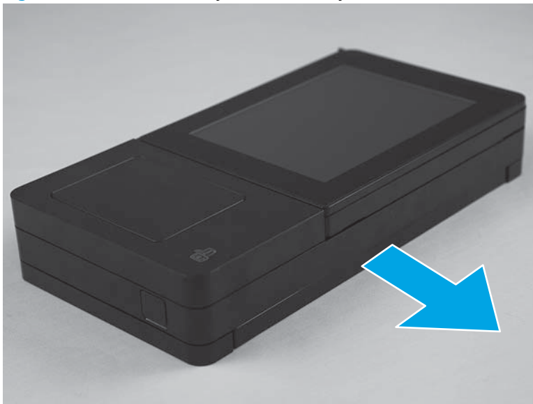
Figure 1-55 Remove the keyboard assembly (M680z; 5 of 7)
