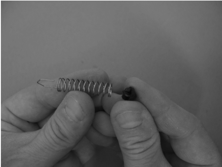
Figure 1-411 Reinstall the lifter base assembly (1x500-sheet paper feeder)
