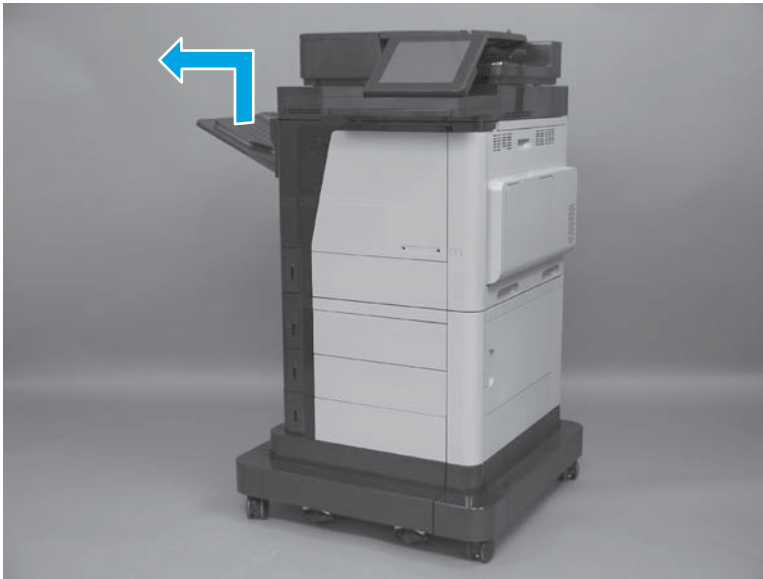
Figure 1-77 Remove the standard output bin
