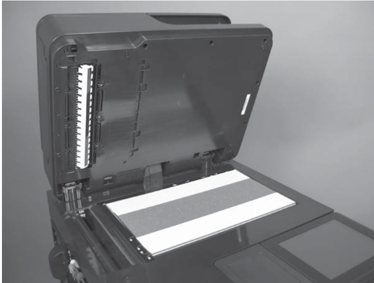
Figure 1-82 Install a replacement document feeder white backing (1 of 9)
