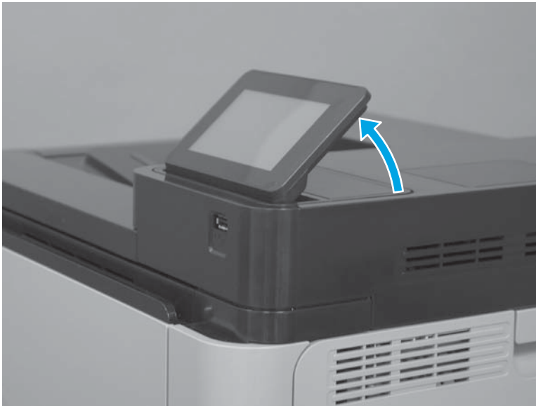
Figure 1-33 Remove the control panel (M651; 1 of 8)
