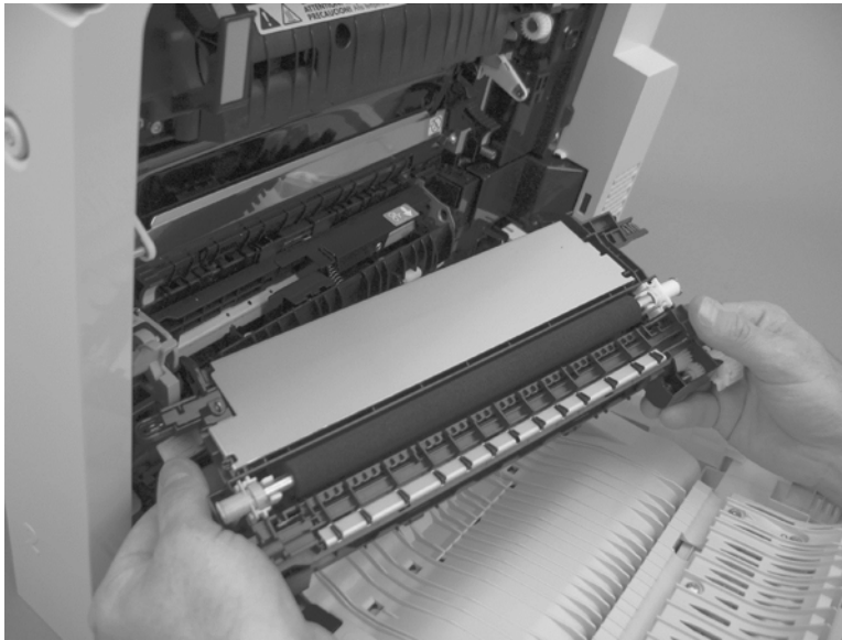
Figure 1-238 Remove the secondary transfer assembly (3 of 3)
