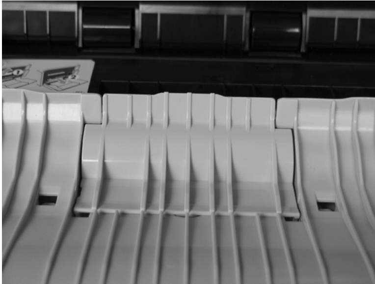
Figure 1-72 Incorrect position of cover
