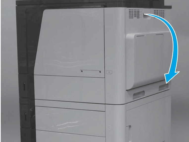
Figure 1-236 Remove the secondary transfer assembly (1 of 3)
