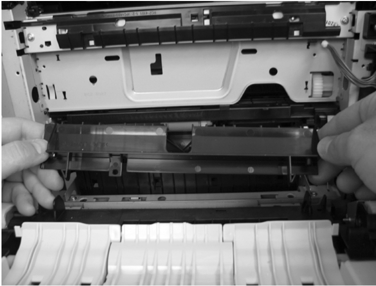
Figure 1-347 Remove the paper-pickup assembly (7 of 11)
