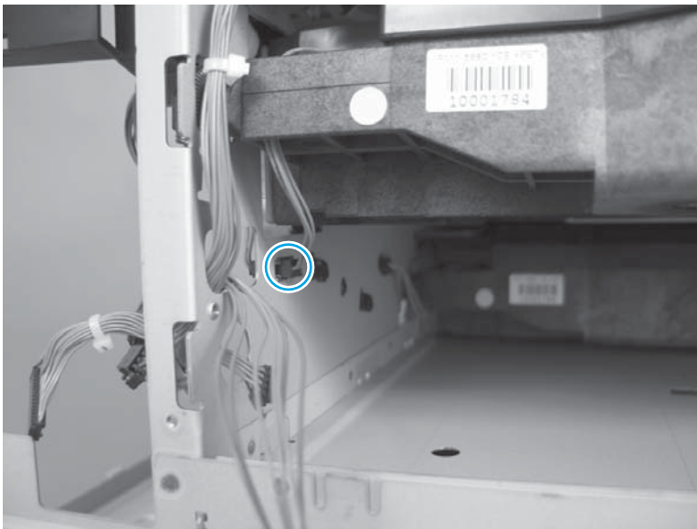
Figure 1-353 Remove the laser/scanner assembly (Y/M; 2 of 5)
