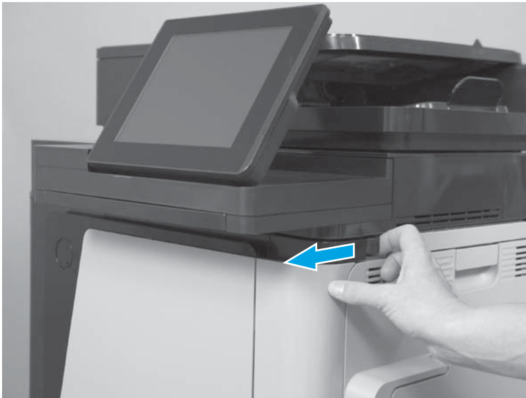
Figure 1-149 Remove the SCB (7 of 13)
