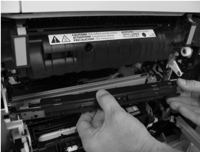
Figure 1-252 Remove the RD sensor assembly (7 of 7)
