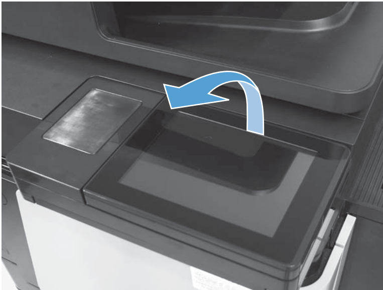
Figure 1-41 Remove the control-panel assembly (M680; 1 of 7)
