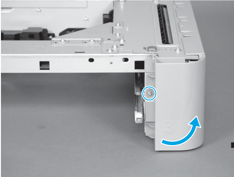
Figure 1-401 Remove the right-front cover (1x500-sheet paper feeder)
