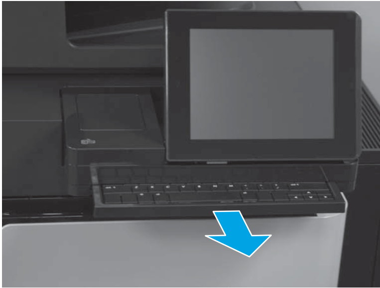
Figure 1-43 Remove the control-panel assembly (M680; 3 of 7)
