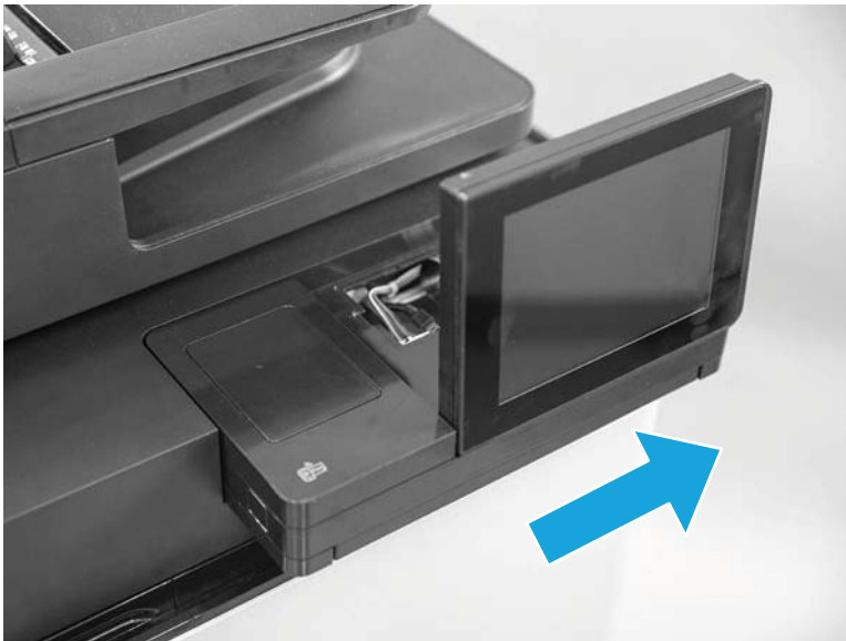
Figure 1-46 Remove the control-panel assembly (M680; 6 of 7)
