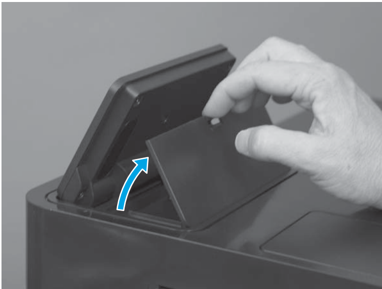
Figure 1-34 Remove the control panel (M651; 2 of 8)
