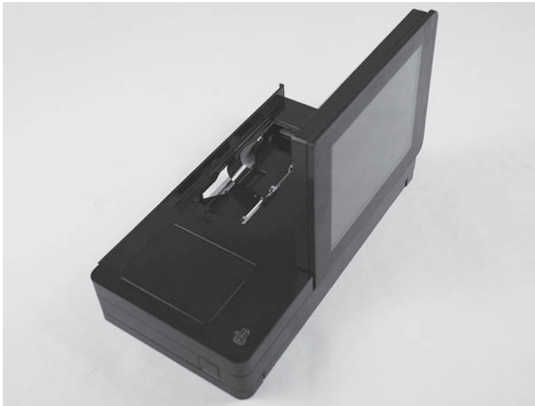
Figure 1-51 Remove the keyboard assembly (M680z; 1 of 7)
