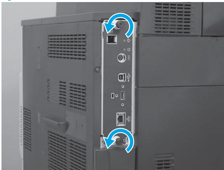
Figure 1-9 Remove the formatter
