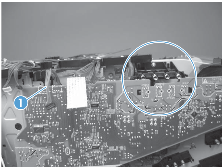
Figure 1-369 Reinstall the high-voltage power supply upper
