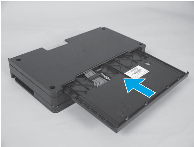
Figure 1-59 Reinstall the keyboard assembly (M680z; 2 of 7)
