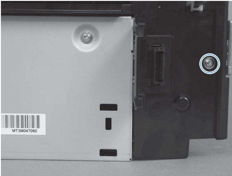
Figure 1-472 Remove the holder connector (stapling mailbox)
