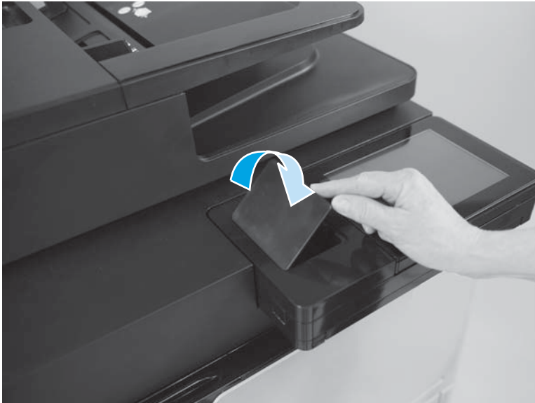
Figure 1-134 Reinstall the HIP cover (M880; 2 of 2)
