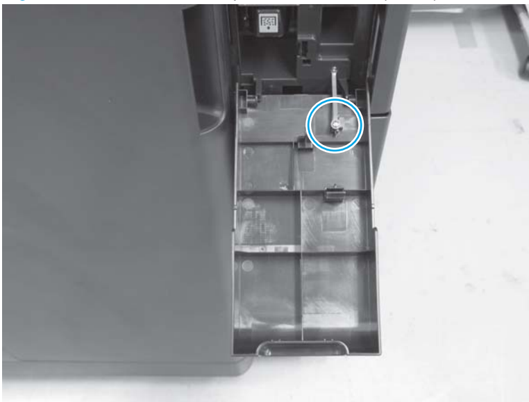
Figure 1-1025 Remove the punch front cover (1 of 2)
