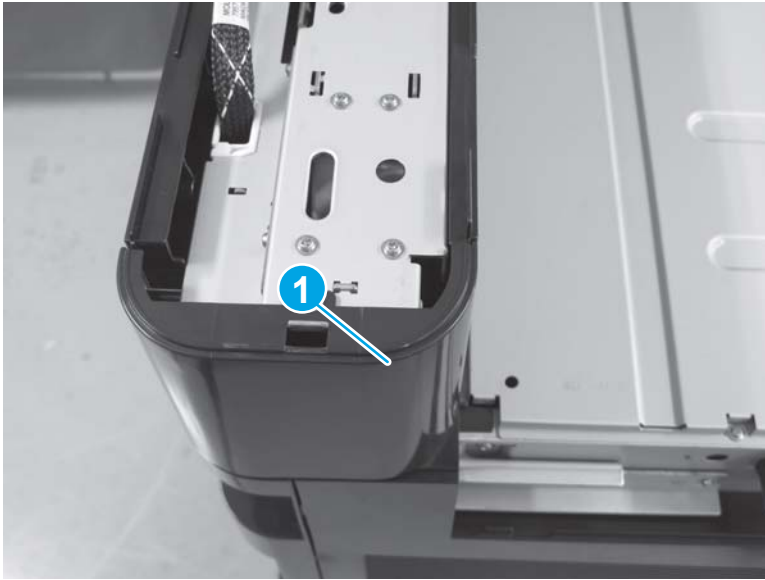
Figure 1-155 Remove the left upper rear cover and rear upper B cover (M880; 2 of 3)
