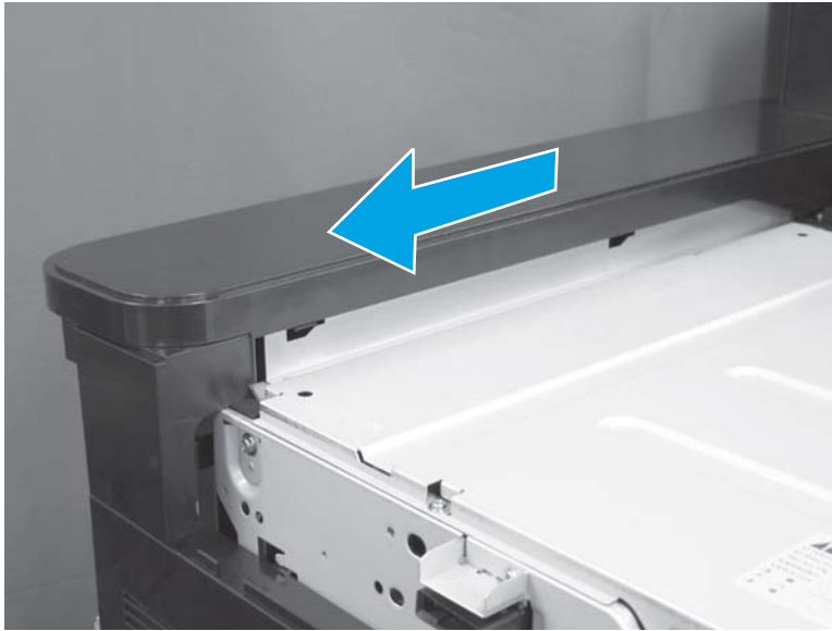
Figure 1-162 Remove the rear top cover (M855; 2 of 3)
