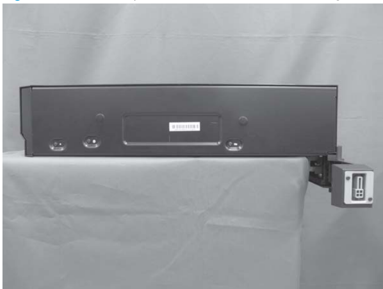
Figure 1-634 Incorrect placement of the IPTU for servicing
