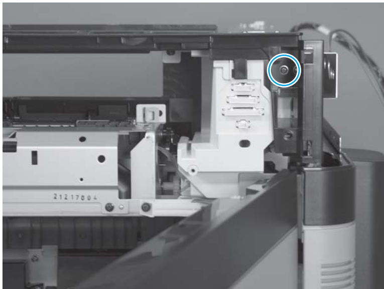
Figure 1-489 Remove the face-down delivery assembly (M880; 1 of 19)
