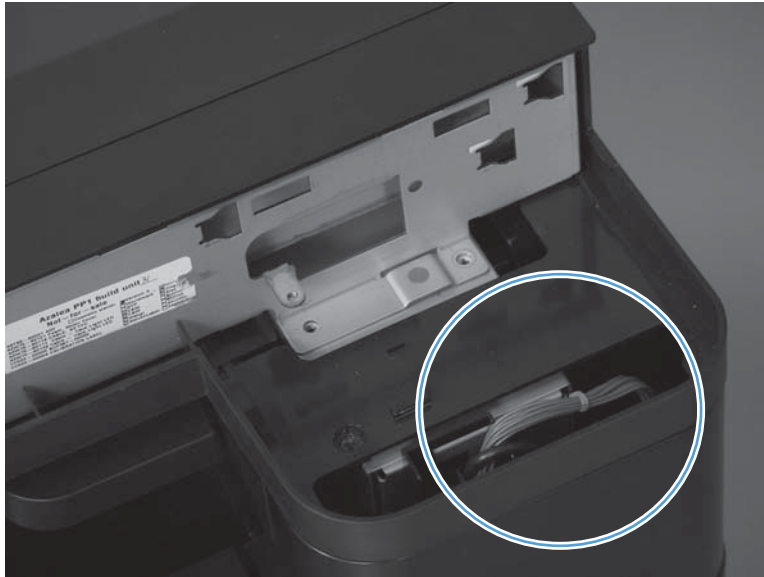
Figure 1-234 Remove the scanner assembly (M880; 6 of 7)
