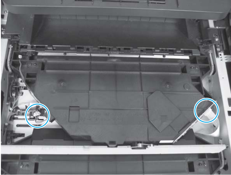
Figure 1-453 Remove the laser/scanner assembly (yellow and magenta; 2 of 6)
