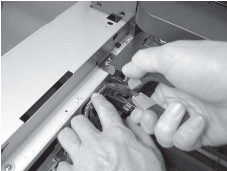
Figure 1-465 Remove the laser/scanner assembly (cyan and black; 6 of 8)
