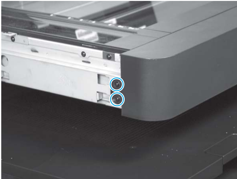
Figure 1-124 Remove the scanner front cover (M880; 5 of 8)
