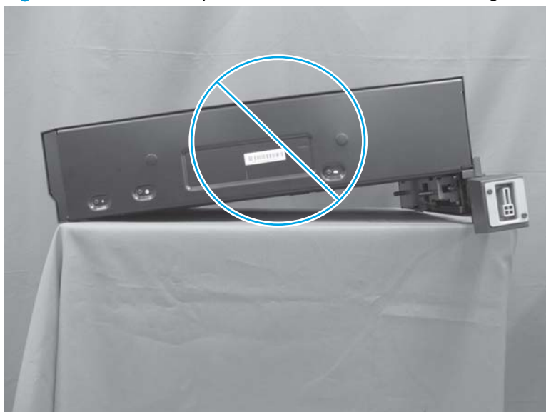
Figure 1-634 Incorrect placement of the IPTU for servicing
