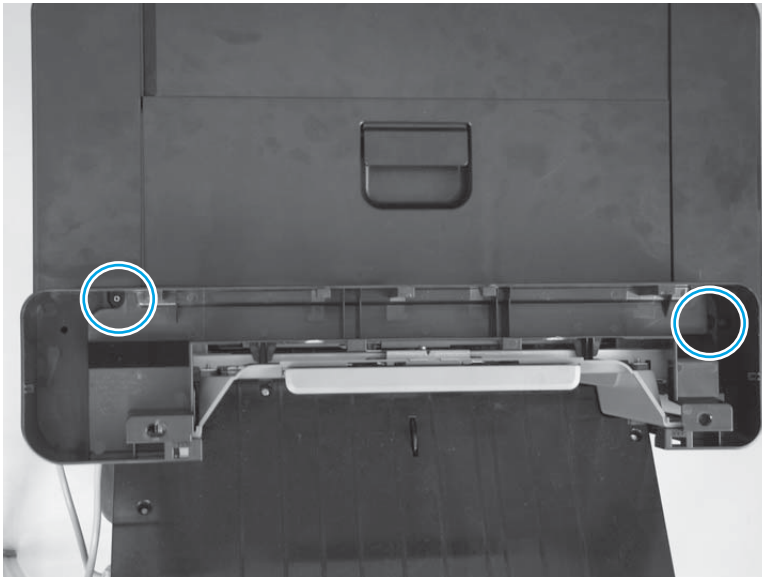
Figure 1-697 Remove the lower stepped cover assembly (1 of 5)
