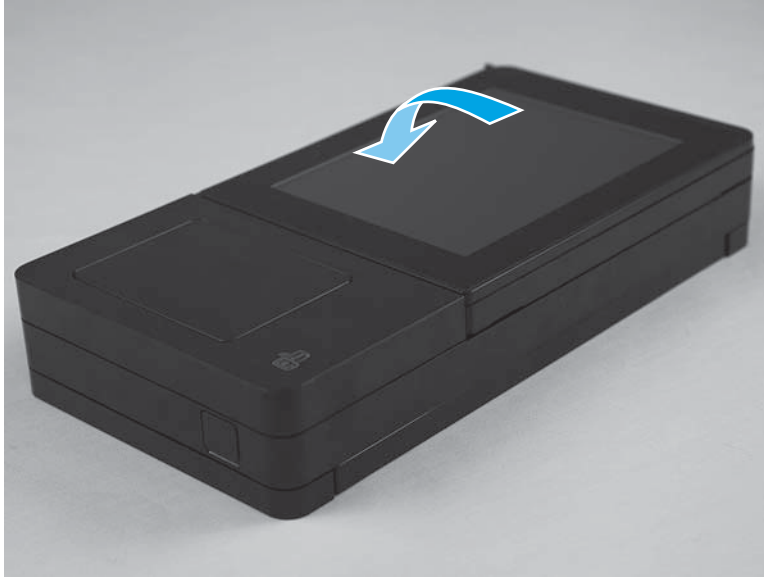
Figure 1-74 Remove the keyboard assembly (M880; 4 of 7)
