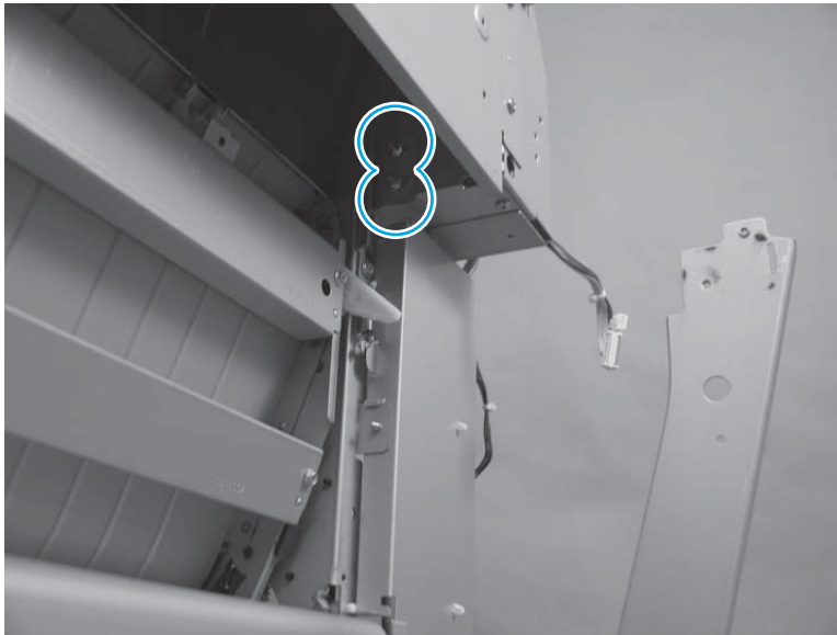
Figure 1-907 Remove the paper pass assembly (5 of 6)
