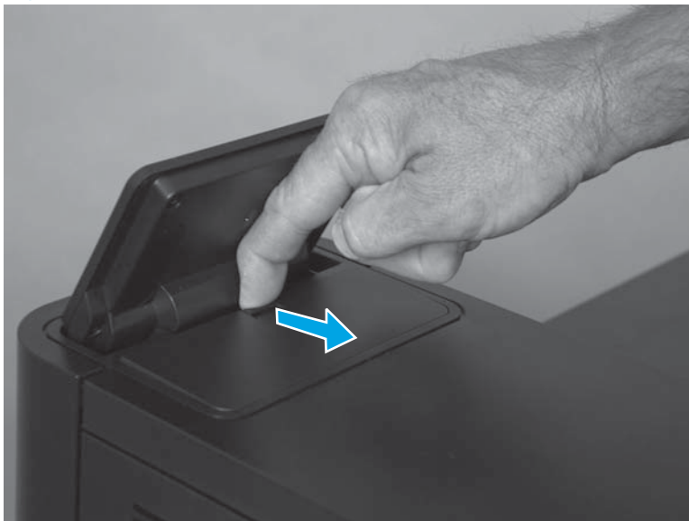
Figure 1-50 Remove the control panel assembly (M855; 2 of 10)
