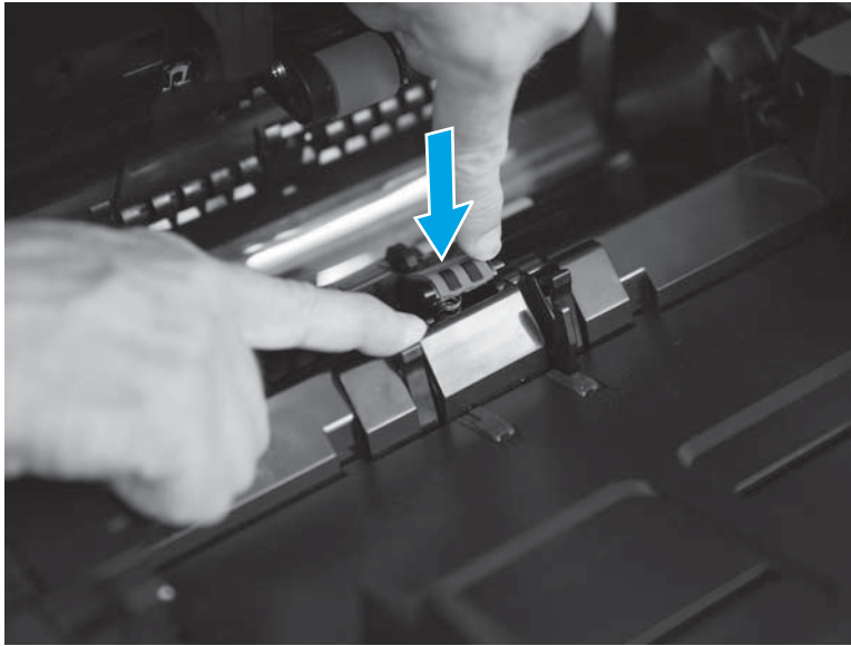
Figure 1-95 Reinstall the document-feeder separation pad (M880; 3 of 5)
