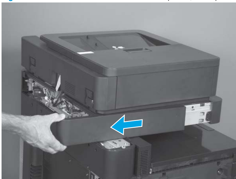
Figure 1-117 Remove the scanner left cover (M880; 2 of 2)
