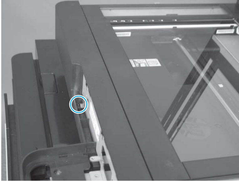
Figure 1-123 Remove the scanner front cover (M880; 4 of 8)
