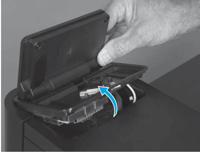
Figure 1-53 Remove the control panel assembly (M855; 5 of 10)
