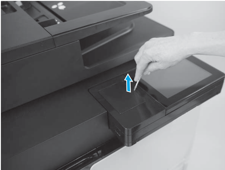
Figure 1-131 Remove the HIP cover (M880; 2 of 3)
