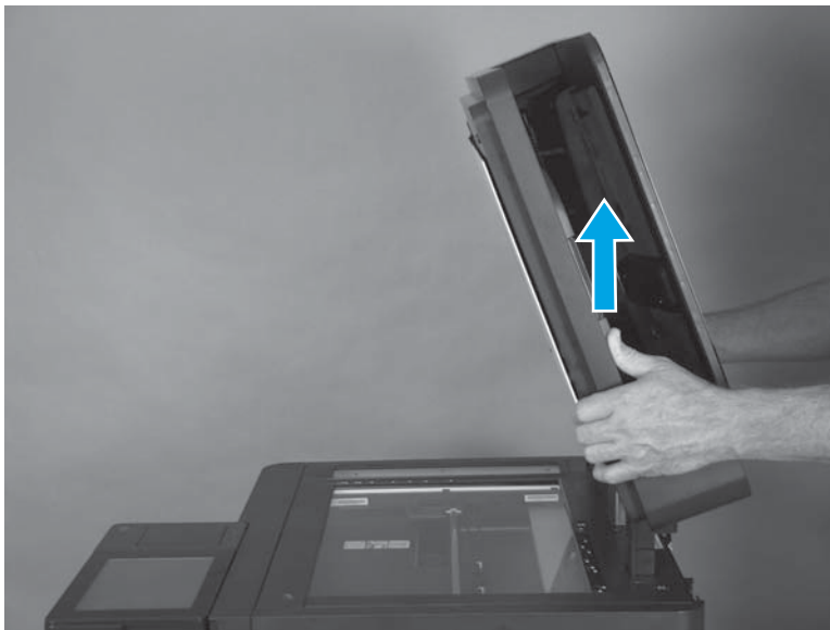
Figure 1-222 Remove the document feeder assembly (M880; 7 of 9)
