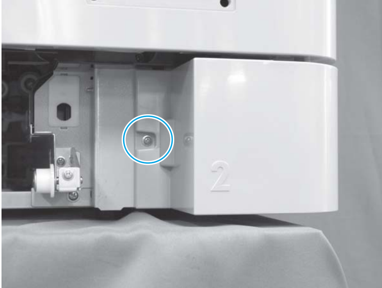
Figure 1-145 Remove the lower right cover (1 of 2)
