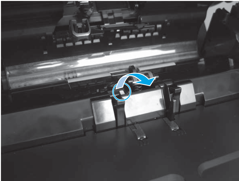
Figure 1-90 Remove the document-feeder separation pad (M880; 2 of 4)
