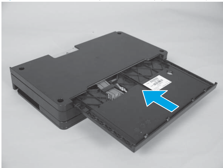
Figure 1-79 Reinstall the keyboard assembly (M880; 2 of 7)
