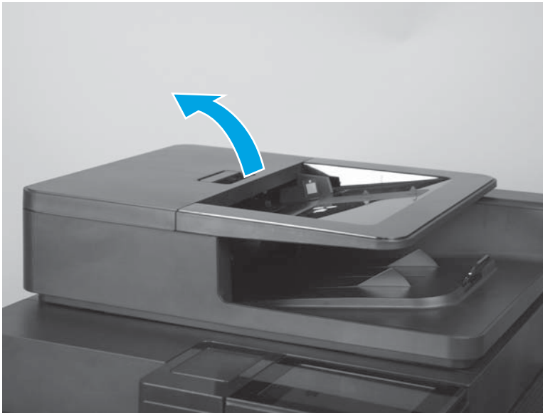
Figure 1-85 Remove the document-feeder roller (M880; 1 of 3)
