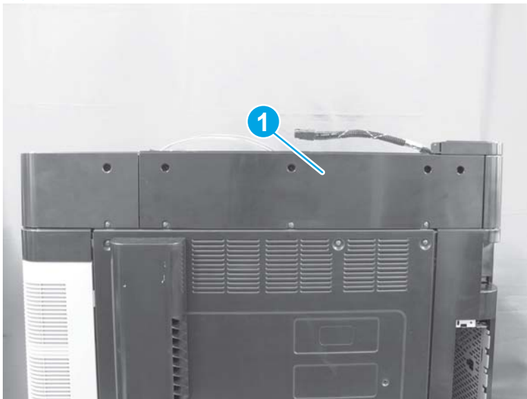
Figure 1-148 Remove the rear upper rear cover (M880; 2 of 2)
