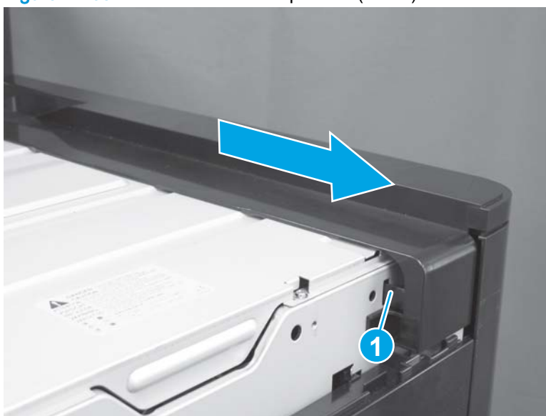
Figure 1-160 Remove the front top cover (2 of 2)
