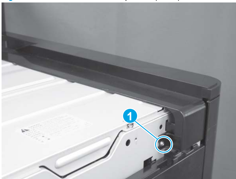
Figure 1-159 Remove the front top cover (1 of 2)
