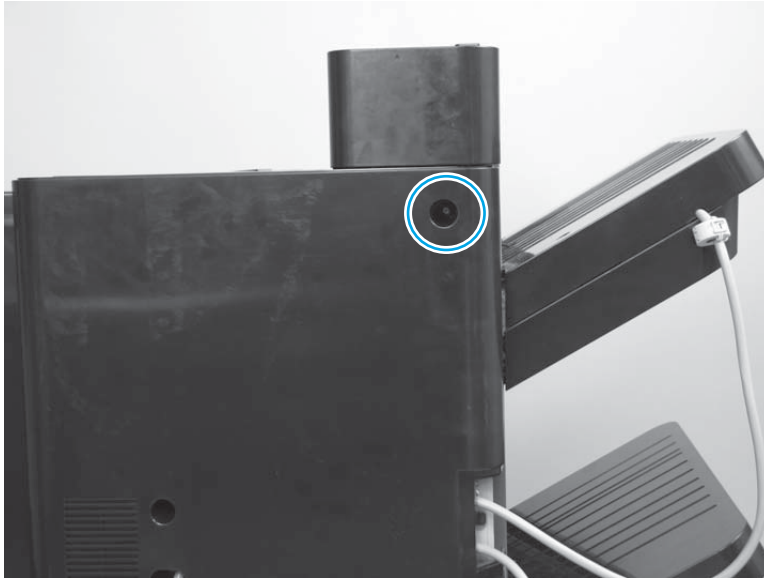
Figure 1-698 Remove the lower stepped cover assembly (2 of 5)
