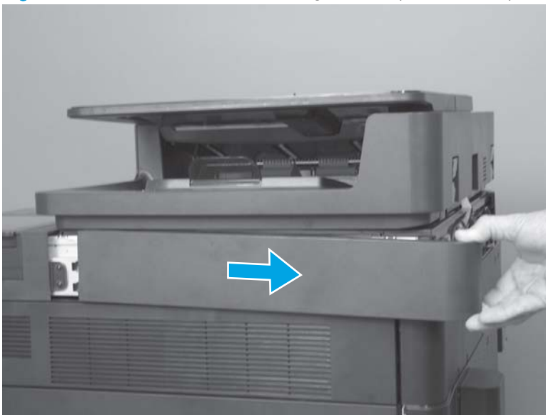
Figure 1-119 Remove the scanner right cover (M880; 2 of 2)
