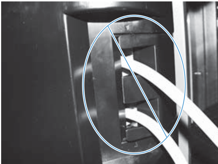
Figure 1-735 Bin cable guide cover incorrectly installed
