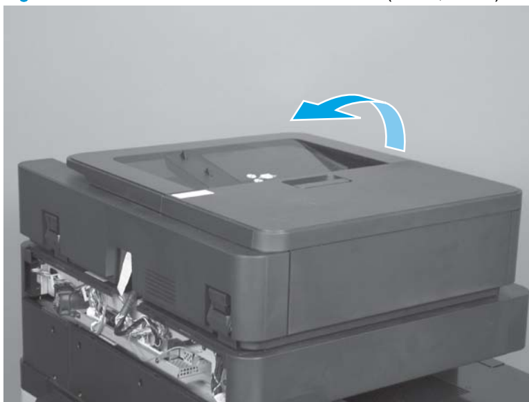
Figure 1-120 Remove the scanner front cover (M880; 1 of 8)
