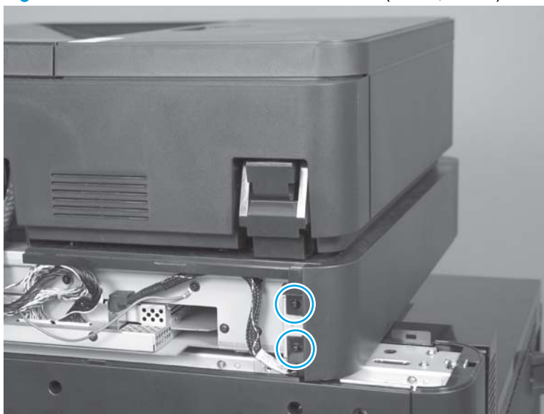
Figure 1-116 Remove the scanner left cover (M880; 1 of 2)
