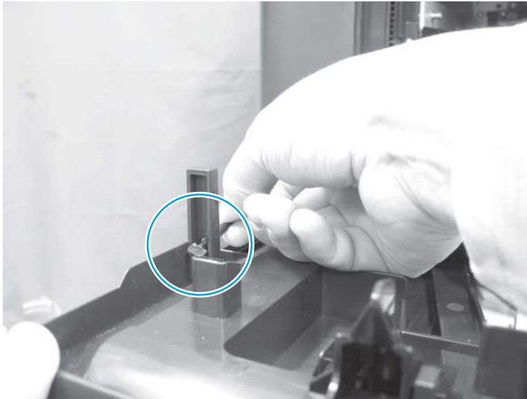
Figure 1-193 Remove the front door (1 of 9)
