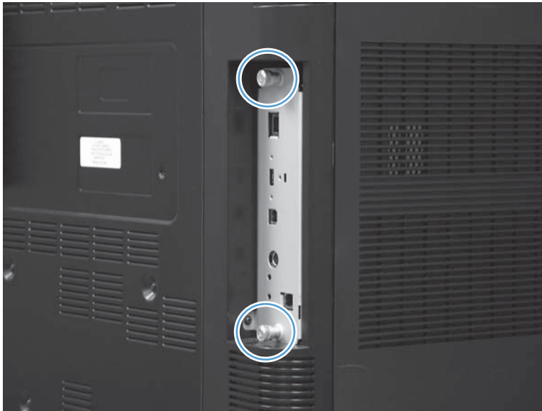
Figure 1-16 Remove the formatter (1 of 2)
