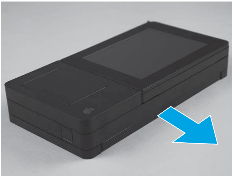
Figure 1-75 Remove the keyboard assembly (M880; 5 of 7)
