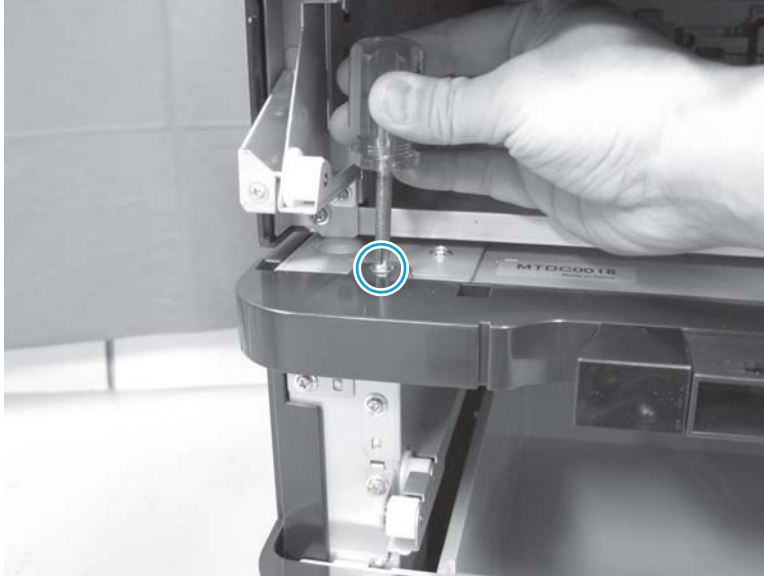
Figure 1-575 Remove the 1x500 and 3x500 upper front cover (2 of 4)
