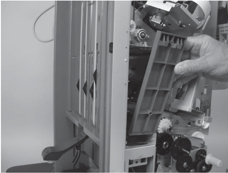
Figure 1-969 Remove the saddle delivery inner cover, front assembly (3 of 3)
