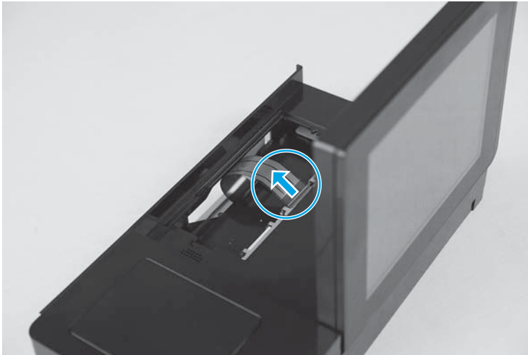
Figure 1-73 Remove the keyboard assembly (M880; 3 of 7)
