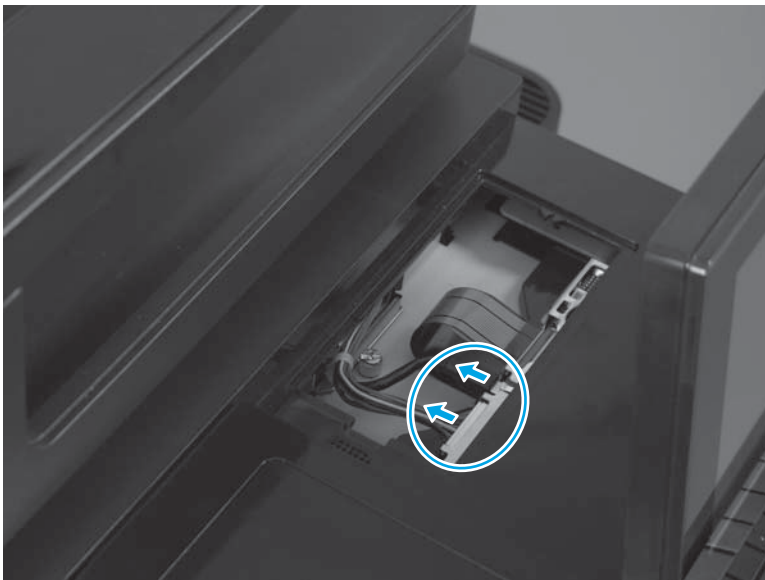
Figure 1-63 Remove the control panel assembly (M880; 4 of 8)
