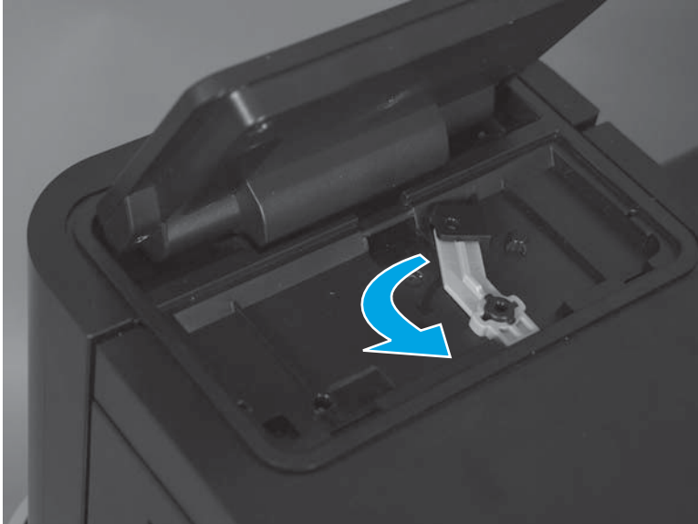
Figure 1-52 Remove the control panel assembly (M855; 4 of 10)
