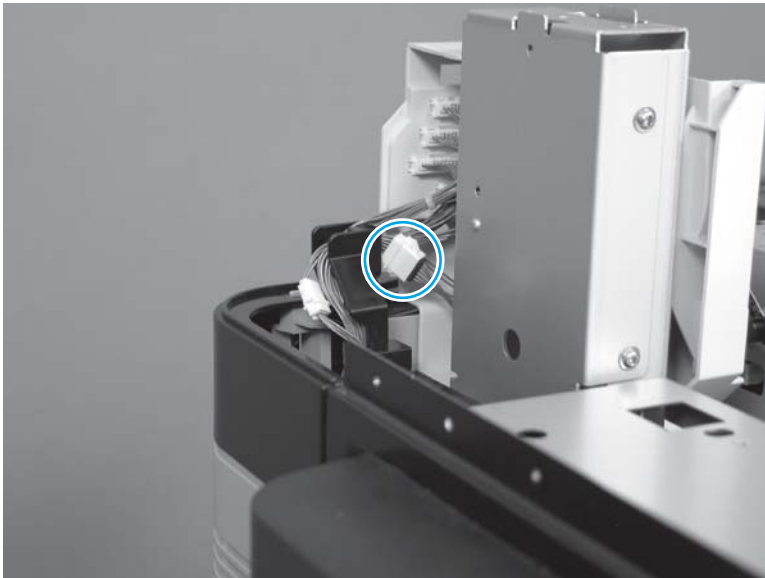
Figure 1-487 Remove the face-down delivery assembly (M855; 7 of 8)
