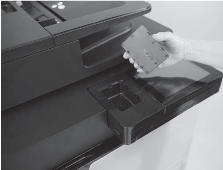
Figure 1-132 Remove the HIP cover (M880; 3 of 3)
