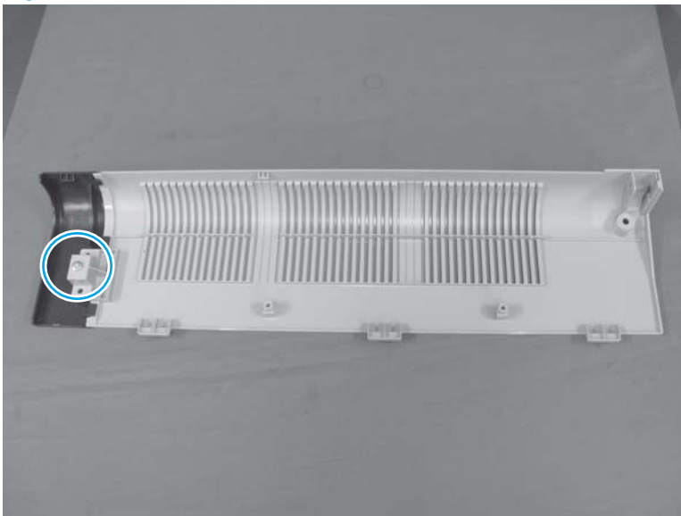
Figure 1-210 Remove the right rear cover (2 of 2)
