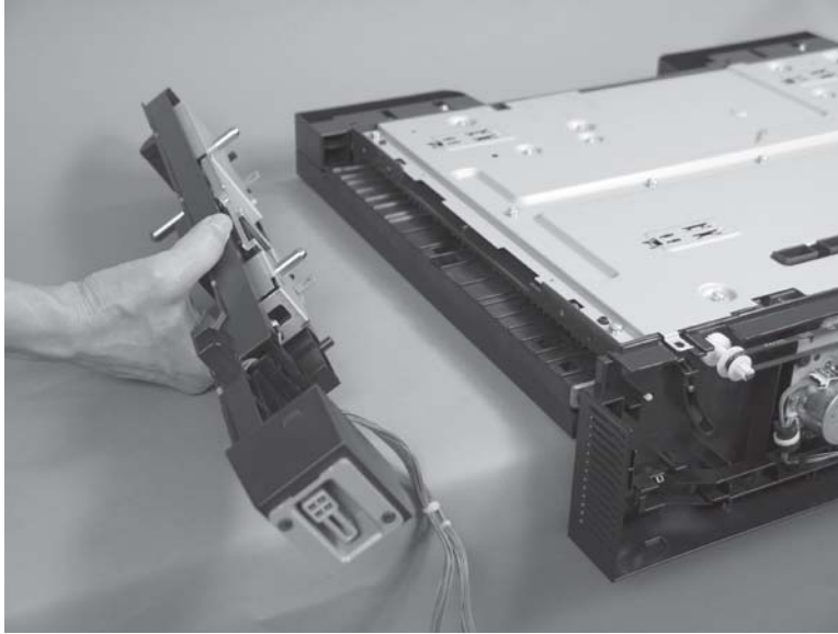
Figure 1-654 Remove the IPTU finisher lock assembly (5 of 5)
