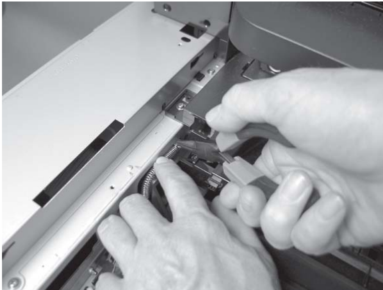
Figure 1-455 Remove the laser/scanner assembly (yellow and magenta; 4 of 6)
