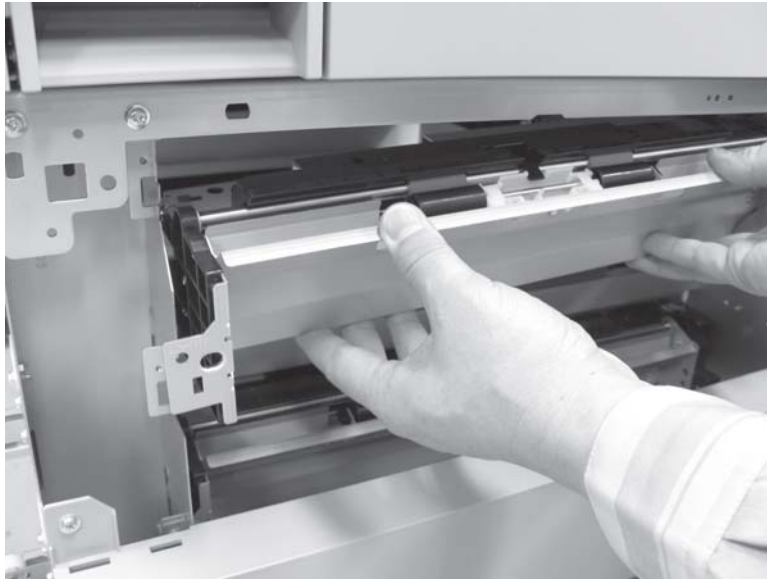
Figure 1-598 Remove the 3x500 Tray 3 pickup assembly (4 of 4)
