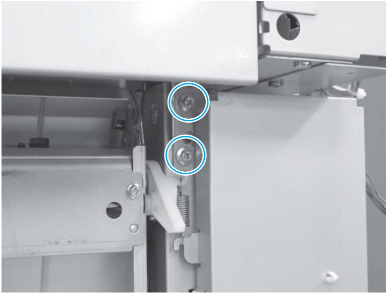
Figure 1-986 Remove the saddle feed assembly (5 of 7)
