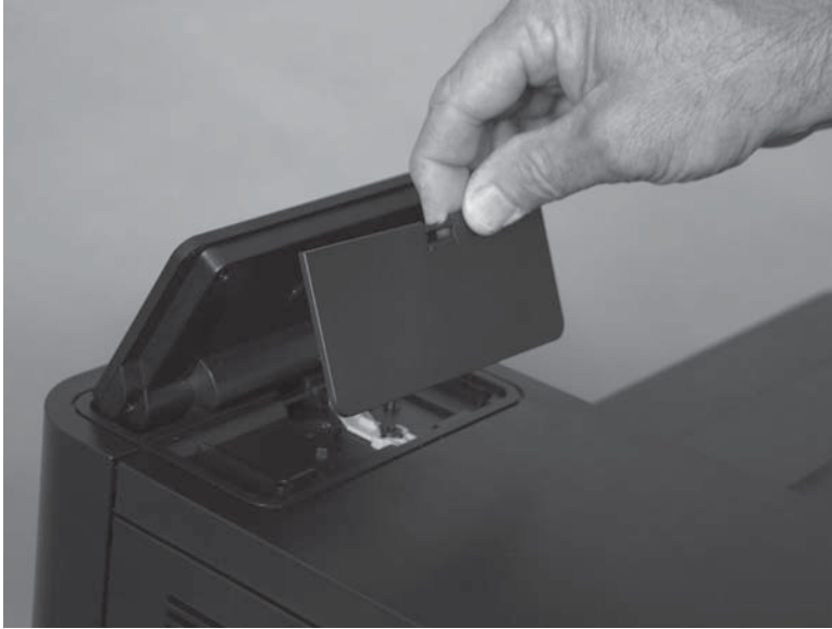
Figure 1-51 Remove the control panel assembly (M855; 3 of 10)
