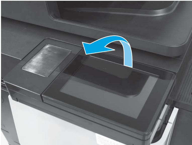
Figure 1-60 Remove the control panel assembly (M880; 1 of 8)
