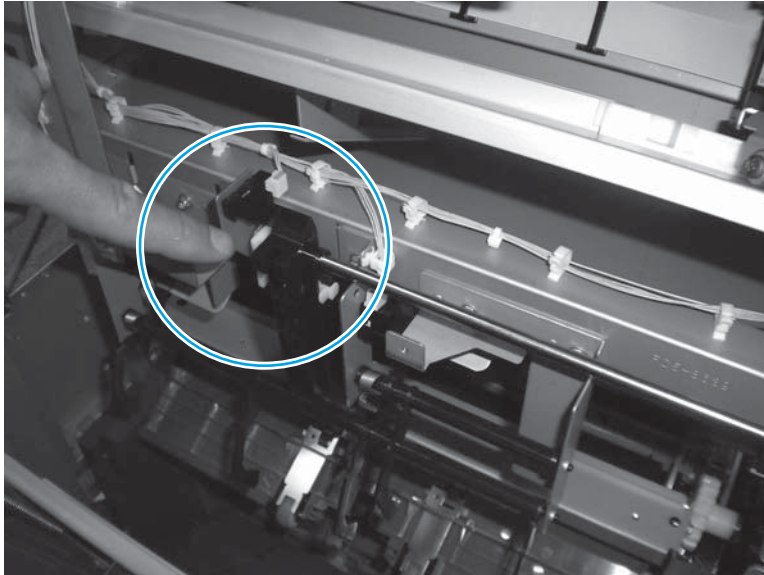
Figure 1-812 Reinstall the height wall assembly
