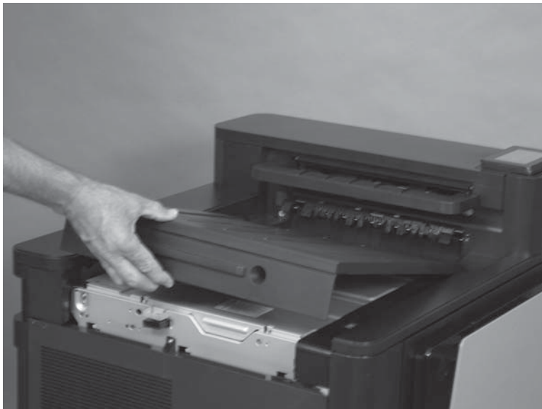
Figure 1-136 Remove the face-down bin (2 of 2)
