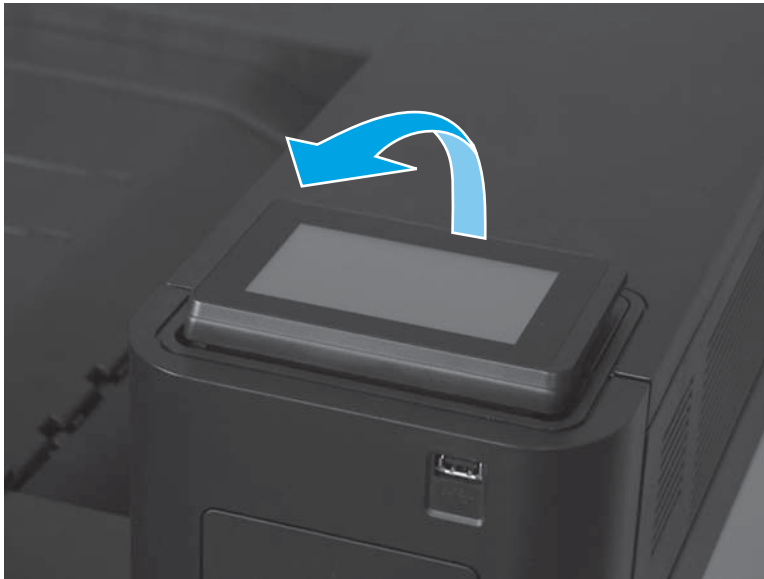
Figure 1-49 Remove the control panel assembly (M855; 1 of 10)
