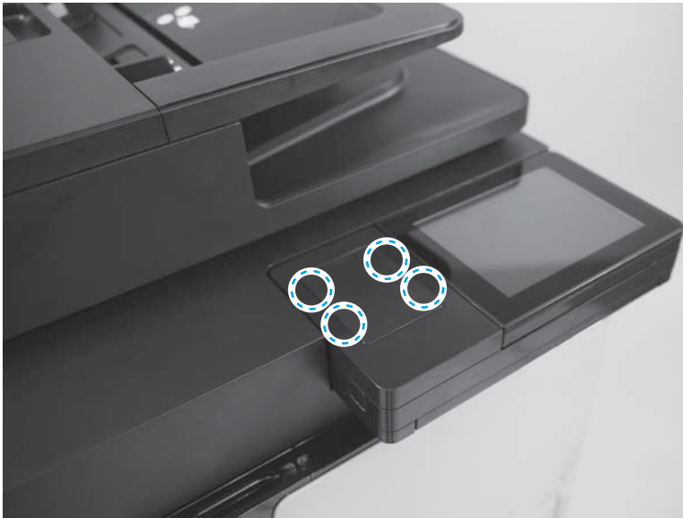
Figure 1-130 Remove the HIP cover (M880; 1 of 3)
