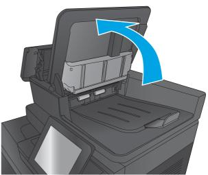
Squeeze inward on the two slots at each end of the backside-background selector assembly.
