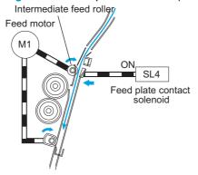
2. The solenoid turns off when the paper touches the paper-positioning plate. The feed motor continues to rotate.
