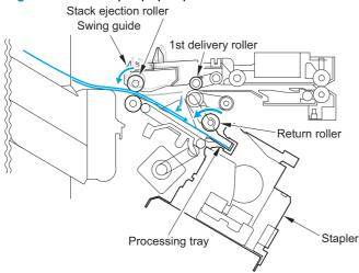
When the last sheet is aligned, the stacker controller PCA moves the aligning plate to the alignment position with the aligning motor (M103/M104) (the paper is held by the aligning plate). Then the stacker controller PCA staples at the specified staple position. After stapling, the stacker controller PCA starts the swing motor (M106) and lowers the swing guide. Then the stack is ejected by the stack-delivery roller, return roller, and stack trailing-edge assist guide.
