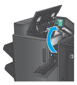
5. If paper is jammed in the bottom of the holepunch unit, carefully remove it.
