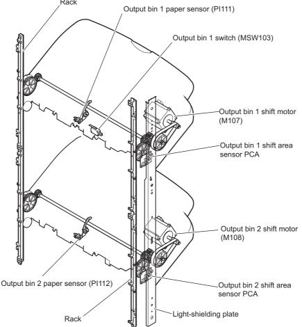
NOTE: PI111 is located on output-bin 1. PI112 is located on output-bin 2.
