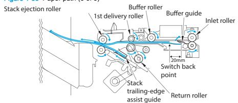
4. When the stack in the processing output bin is sent to the delivery output bin and the trailing edge of the first and second paper exits the first delivery roller, the stack-delivery roller and return roller deliver the first and second sheet to the processing output bin.
