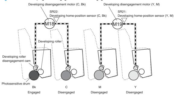
The DC controller rotates the developing disengagement motor and changes the direction of the cam according to the instructions from the formatter for each print job.
