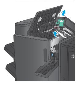
6. Lift the jam access cover for the output slot, and gently remove any jammed paper.
