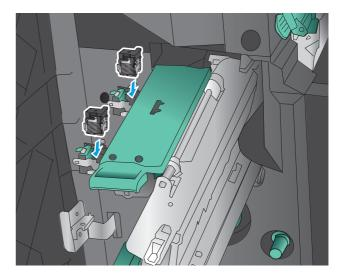
Pull the handle of the staple cartridge unit toward you and rotate it downward to its original position. Lock it into position by pushing in the handle.
