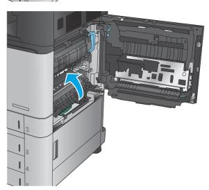
8. If paper is jammed in the fuser, lift the jamaccess cover on top of the fuser, and gently pull out the paper.
