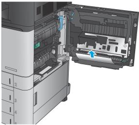
Check for paper in the duplex-printing path inside the right door. If paper is near the top of the duplex-printing path, gently pull it out to remove it.
