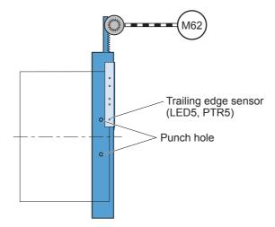
When the hole punching operation is completed, the hole punch controller drives the hole punch feed motor and reverses the side registration motor so that the hole punch slide assembly moves back to its home position.
