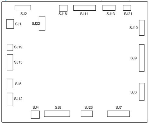
Table 2-36 Saddle stitcher controller PCA connectors (BM and BMHP)
