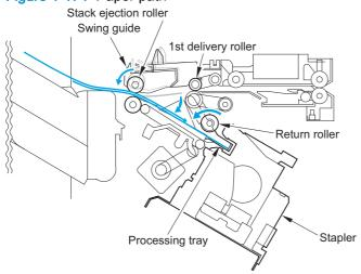
When the last sheet is aligned, the stacker controller PCA moves the aligning plate to the alignment position with the aligning motor (M103/M104) (the paper is held by the aligning plate). Then the stacker controller PCA staples at the specified staple position. After stapling, the stacker controller PCA starts the swing motor (M106) and lowers the swing guide. Then the stack is ejected by the stack-delivery roller, return roller, and stack trailing-edge assist guide.
