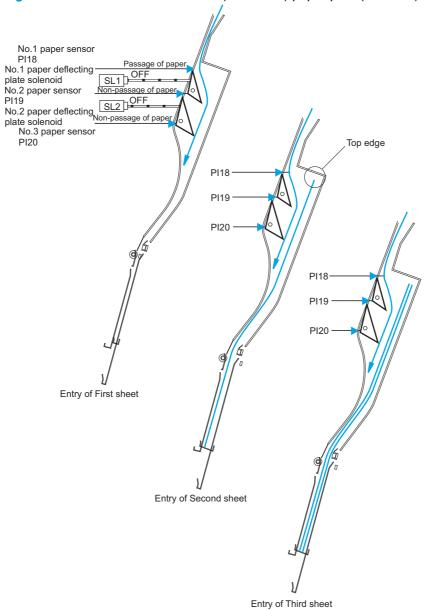
Figure 1-136 B4/LGL paper path (3 sheets) Passage of paper No.1 paper sensor PI18 No.2 paper sensor PI19 ssage of paper No.3 paper sensor Non-passage of paper PI20 PI18 PI19 PI20 PI18 PI19 PI20 Entry of First sheet Entry of Second sheet
