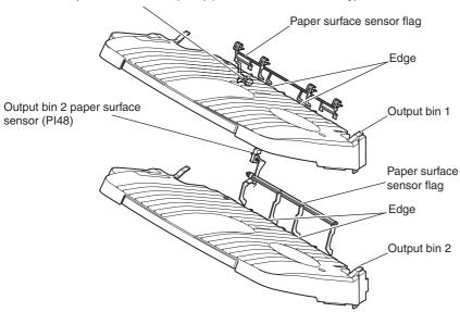
When the output bin capacity is reached, the ON/OFF combinations of the area sensors (PS981, PS982 and PS983) are used to determine an over-stacking condition. Area sensor conditions are as follows:
