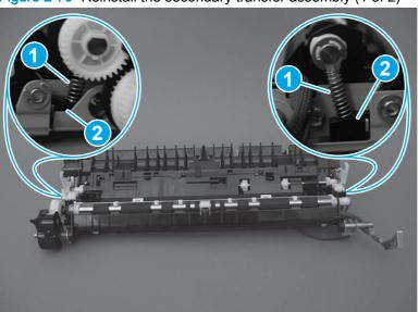
Figure 2-79 Reinstall the secondary transfer assembly (1 of 2)
