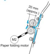
The paper-folding rollers rotate forward to push the stack forward. The paper-pushing plate returns to its home position.
