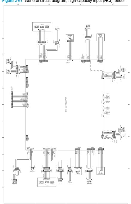
Figure 2-67 General circuit diagram, high-capacity input (HCI) feeder
