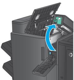
Hole punch models only: If paper is jammed in the bottom of the hole-punch unit, carefully remove it.
