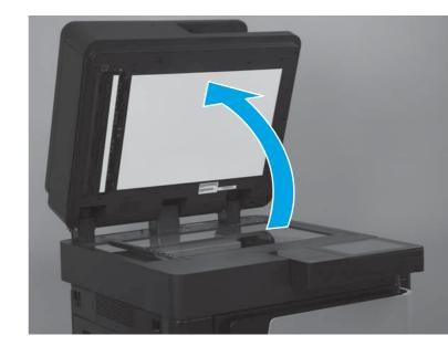
3. Clean the main scanner glass (callout 1), the document-feeder glass (the small strip of glass on the left side of the scanner, callout 2), and the white backing (callout 3). Use a soft cloth or sponge that has been moistened with nonabrasive glass cleaner. Dry the glass and white plastic backing by using a chamois or a cellulose sponge to prevent spotting.
