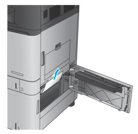
10. Close the jam-access door on the right side of the high-capacity tray cabinet.
