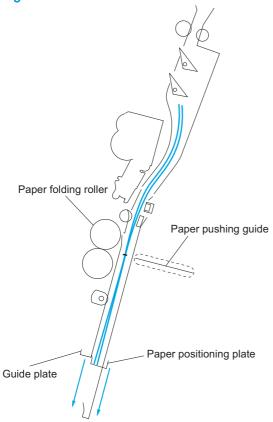
The paper-postioning plate moves the stack to the paper-folding rollers that hold the stack at its center and fold it. The paper-folding rollers and delivery roller then output the stack to the output bin.
