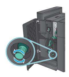
**14.** Press the large jam-release knob, and then turn it clockwise.
