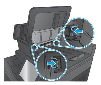
Remove the backside-background selector assembly by pulling it out.
