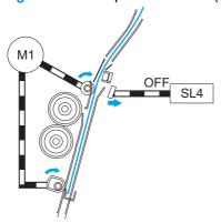
3. The solenoid turns on when the next sheet arrives, and the feed plate comes into contact with the page.
