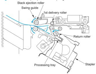
Figure 1-101 Rollers and sensors for stapling
