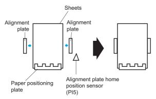
2. The alignment plates move away from the stack and then return (Second alignment).
