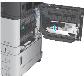
5. Lift the green handle on the transfer-access panel and open the panel.
