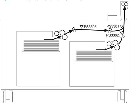
Table 2-20 High-capacity input (HCI) feeder jam sensors
