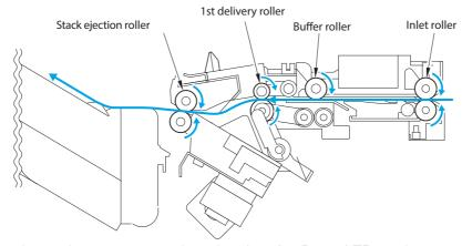
When the product sorts paper size other than A4, B5, or LTR or when set to staple and sort, copies are delivered to the processing output bin for aligning and stapling and then ejected using the stack trailing-edge assist.
