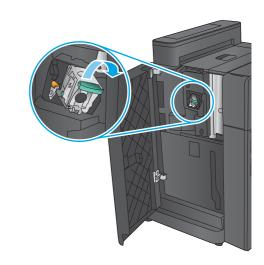
Lift up the metal handle on the front of the staple cartridge.
