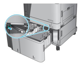
If jammed paper is in the feed area, pull it down to remove it.
