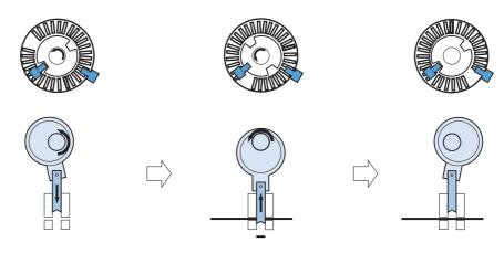
Punch shaft stops: Home position for 3-hole Punch shaft turns 90 degrees ccw.: Operates 2-hole punching
