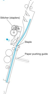
The booklet maker unit folds the stitched stack, and then feeds it to where the stapling position matches the height of the paper-pushing plate and the paper-folding roller nip. The paper-positioning plate moves the stack forward and the guide plate descends so that the paper-folding rollers directly face the stack.
