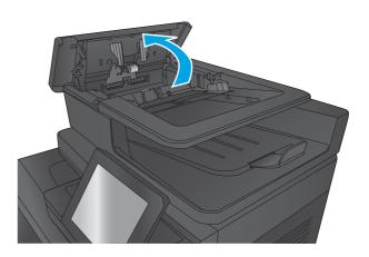
Lift the jam-access door, and remove any jammed paper.
