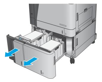
Remove the paper from the trays and discard any damaged sheets.
