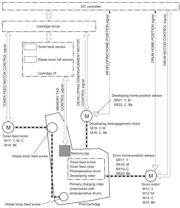
The drum motor causes the photosensitive drum to rotate. That rotation causes the primary charging roller to rotate. The drum motor also drives the toner feed screw, the toner feed roller, and the developing roller to transfer toner from the toner cartridge onto the imaging drum.
