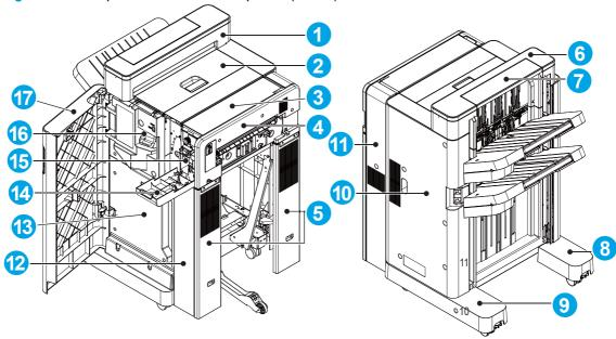
Table 2-53 Stapler/stacker with hole punch (SSHP) covers
