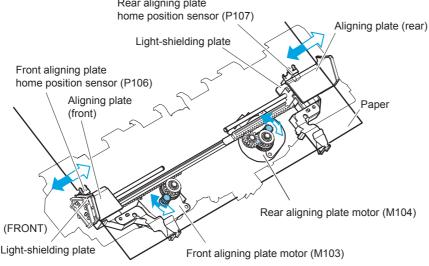
Figure 1-164 Stack job offset example
