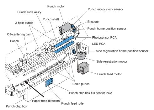
2-hole/4-hole puncher assembly
