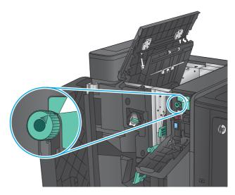
5. Hole punch models only: Lift the hole-punch unit.
