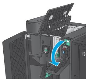
4. Hole punch models only: Turn the knob to align the arrows.
