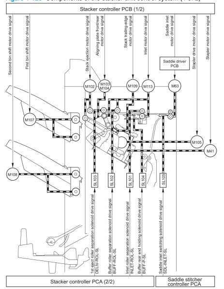
Figure 1-125 Components of the stacker unit control system (1 of 2)
