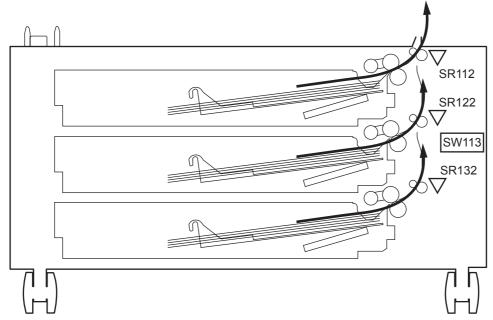
Table 2-22 1x500-sheet and 3x500-sheet paper feeder jam sensors and switch
