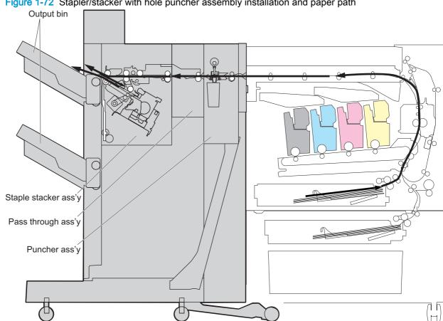
Figure 1-72 Stapler/stacker with hole puncher assembly installation and paper path
