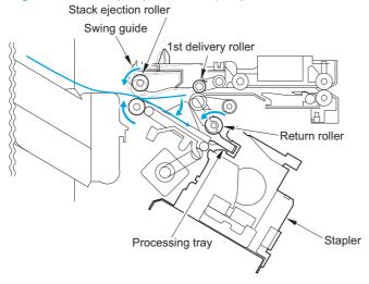
Figure 1-173 Rollers and sensors for stapling
