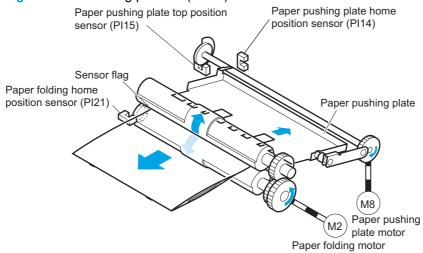
Figure 1-155 Folding start position (3 of 5)
