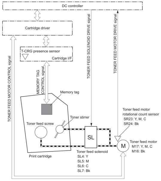
The toner feed screw rotates, picks up the toner particles, and transports them into the imaging drum. The toner stirrer rotates at the same time as the toner feed screw to keep the toner particles from sticking to each other.
