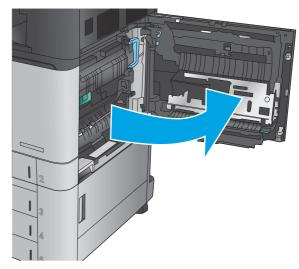
Lift the green handle on the transfer-access panel and open the panel.
