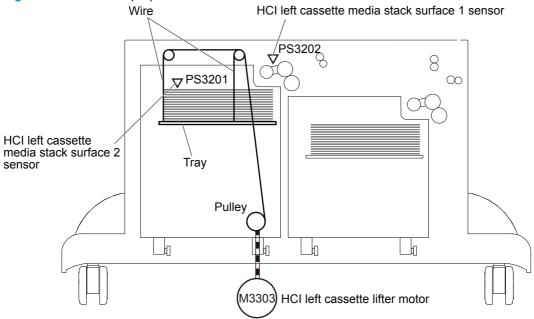
The figure above illustrates the mechanism for the left cassette, but each HCl cassette has the same mechanism.
