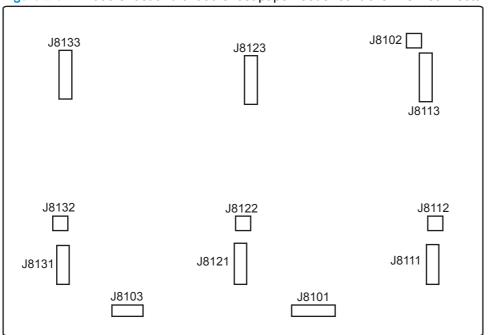
Table 2-32 11x500-sheet and 3x500-sheet paper feeder controller PCA connectors
