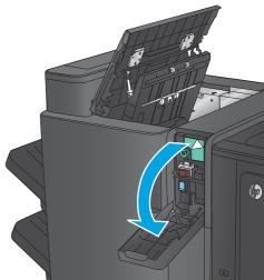
3. Hole punch models only: Turn the knob to align the arrows.
