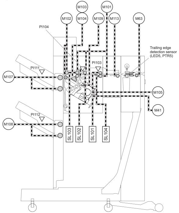
Table 1-46 Stapler/stacker with hole puncher assembly feed-and-delivery electrical components
