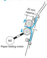
3. The paper-folding rollers rotate in reverse, pushing the stack backward 20 mm (reverse feeding).
