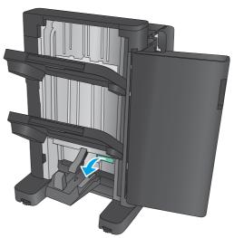
**13.** Turn the small jam-release knob counterclockwise.
