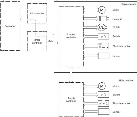
Table 1-42 Stapler/stacker electrical components (1 of 2)
