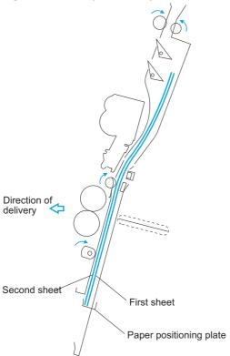
The alignment plates put paper in order when it is output to the vertical-path assembly. Mounted at the edge of the-vertical path assembly, alignment plates also prepare the stack for delivery after stapling.
