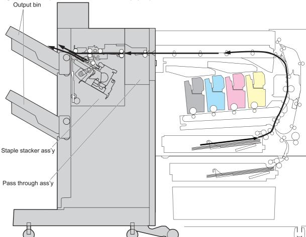
Figure 1-71 Staple/stacker installation and paper path
