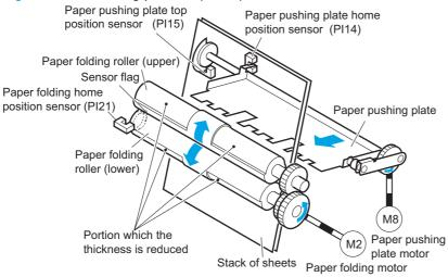
Figure 1-154 Folding process (2 of 5)
