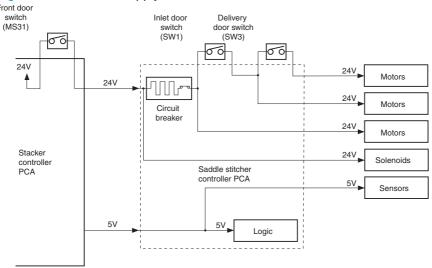
Figure 1-116 Power-supply route for the stacker unit
