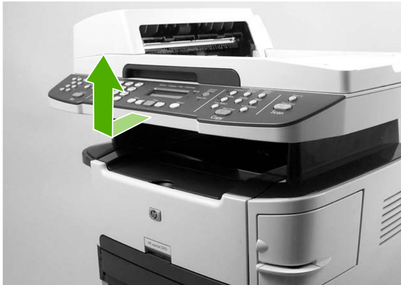
Figure 5-30 Remove the scanner/ADF assembly (3 of 3)
