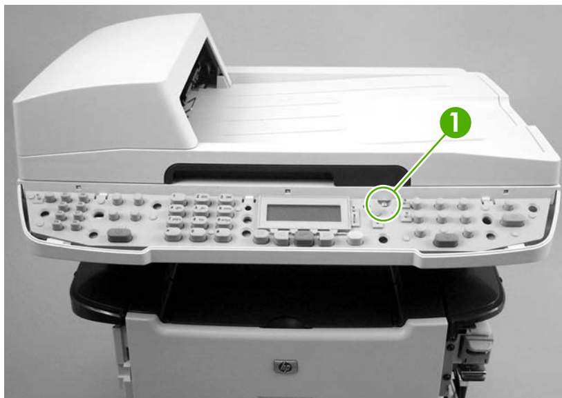
Figure 5-32 Remove the bezel and control panel (2 of 4)
