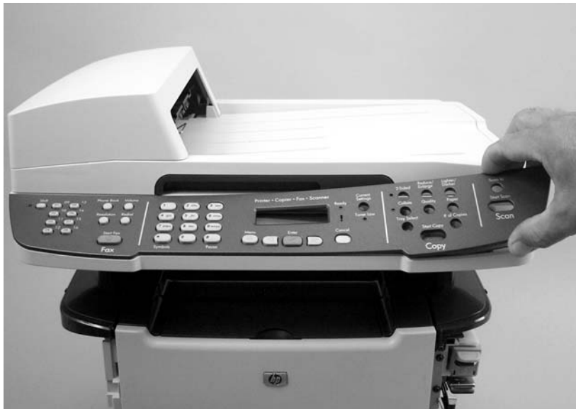
Figure 5-31 Remove the bezel and control panel (1 of 4)
