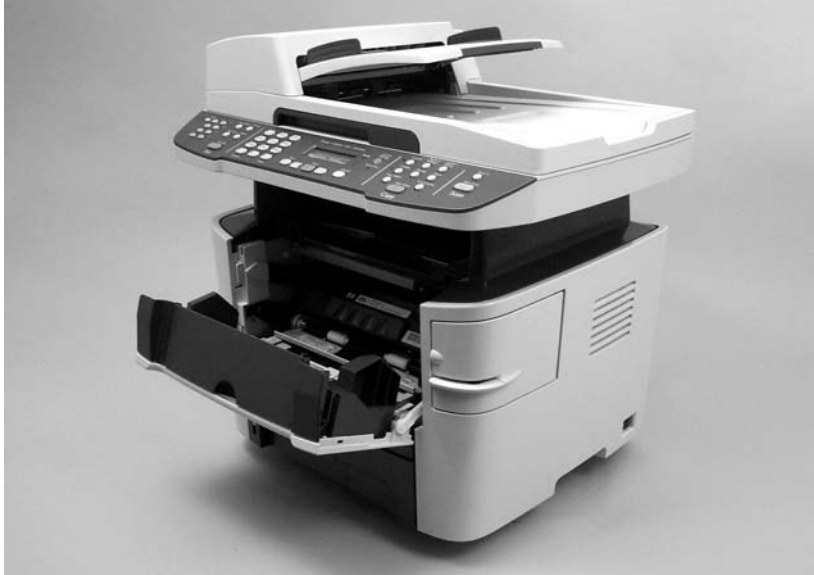
Figure 5-3 Remove the print cartridge (1 of 2)
