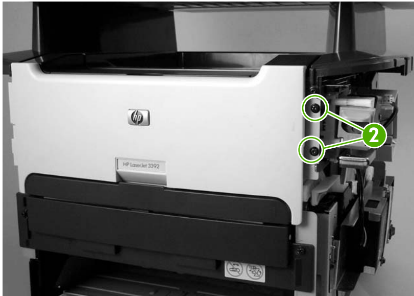
Figure 5-36 Remove the convenience-stapler assembly (2 of 2)
