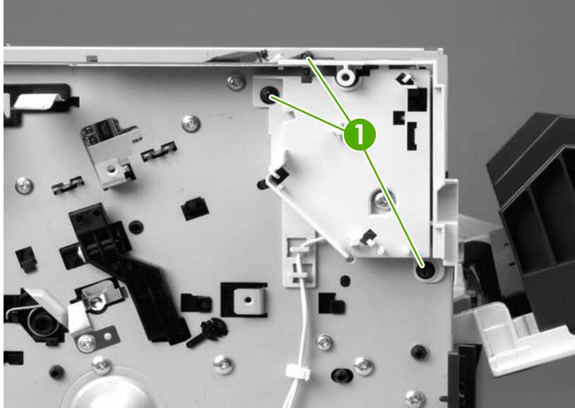
Figure 5-70 Remove the interlock assembly (1 of 2)
