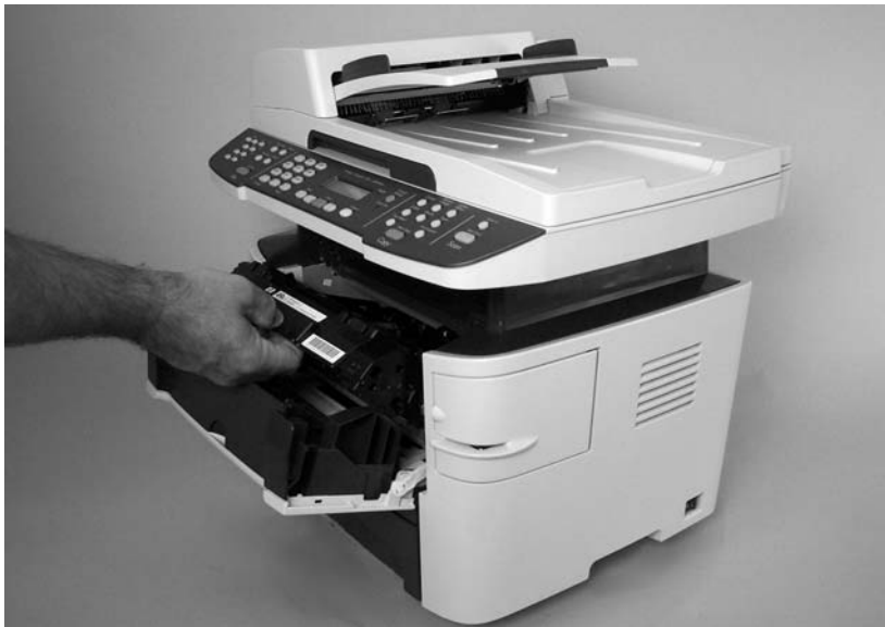
Figure 5-4 Remove the print cartridge (2 of 2)
