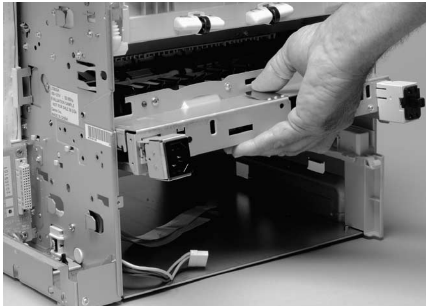
Figure 143. Power supply (5 of 5)
