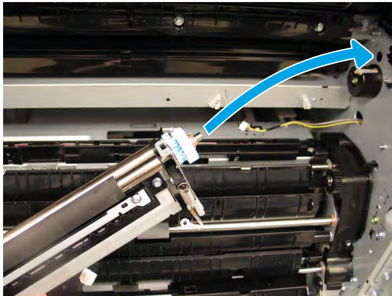
Figure 2-445 Install the gear side of the shaft
