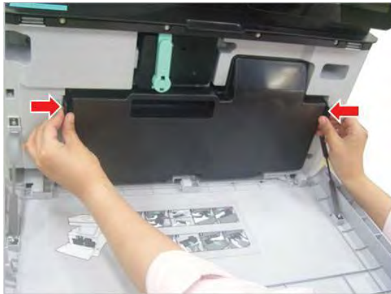
Figure 2-464 Remove the TCU
