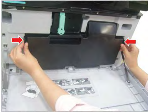
Figure 2-55 Remove the TCU
