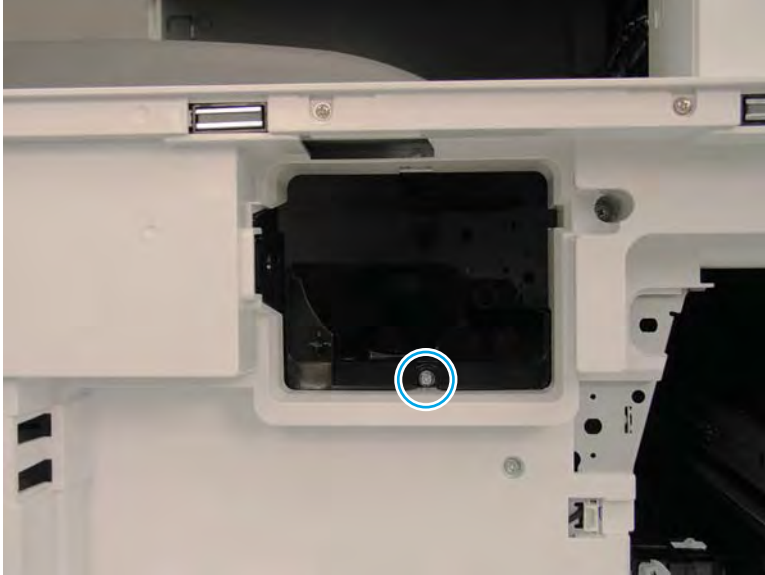
Figure 2-226 Remove one screw
