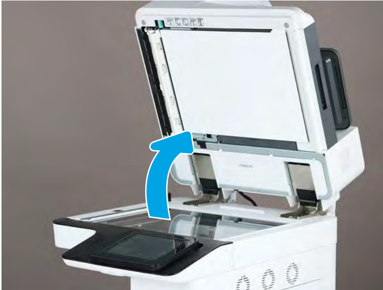
Figure 2-8 Open document feeder unit
