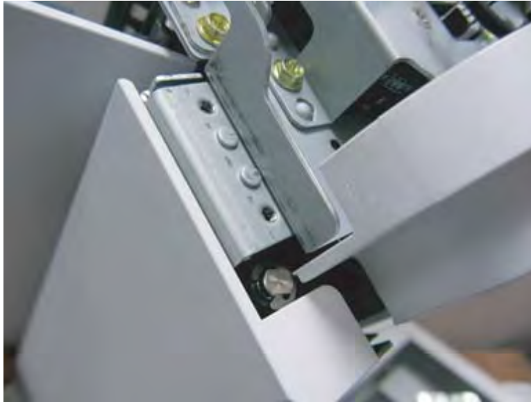
Figure 2-867 Pry the scan in lower assembly away from the ADF
