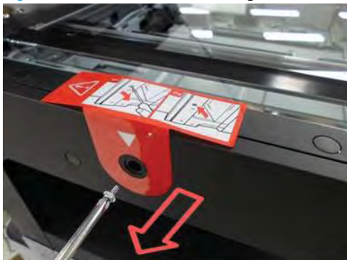
Figure 1-44 Remove scan locking screw
