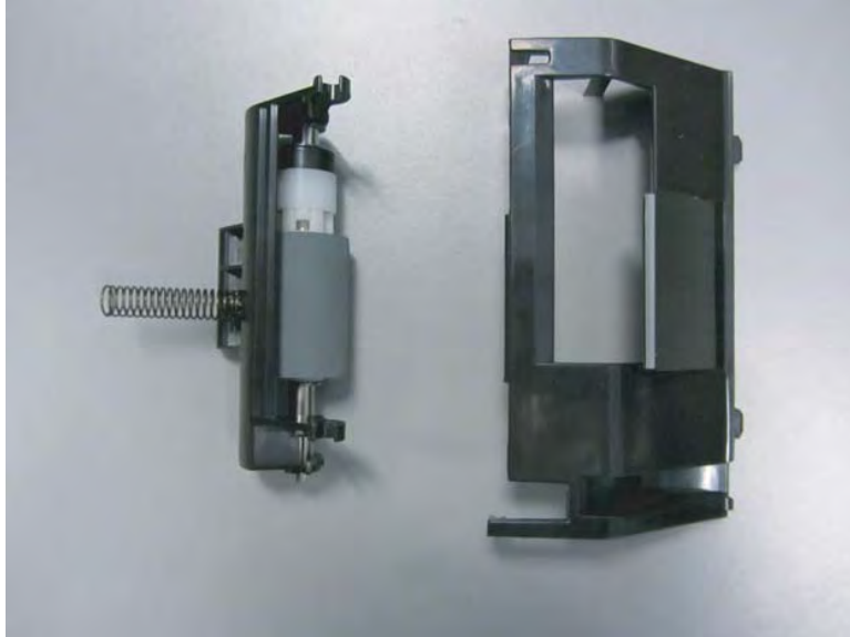
Figure 2-733 Document feeder separation roller cover and roller assembly
