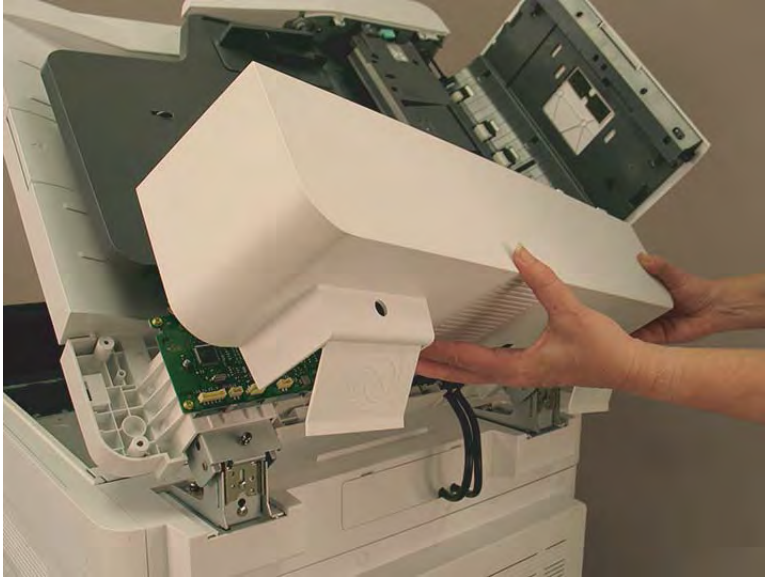
Figure 2-849 Remove back cover.
