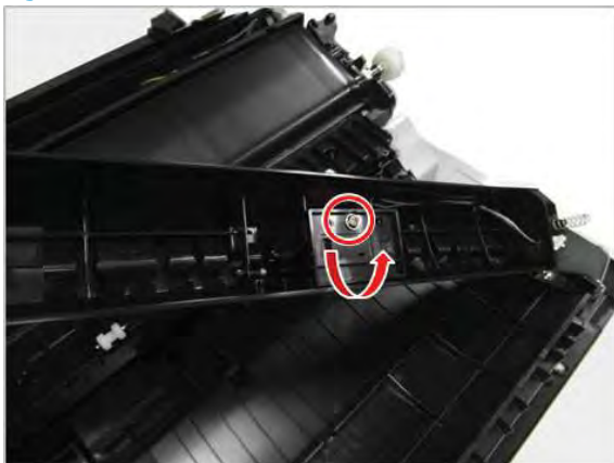
Figure 2-566 Remove one screw
