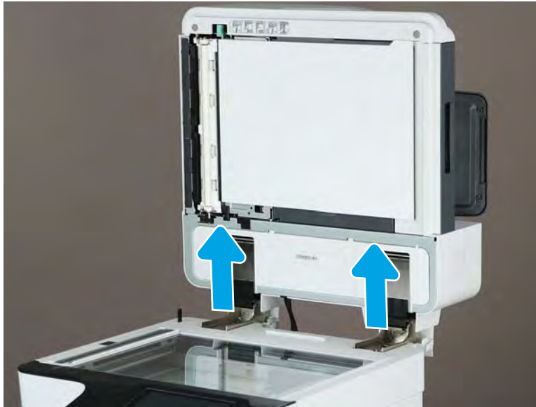
Figure 2-876 Remove two screws and lift up to remove ADF
