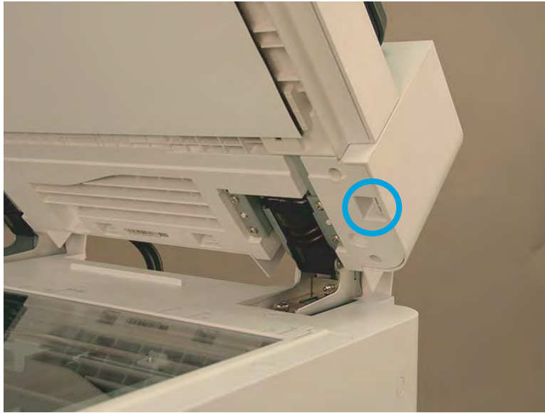
Figure 2-861 Release one tab on the right side of back cover.
