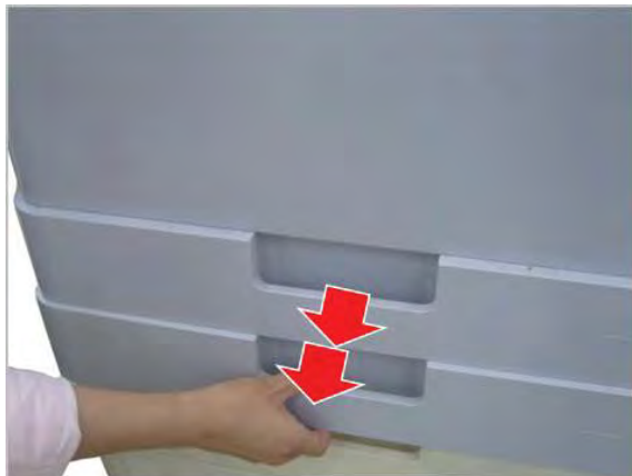
Figure 2-526 Remove the two cassettes
