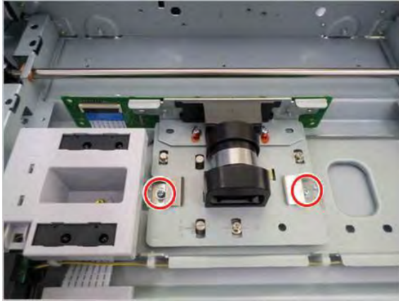
Figure 2-901 Remove screws and release scanner imaging unit
