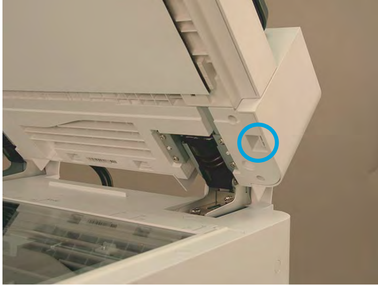
Figure 2-796 Release one tab on the right side of back cover.
