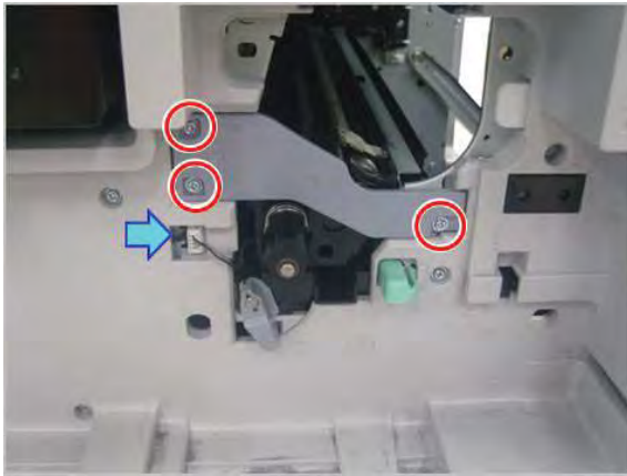
Figure 2-53 Remove three screws and disconnect the small, black cable connector
