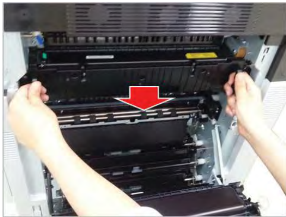
Figure 2-100 Fuser unit removal
