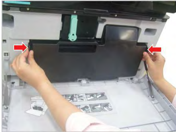
Figure 2-56 Remove the TCU
