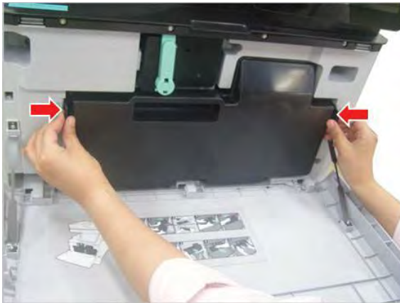
Figure 2-367 Remove the TCU
