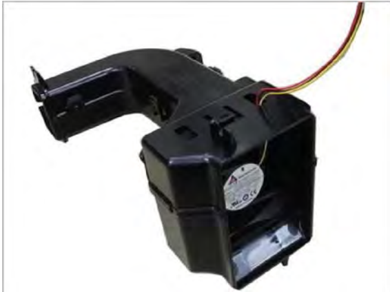
Figure 2-186 Release five tabs
