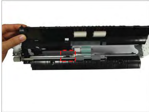
Figure 2-303 Remove prefeed sensor 2
