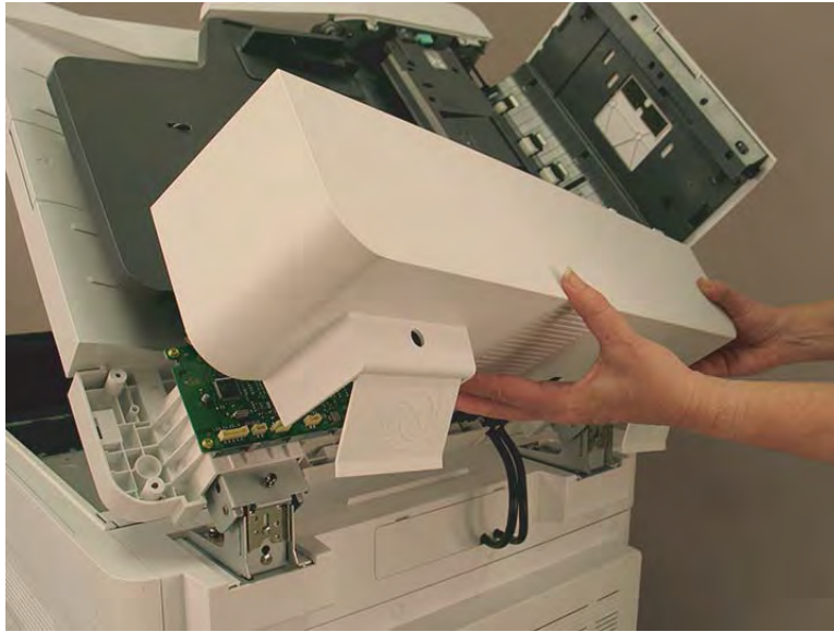
Figure 2-694 Remove back cover.
