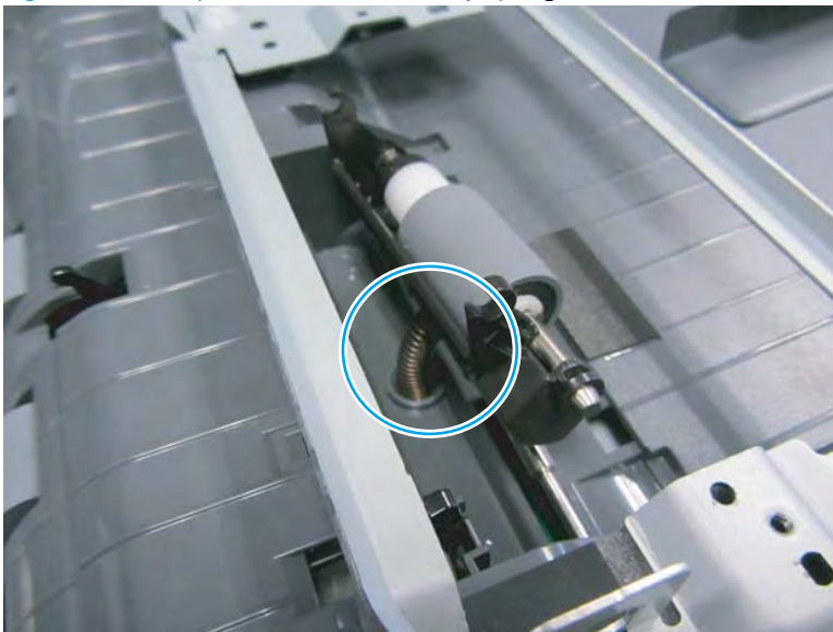
Figure 2-735 Separation roller assembly spring
