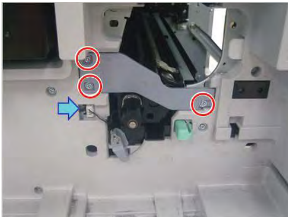
Figure 2-219 Remove three screws and disconnect the small, black cable connector
