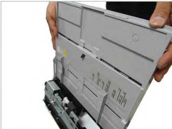
Figure 2-628 Remove the Tray 1 tray upper
