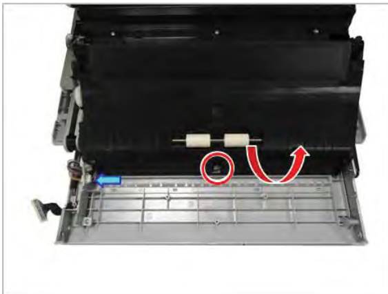
Figure 2-616 Remove the feed guide take away upper
