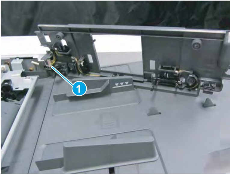
Figure 2-715 Turn the cover over and disconnect connector
