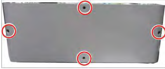
Figure 2-960 Remove the rear cover
