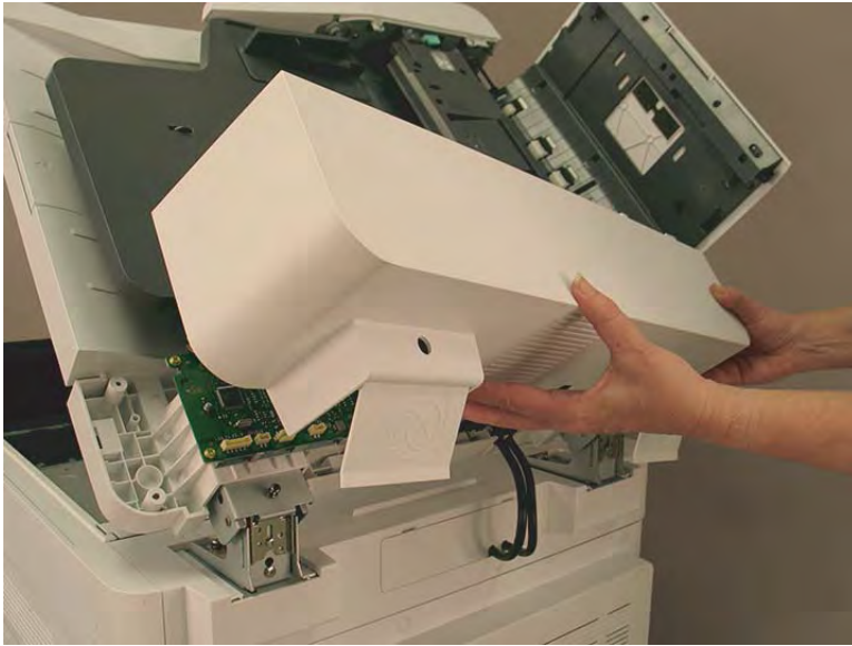
Figure 2-830 Remove back cover.
