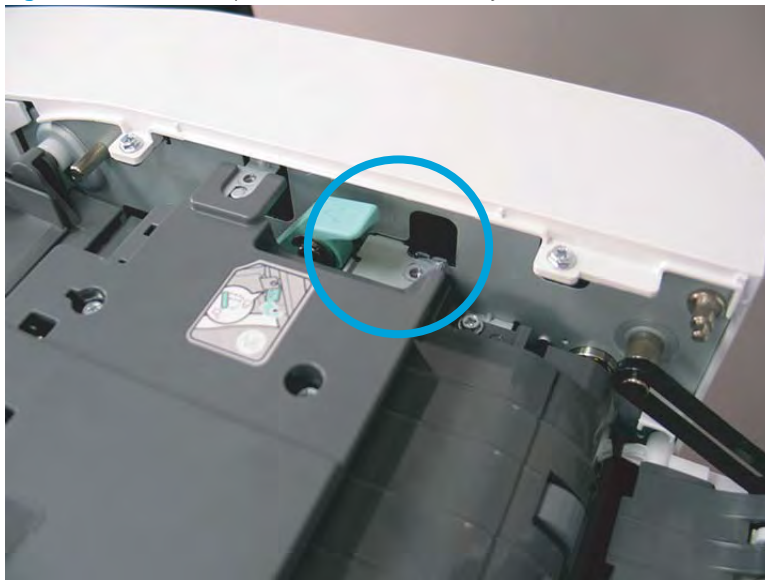
Figure 2-699 Rotate pick/feed roller assembly to release sheet metal tab from ADF frame.
