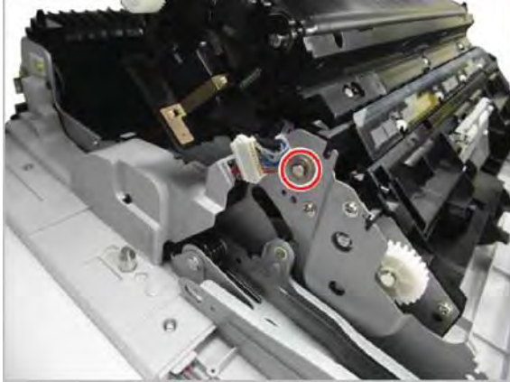
Figure 2-544 Remove one e-ring and bushing
