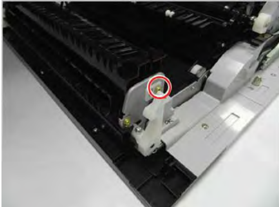
Figure 2-564 Remove one screw
