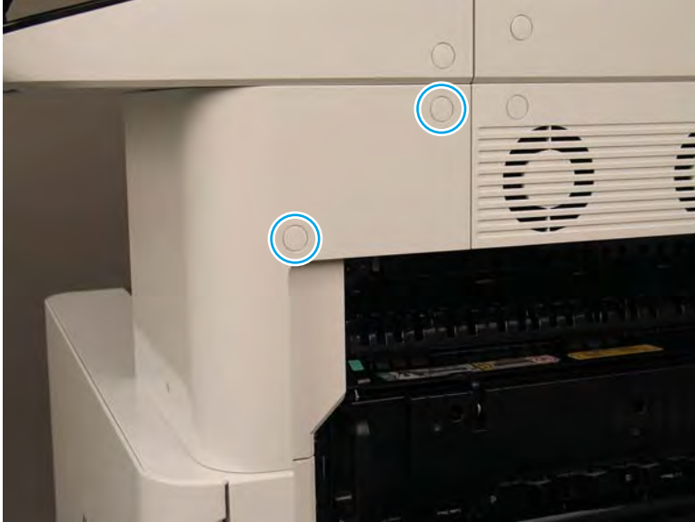
Figure 2-264 Remove two screws and rotate the cover
