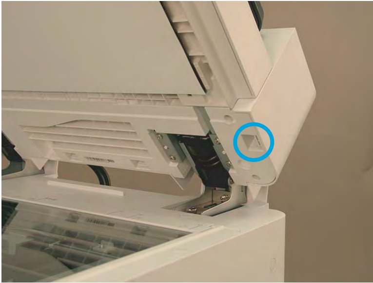
Figure 2-684 Release one tab on the right side of back cover.
