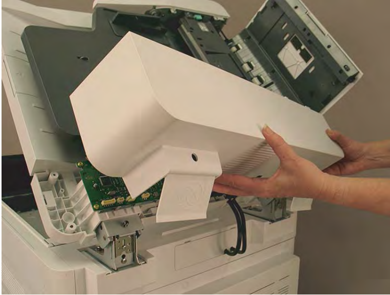
Figure 2-820 Remove back cover.
