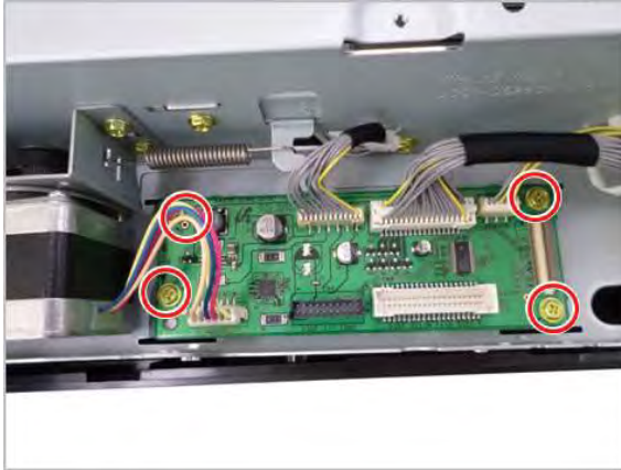
Figure 2-881 Remove screws and release scanner PCA
