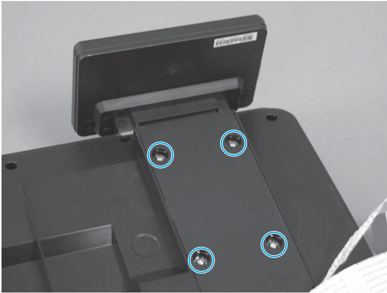
Figure 1-66 Remove the control panel (1 of 4)
