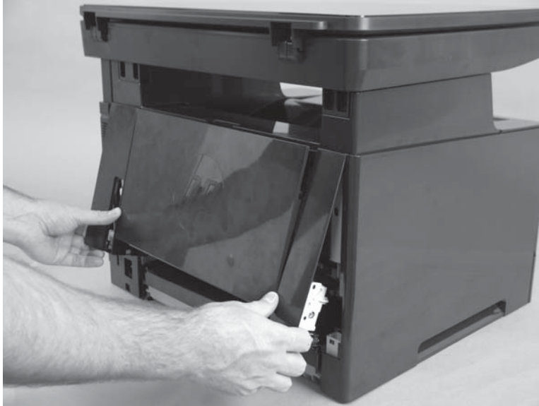
Figure 1-27 Remove the rear-cover assembly (2 of 2)
