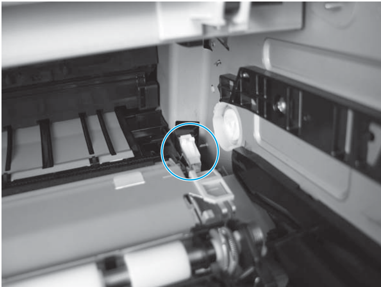
Figure 1-113 Remove the low-voltage power supply PCA (2 of 6)
