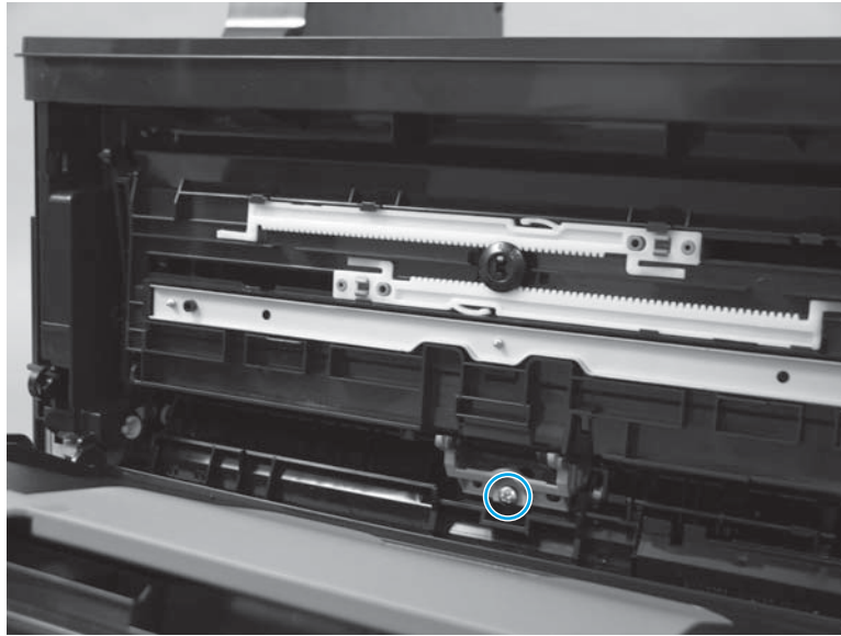
Figure 1-8 Remove the tray 1 separation pad (3 of 4)
