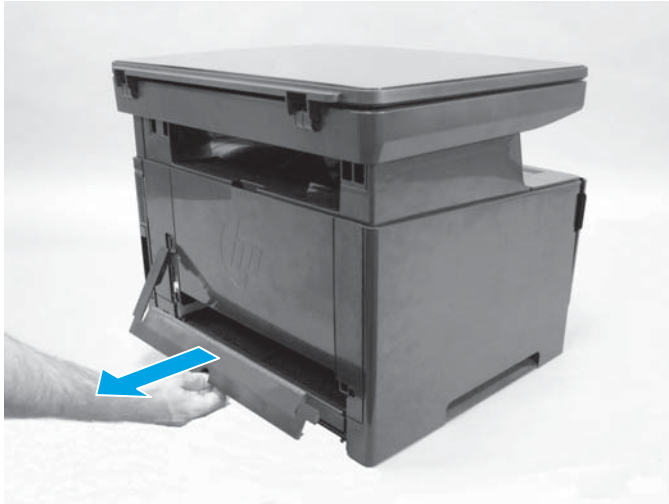
Figure 1-25 Remove the lower back cover
