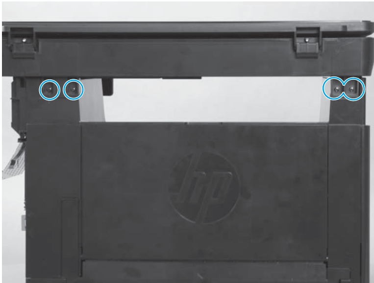
Figure 1-62 Remove the SSA (5 of 6)
