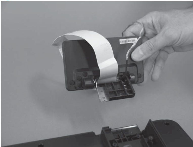
Figure 1-69 Remove the control panel (4 of 4)
