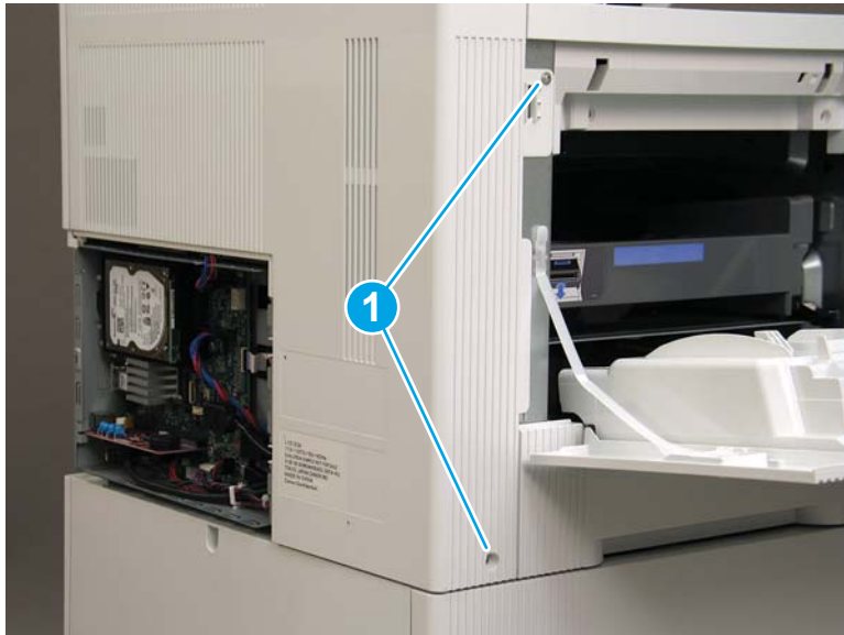
Figure 1-201 Remove two screws
