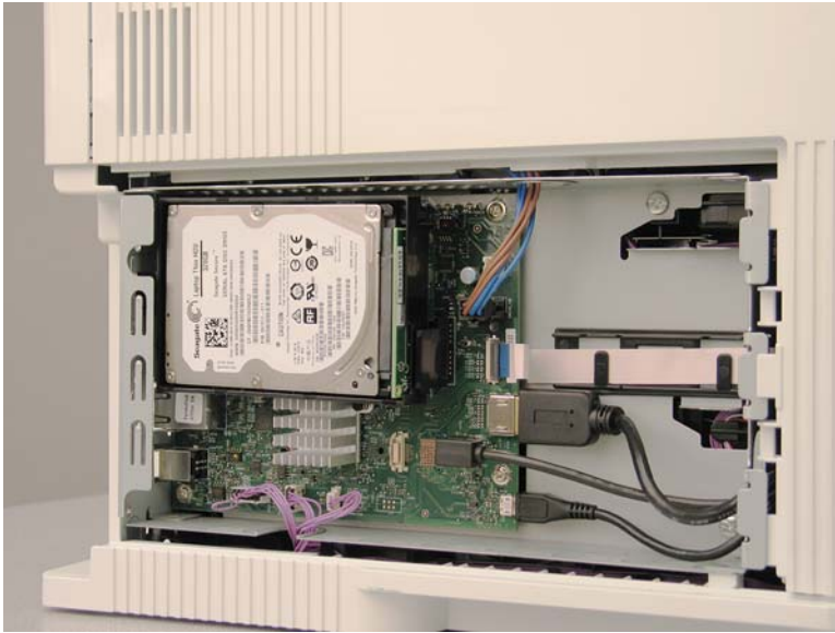
Figure 1-1966 Locate the space for installing the internal USB ports/AA module
