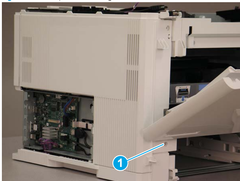
Figure 1-2155 Open the cartridge door and remove one screw
