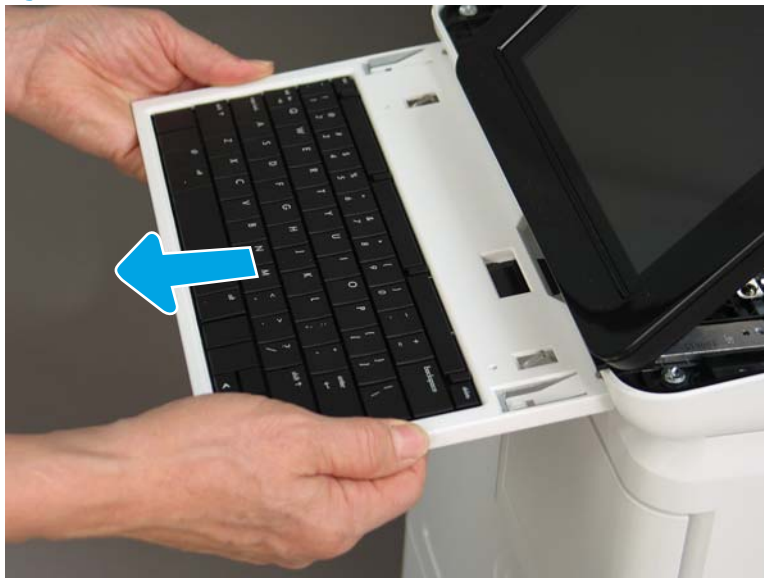
Figure 1-609 Remove the keyboard
