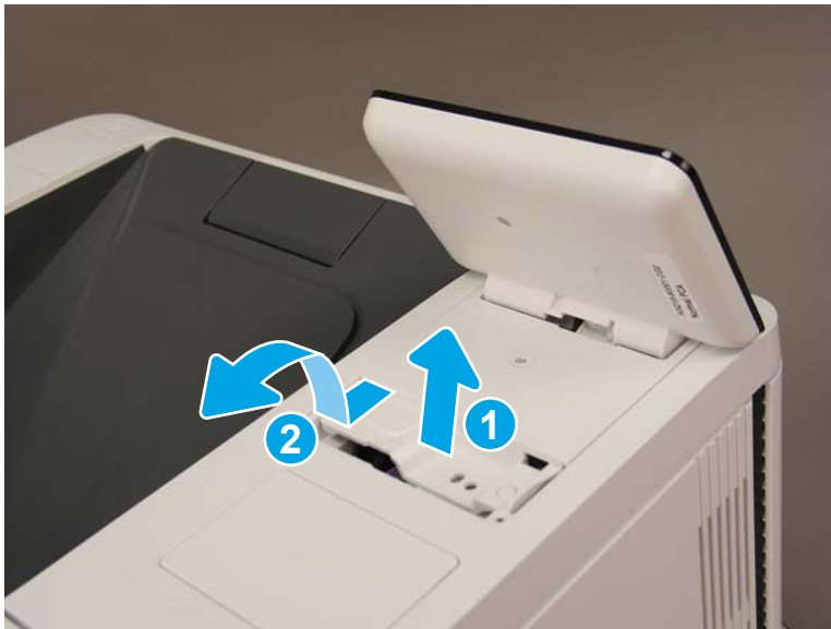
Figure 1-2344 Lift and release the control panel
