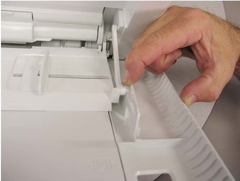
Figure 1-2086 Release the MP tray assembly lift arms from the MP cover
