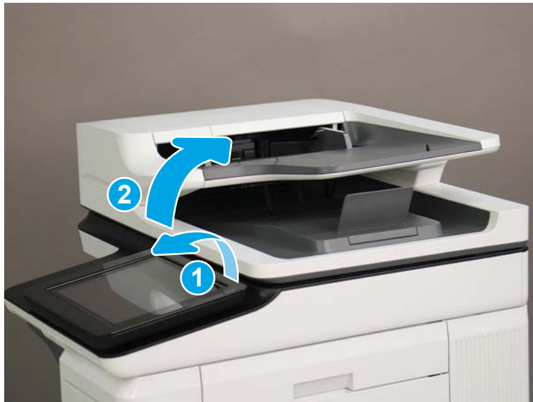
Figure 1-1058 Tilt the control panel and open the document feeder
