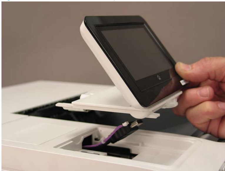
Figure 1-2596 Remove the control panel
