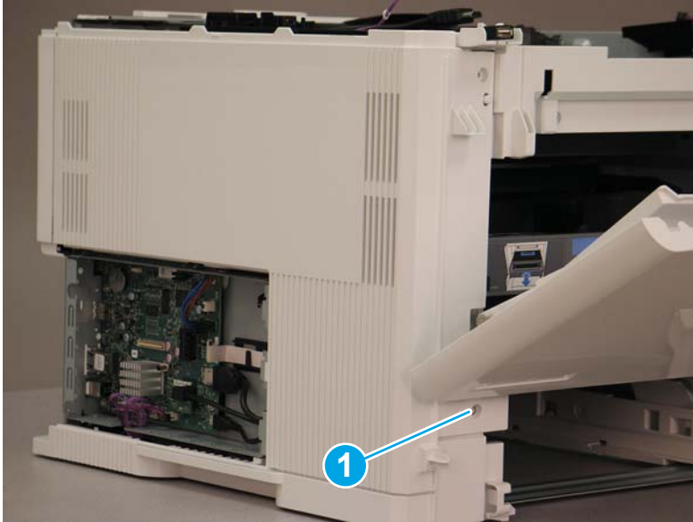
Figure 1-2331 Open the cartridge door and remove one screw
