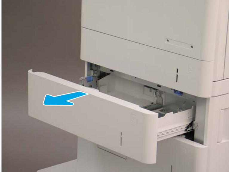
Figure 1-1975 Open the paper tray to locate the rollers
