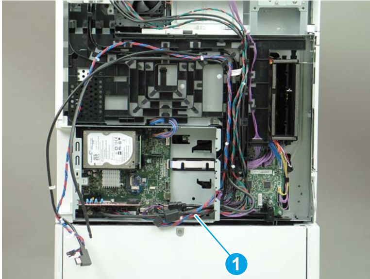
Figure 1-1030 Thread the formatter cables through the formatter case
