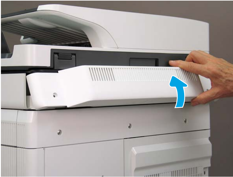
Figure 1-1013 Remove the image scanner back cover
