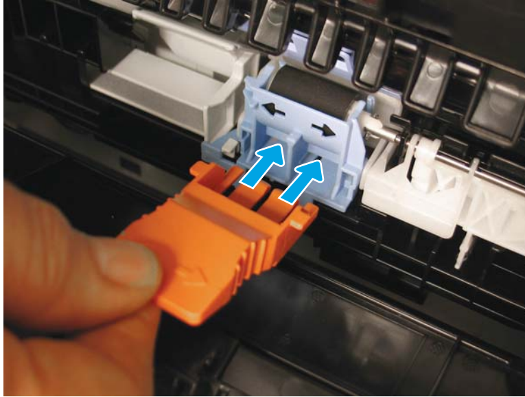
Figure 1-1984 Install the orange tool in the separation roller
