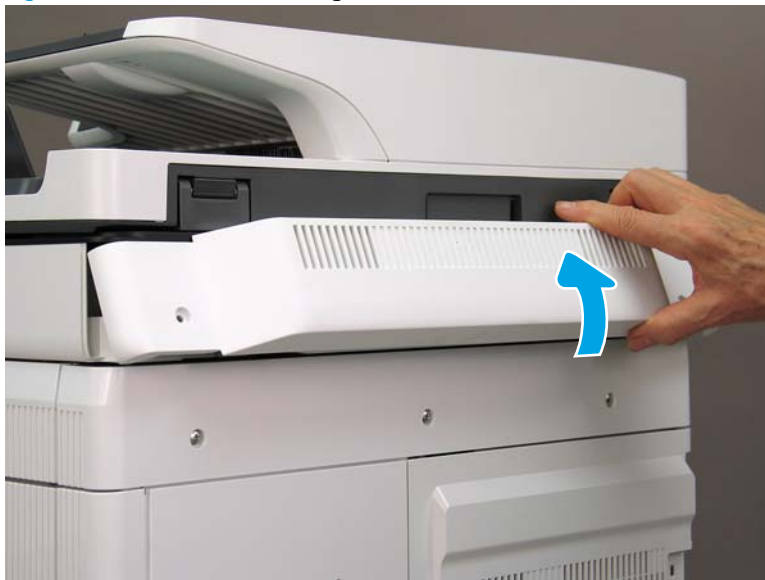
Figure 1-418 Remove the image scanner back cover
