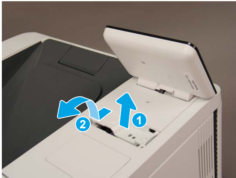
Figure 1-2234 Lift and release the control panel
