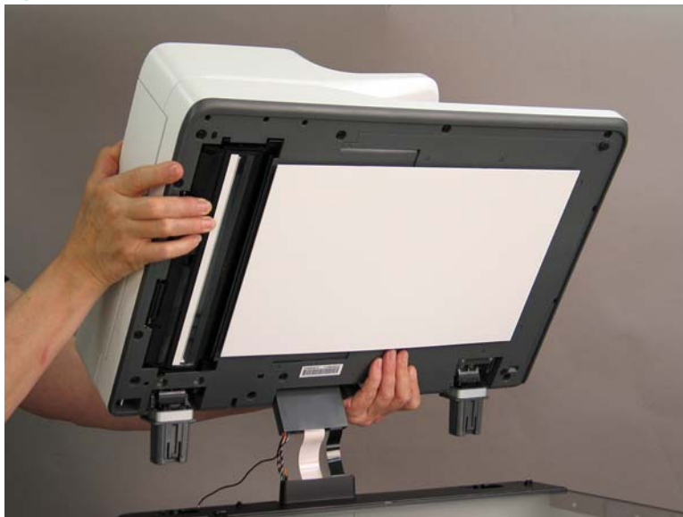
Figure 1-621 Lift and remove the ADF
