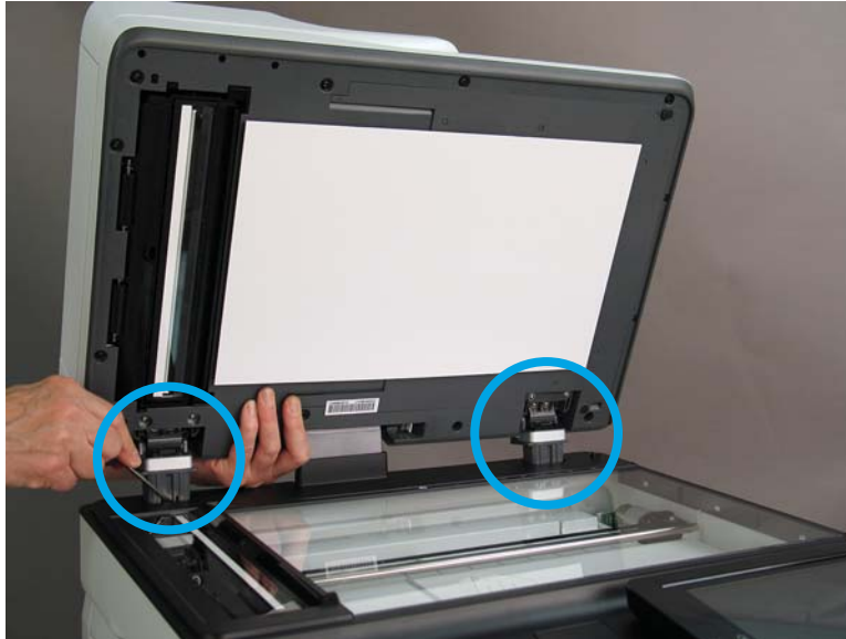
Figure 1-961 Release two tabs on the ADF
