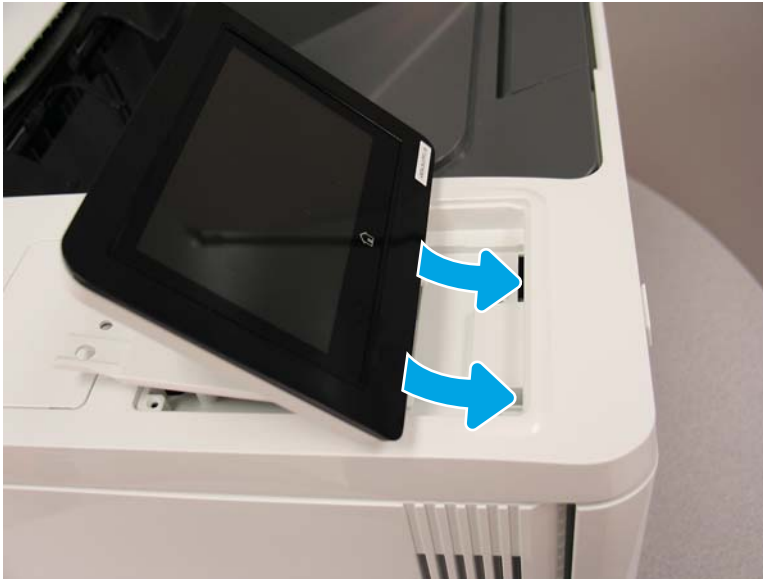
Figure 1-1907 Install the control panel tabs into the printer slots
