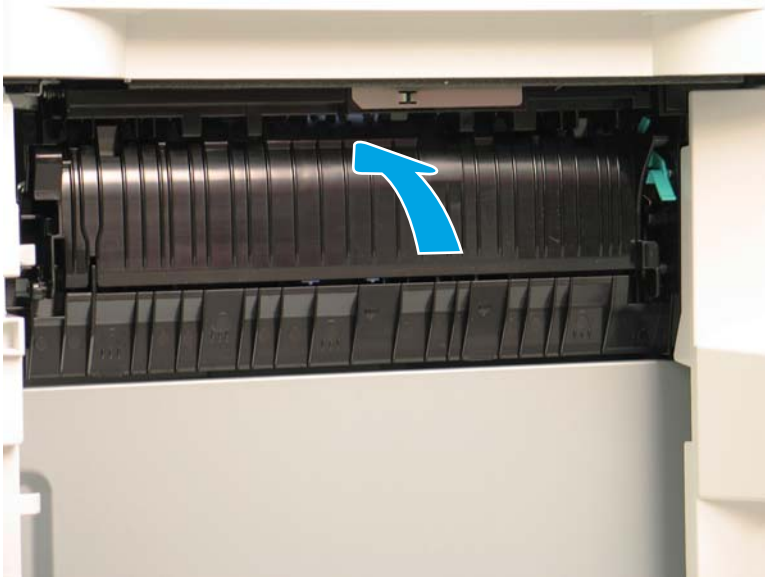
Figure 1-150 Raise the feed assembly cover
