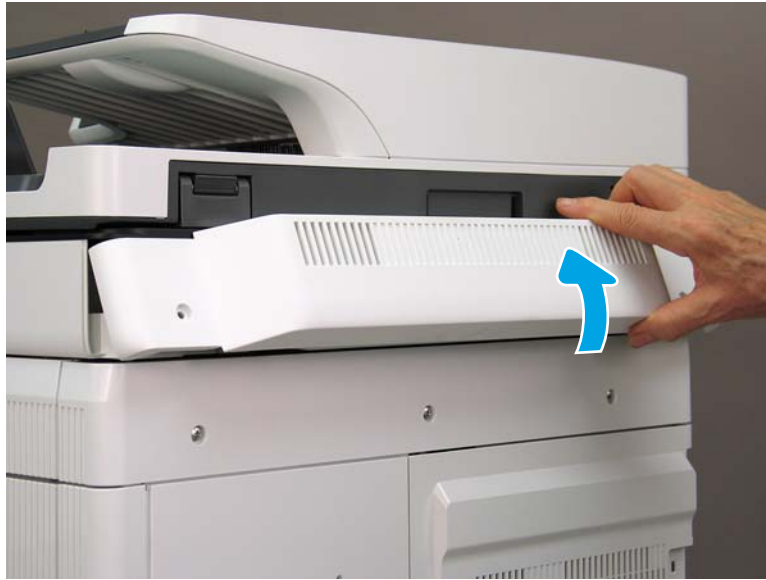
Figure 1-561 Remove the image scanner back cover
