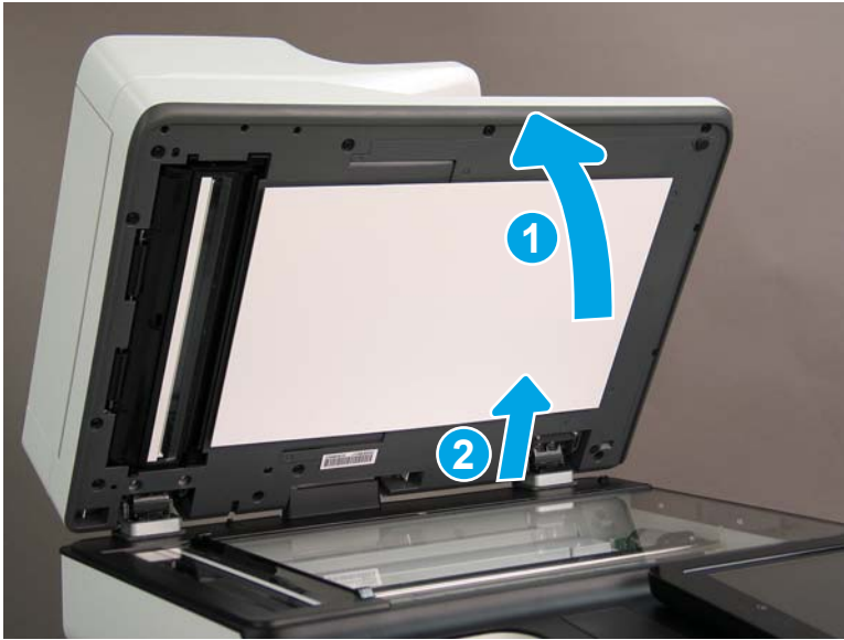
Figure 1-423 Tilt and lift the ADF
