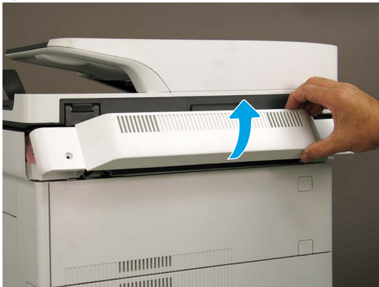
Figure 1-160 Remove the SCB cover
