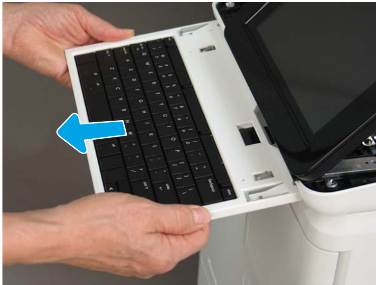
Figure 1-413 Remove the keyboard
