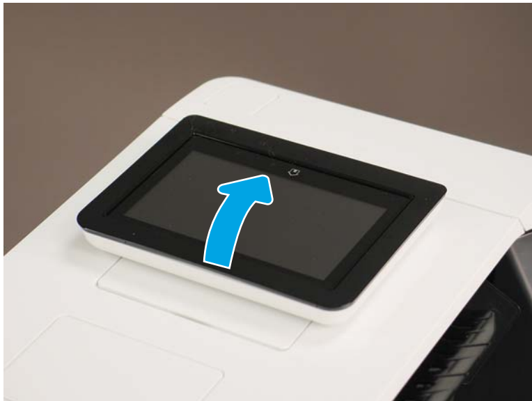
Figure 1-2679 Raise the control panel screen
