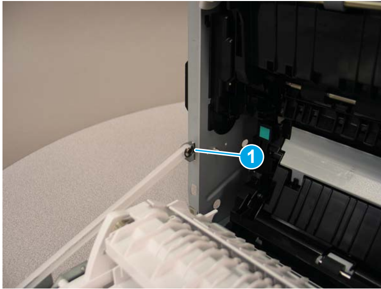
Figure 1-2484 Remove the e-ring
