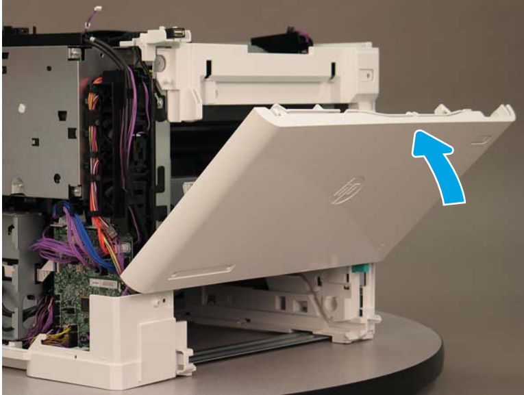
Figure 1-2525 Partially close the cartridge door
