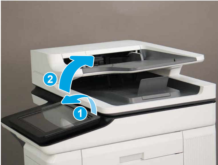
Figure 1-363 Tilt the control panel and open the document feeder
