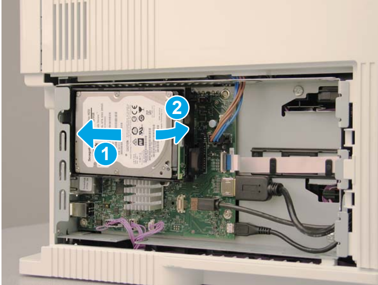
Figure 1-1961 Install the tab into the slot and rotate the connector end
