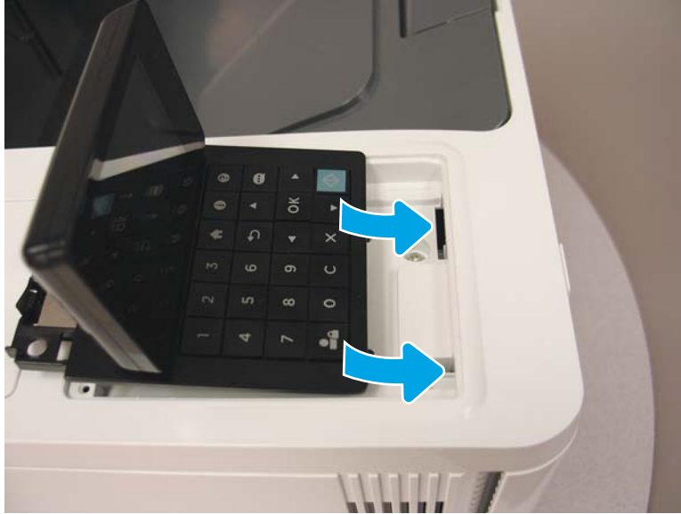
Figure 1-1917 Install the control panel tabs into the printer slots
