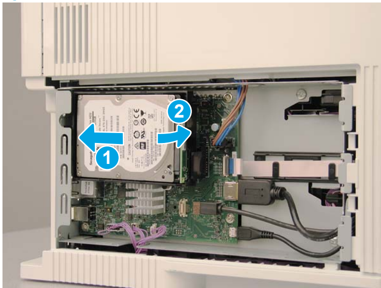
Figure 1-1946 Install the tab into the slot and rotate the connector end
