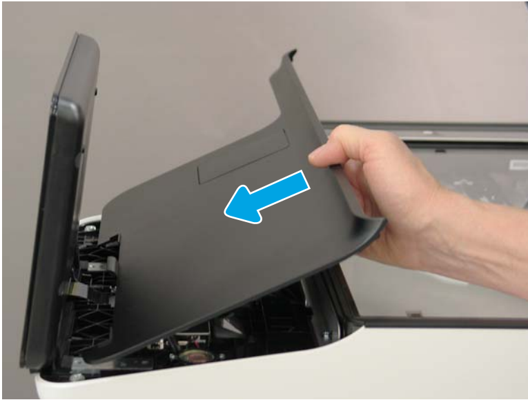
Figure 1-114 Position the cover on the printer
