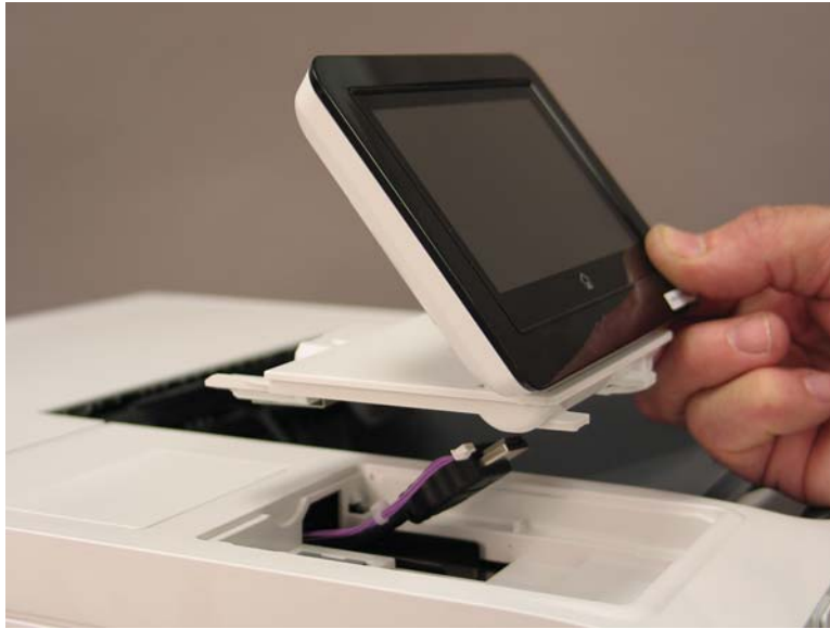
Figure 1-2183 Remove the control panel
