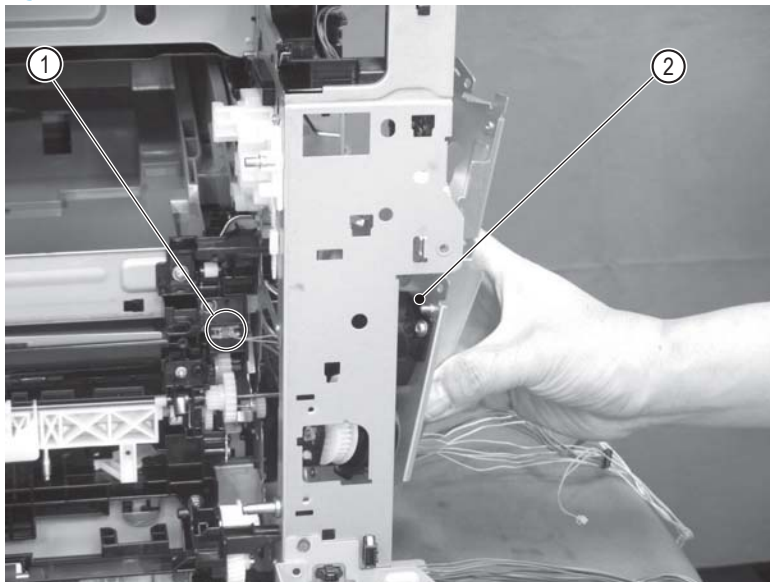
Figure 1-2517 Disconnect one connector and remove the main drive assembly
