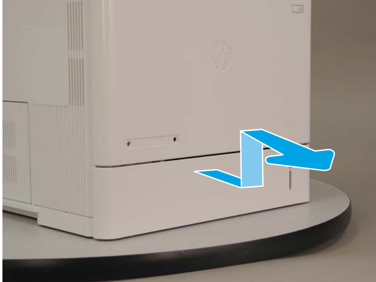
Figure 1-2673 Open and remove the cassette tray 2
