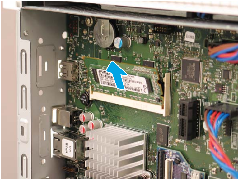
Figure 1-62 Lift up and remove the DIMM
