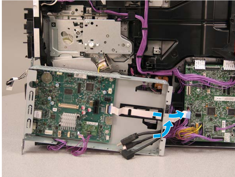
Figure 1-2453 Pull one cable and the FFC through the formatter cage
