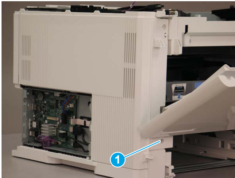
Figure 1-2017 Open the cartridge door and remove one screw
