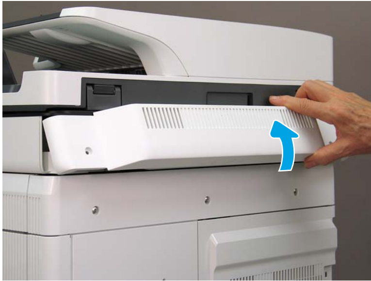
Figure 1-1195 Remove the image scanner back cover
