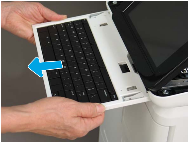
Figure 1-1121 Remove the keyboard
