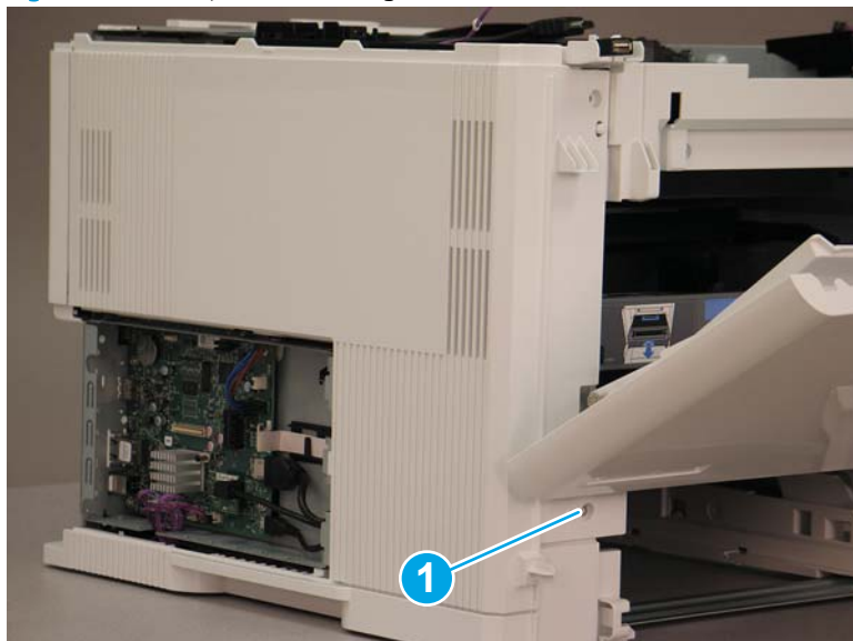
Figure 1-2666 Open the cartridge door and remove one screw
