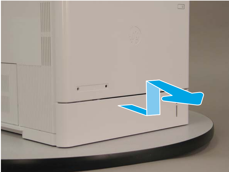
Figure 1-2693 Open and remove the cassette tray 2
