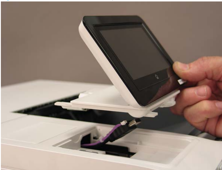
Figure 1-2388 Remove the control panel
