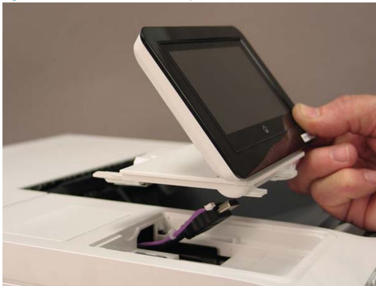
Figure 1-2346 Remove the control panel
