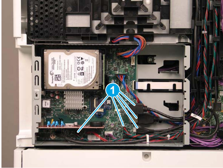
Figure 1-1211 Disconnect connect five connectors
