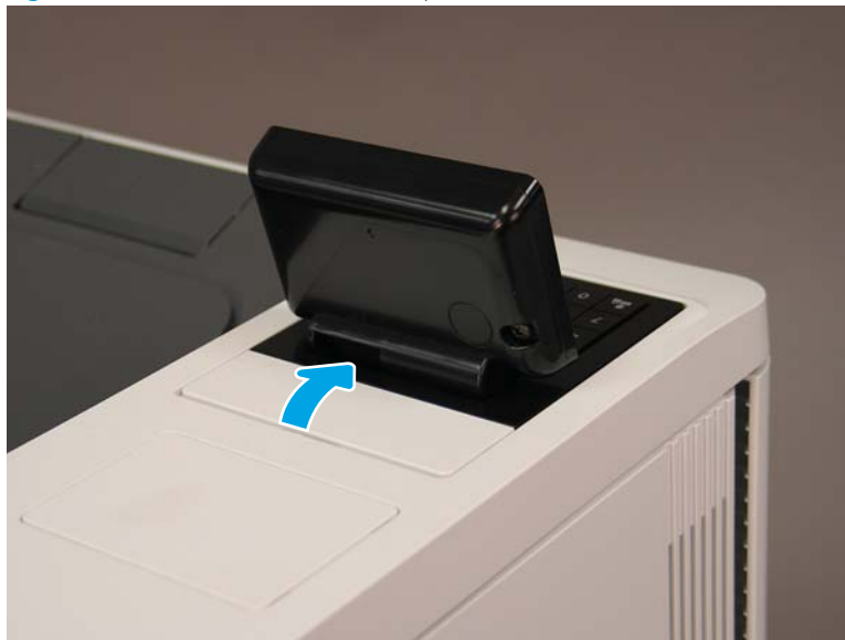
Figure 1-1911 Release the control panel cover and remove it
