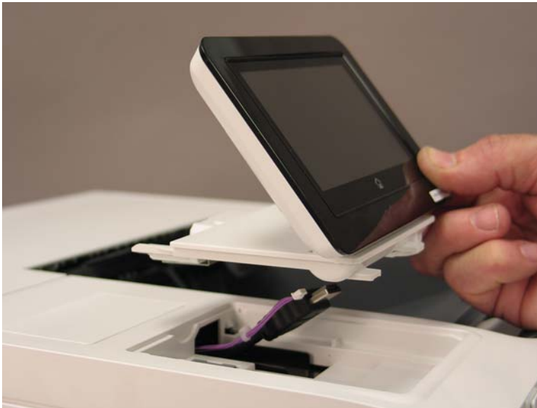
Figure 1-1905 Remove the control panel
