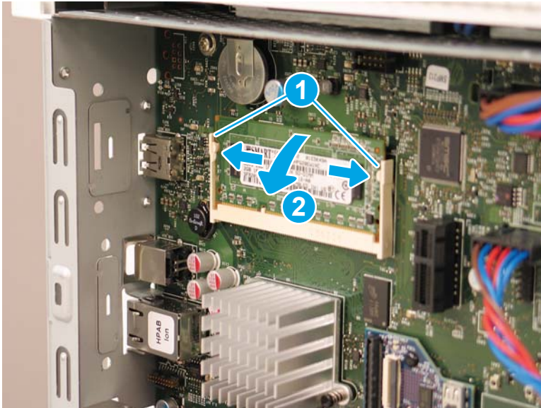
Figure 1-61 Release two locking arms and pivot the DIMM away from the holder
