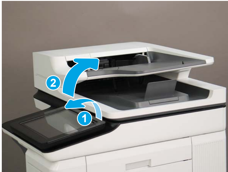
Figure 1-1184 Tilt the control panel and open the document feeder
