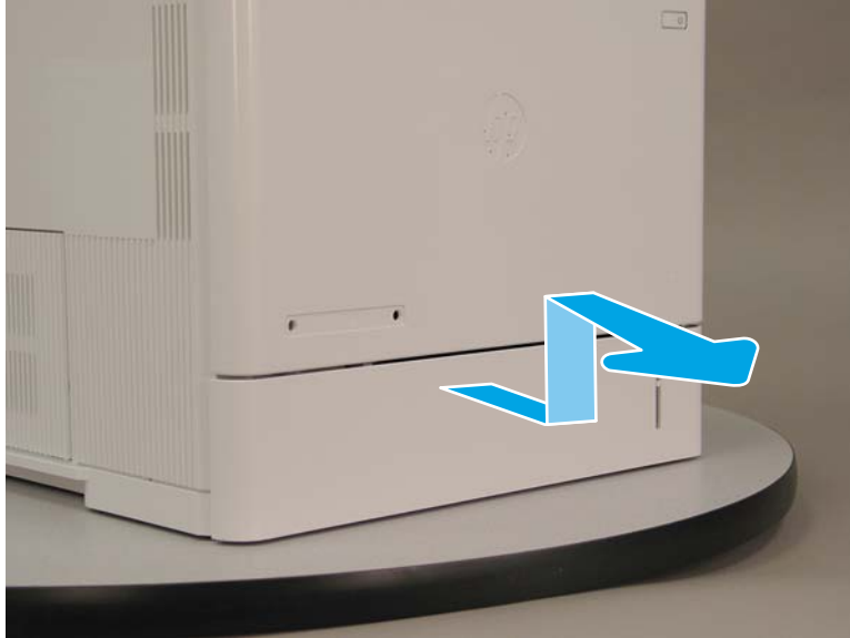
Figure 1-2417 Open and remove the cassette tray 2
