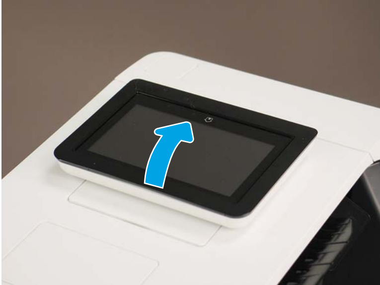
Figure 1-2032 Raise the control panel screen
