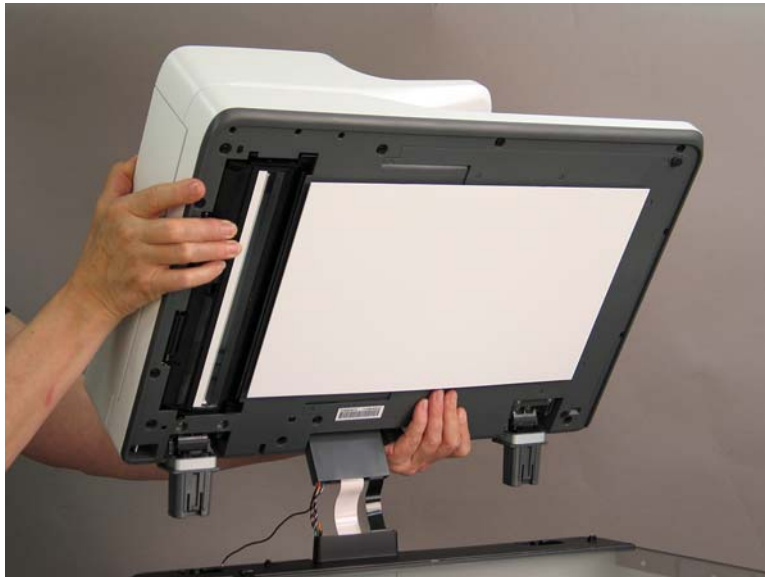
Figure 1-1020 Lift and remove the ADF
