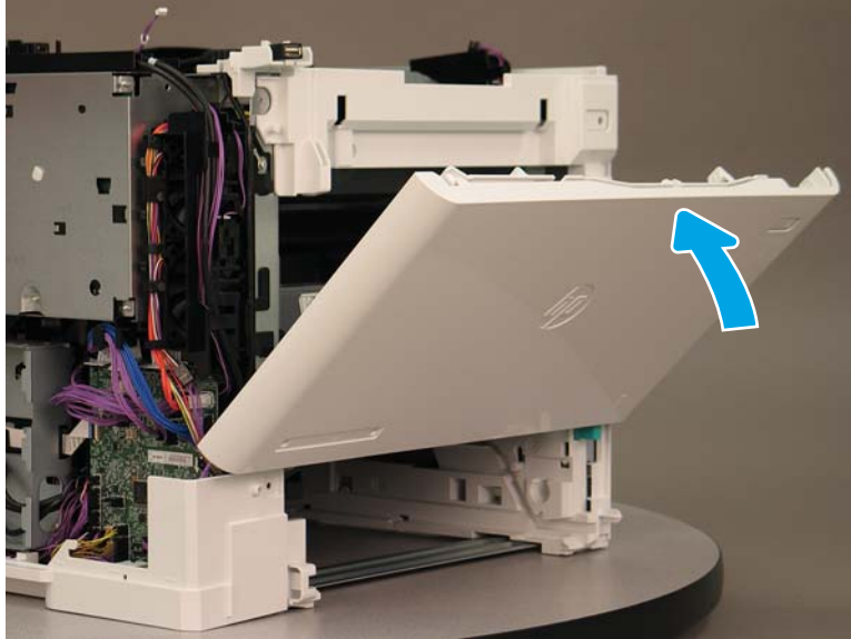
Figure 1-2274 Partially close the cartridge door
