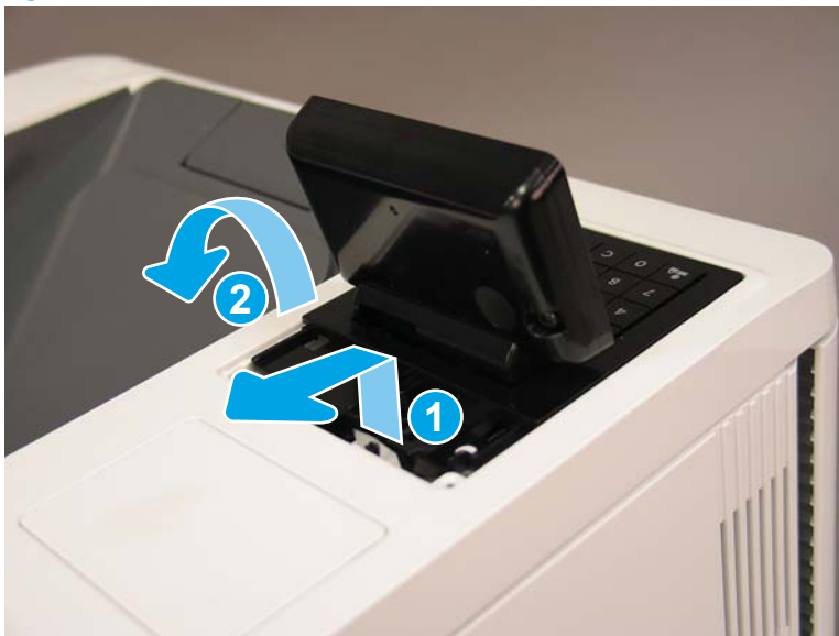
Figure 1-1913 Release the control panel and turn it over
