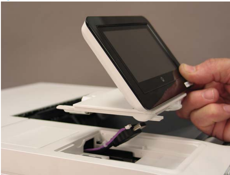
Figure 1-2236 Remove the control panel
