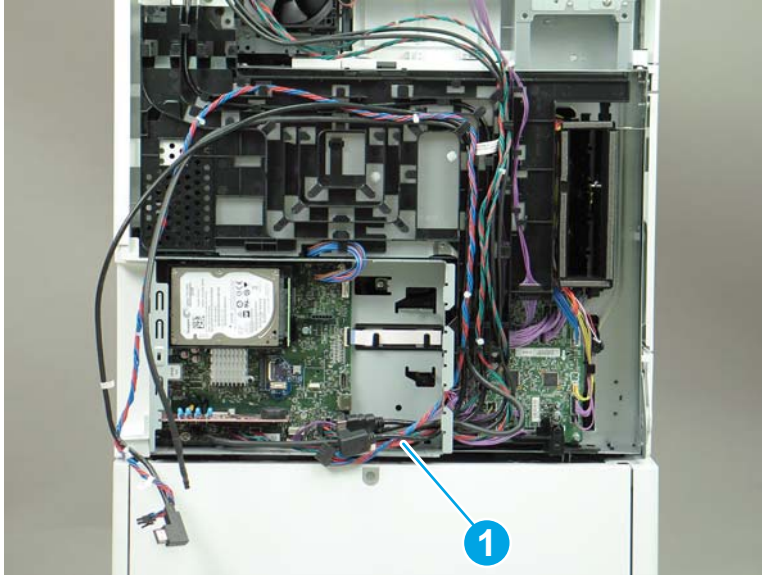
Figure 1-295 Thread the formatter cables through the formatter case
