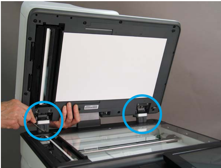
Figure 1-1132 Release two tabs on the ADF
