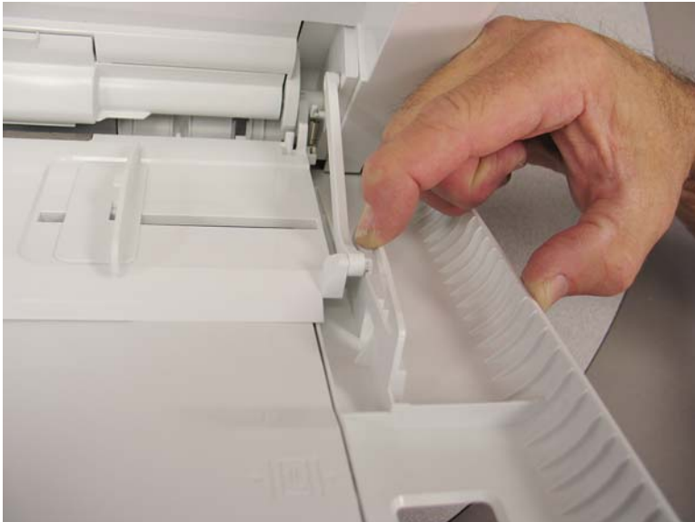
Figure 1-2651 Release the MP tray assembly lift arms from the MP cover
