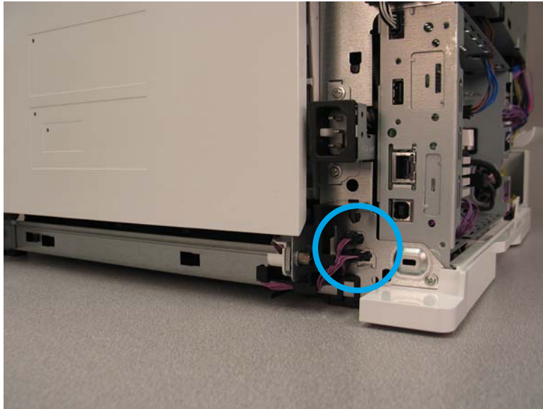
Figure 1-2137 Disconnect two connectors
