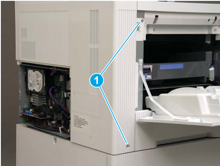
Figure 1-708 Remove two screws
