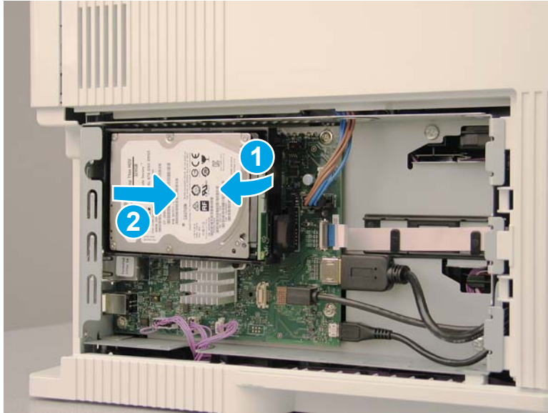
Figure 1-1956 Rotate the HDD away from the formatter and remove the HDD
