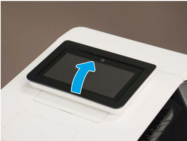
Figure 1-2107 Raise the control panel screen
