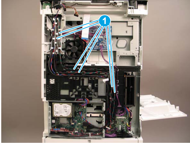
Figure 1-389 Release the formatter cables
