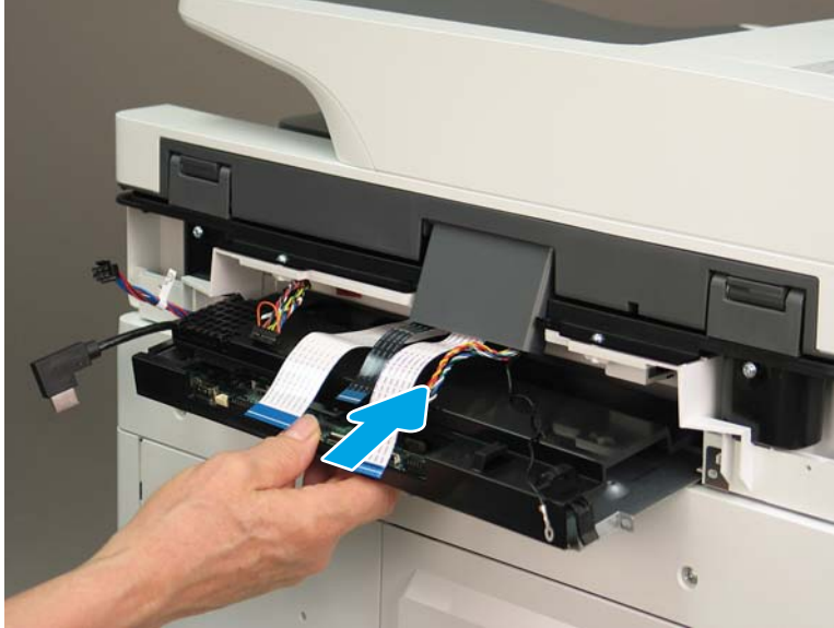
Figure 1-686 Check the cables when installing the SCB
