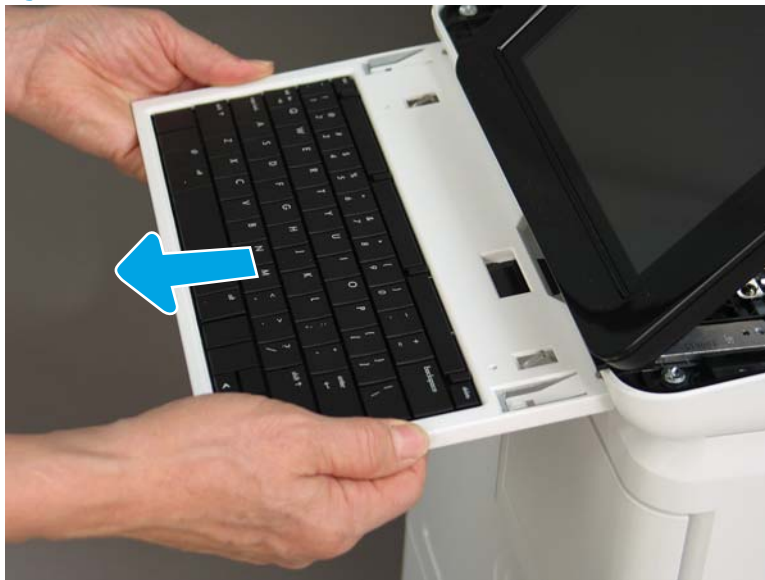
Figure 1-1008 Remove the keyboard
