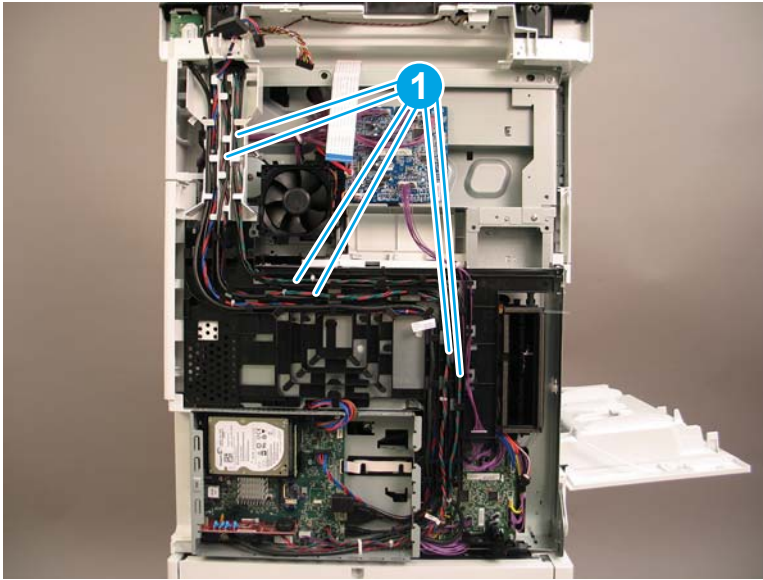
Figure 1-1395 Release the formatter cables
