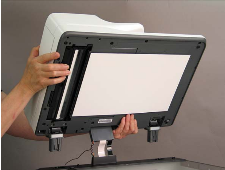
Figure 1-677 Lift and remove the ADF
