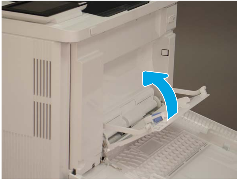
Figure 1-2652 Close the smaller MP tray assembly
