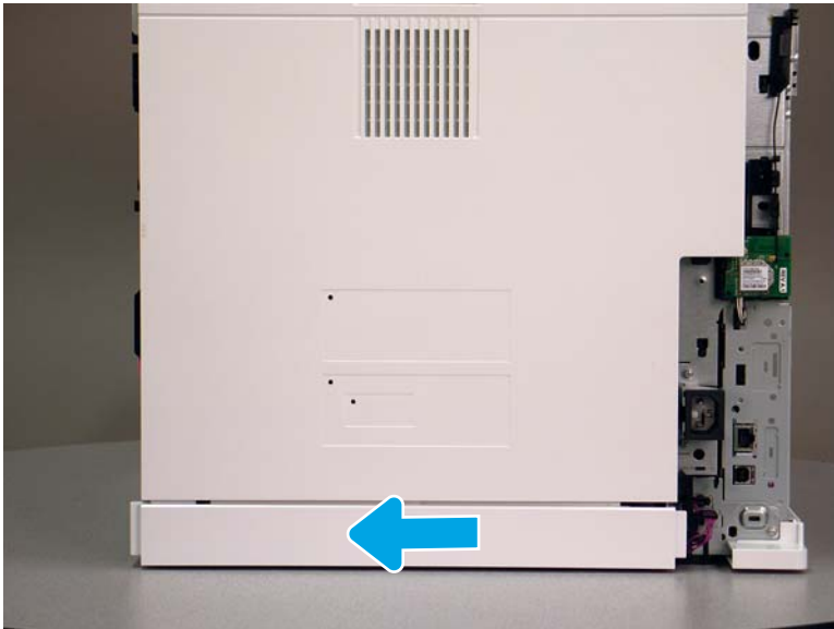
Figure 1-2152 Slide the rear lower cover
