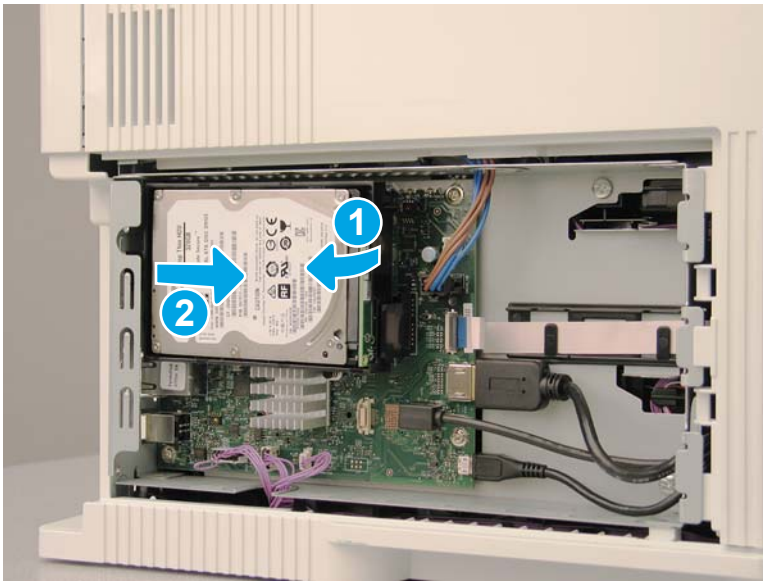
Figure 1-1944 Rotate the HDD away from the formatter and remove the HDD
