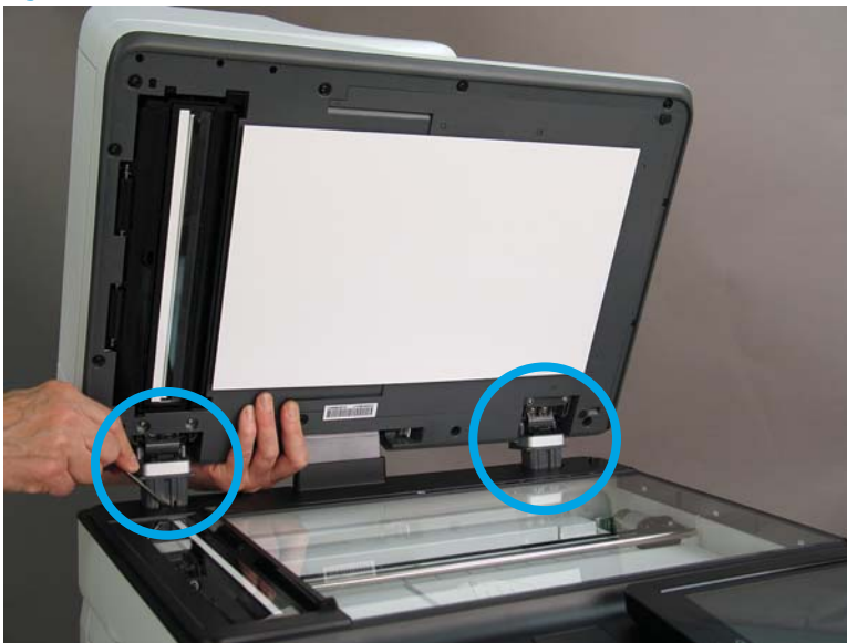
Figure 1-424 Release two tabs on the ADF
