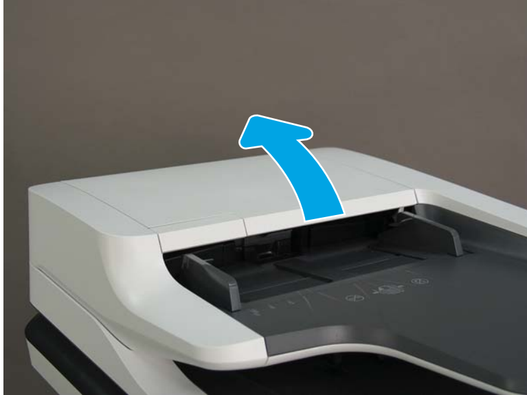
Figure 1-24 Open the document feeder cover
