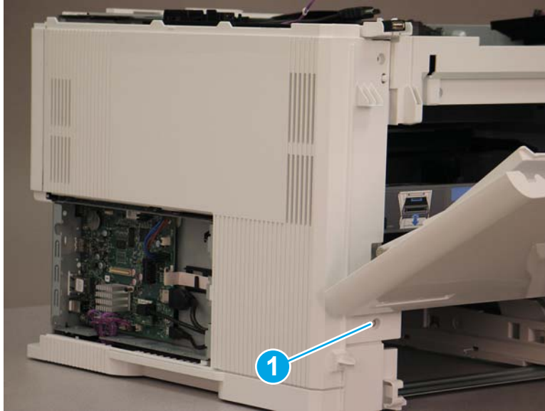
Figure 1-2270 Open the cartridge door and remove one screw
