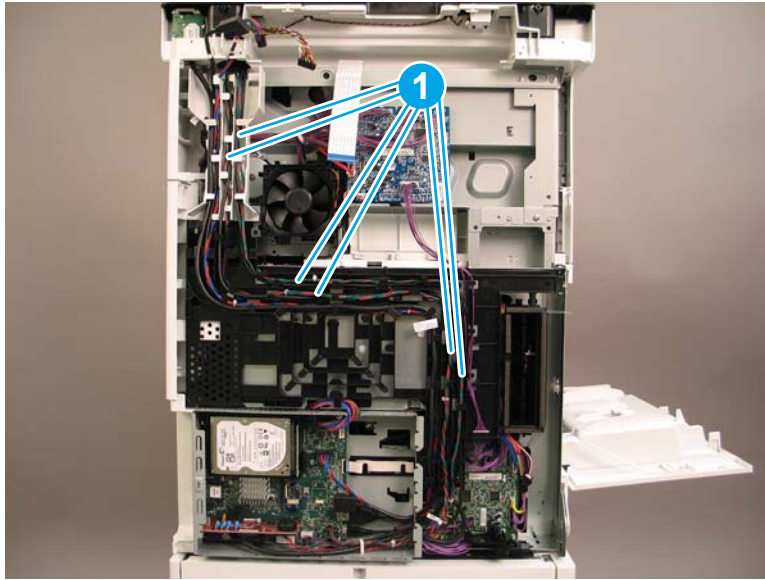
Figure 1-433 Release the formatter cables
