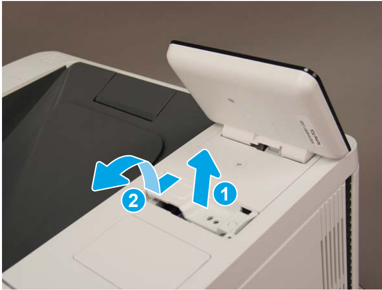
Figure 1-2462 Lift and release the control panel
