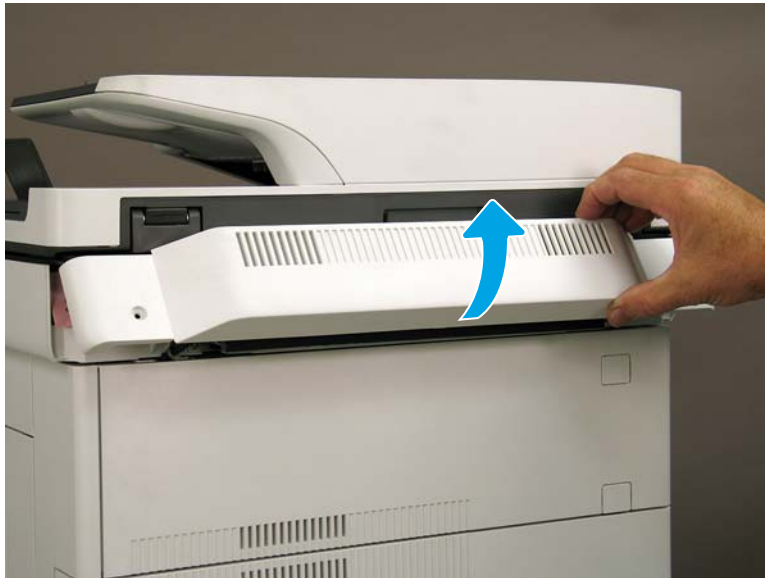
Figure 1-681 Remove the SCB cover
