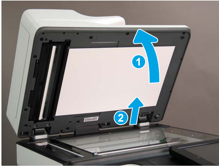
Figure 1-1385 Tilt and lift the ADF
