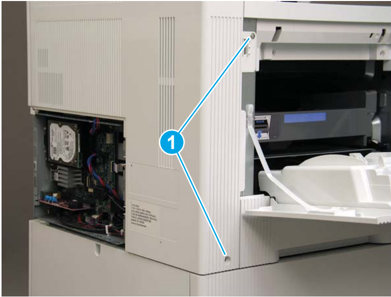
Figure 1-174 Remove two screws
