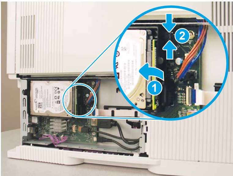
Figure 1-1955 Release the locking connector and release the HDD retainer
