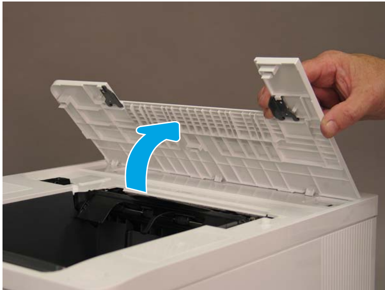
Figure 1-2039 Rotate the blanking cover up
