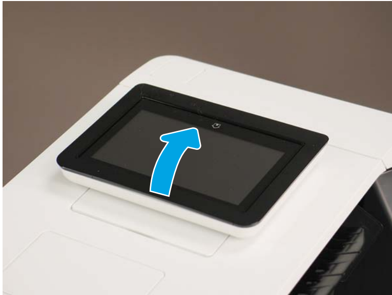
Figure 1-2418 Raise the control panel screen
