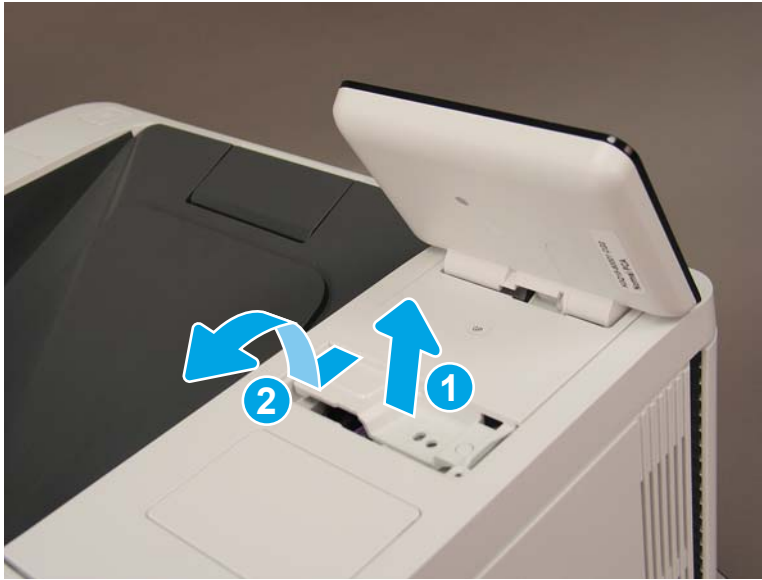
Figure 1-2181 Lift and release the control panel
