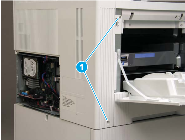
Figure 1-1421 Remove two screws
