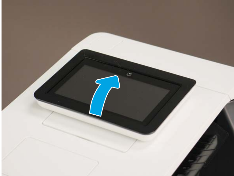
Figure 1-2341 Raise the control panel screen
