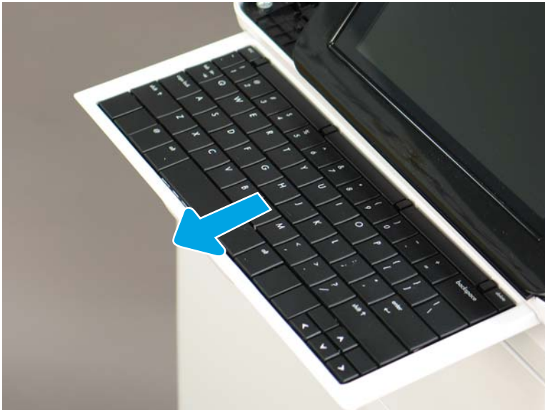
Figure 1-787 Slide the keyboard tray out
