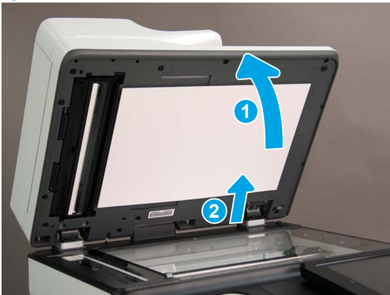
Figure 1-738 Tilt and lift the ADF
