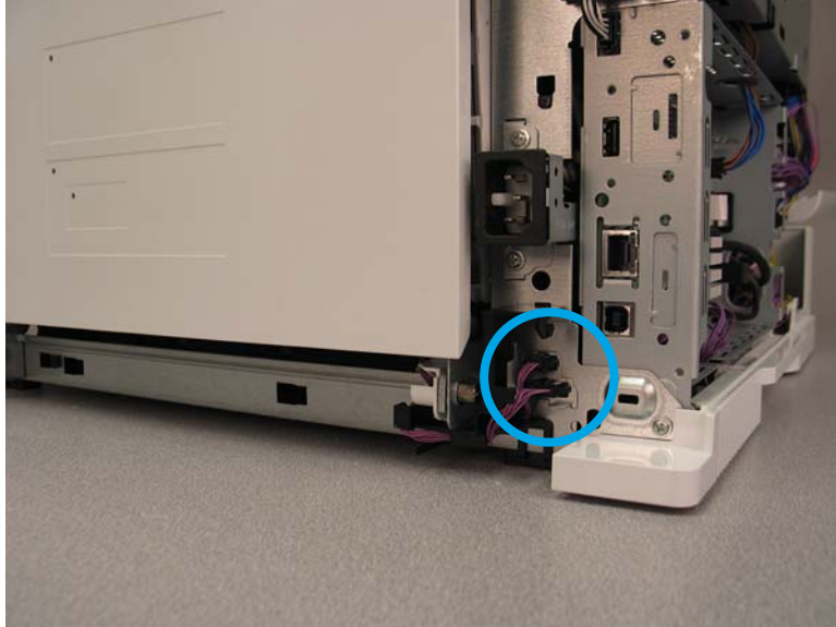
Figure 1-2480 Disconnect two connectors
