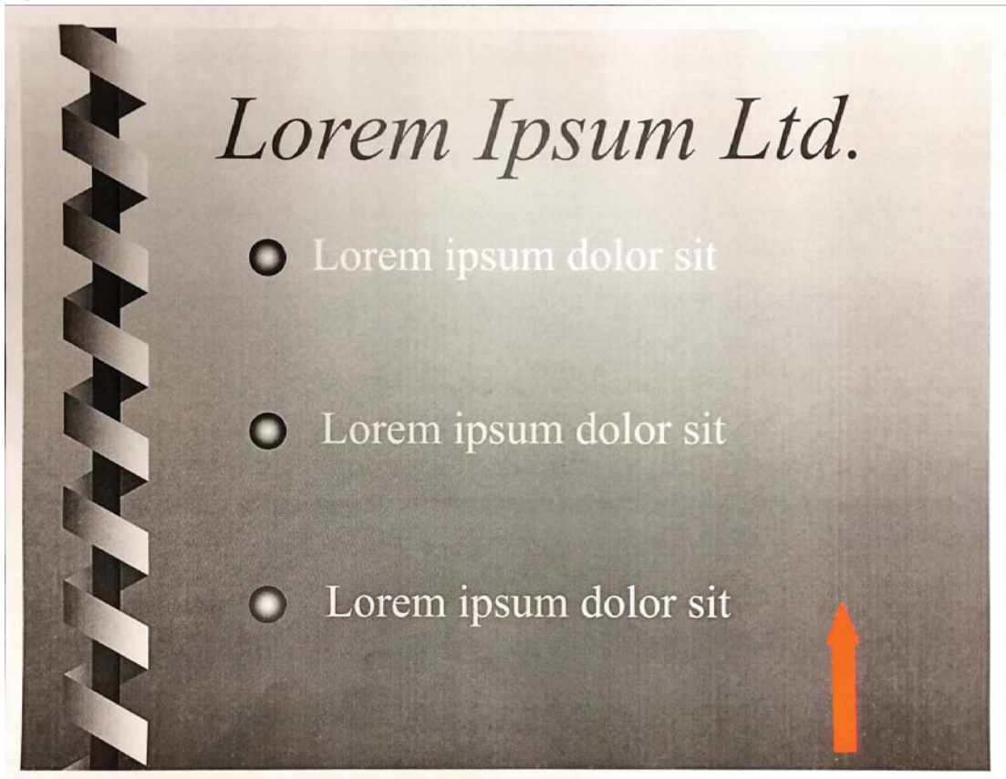
Figure 2-116 46 mm leading edge blur
