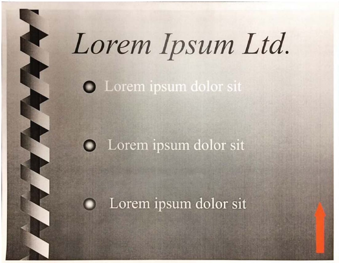
Figure 2-115 18 mm leading edge blur
