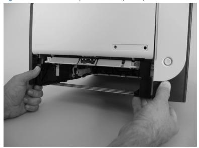
2. Release the two roller-cover locking pins, and then remove the cover.
