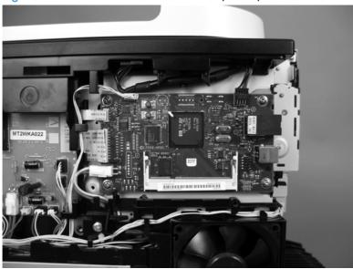
3. Remove four screws (callout 1), and then remove the formatter PCA.
