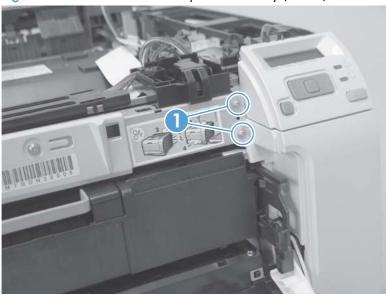
3. Remove the control-panel assembly.
