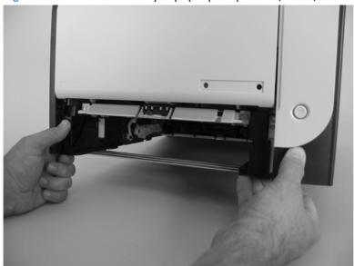
4. Release two tabs, and then rotate the roller away from the product to remove it.
