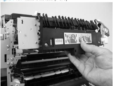
8. **Duplex models only**: Remove two screws (callout 1) and remove the duplex-gear assembly (callout 2). Install the assembly on the replacement fuser.
