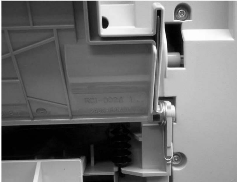
Figure 6-80 Correct tray 1 rear-hinge-spring placement
