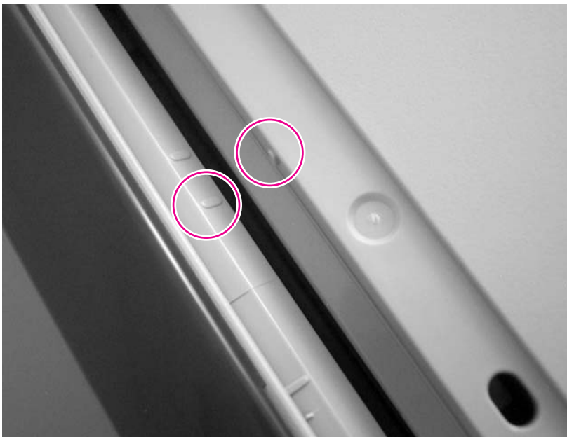
Figure 6-180 Correctly positioning the scanner assembly
