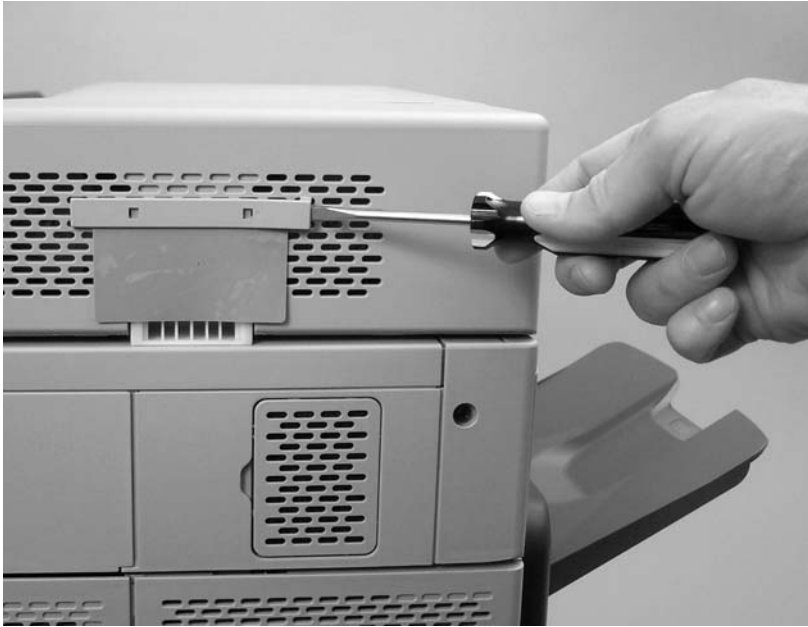
Figure 6-27 Remove the ADF-hinge flap (1 of 3)
