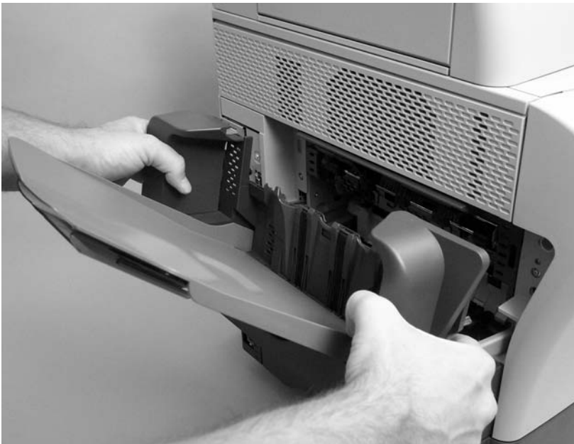
Figure 6-17 Remove the output-bin assembly (2 of 2)
