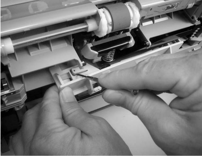
Figure 6-82 Remove the front-cover support (1 of 2)
