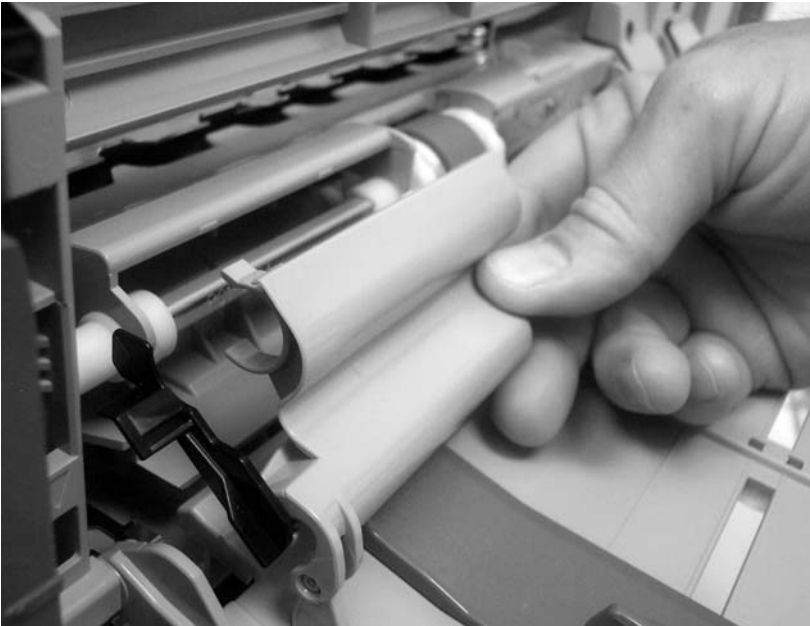
Figure 6-78 Remove the tray 1 assembly (3 of 5)
