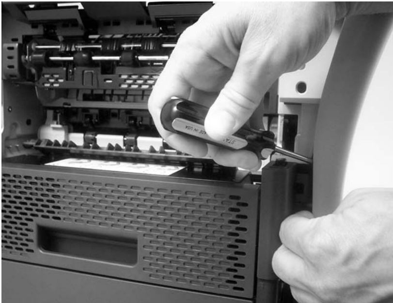
Figure 6-43 Remove the front cover (4 of 7)
