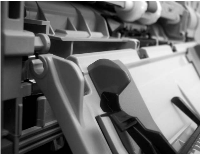
Figure 6-79 Remove the tray 1 assembly (4 of 5)
