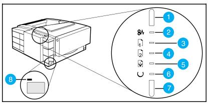
Figure 5 5P/5MP Status Panel Buttons and Lights
