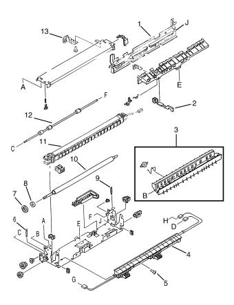
Figure 36. HP LaserJet 5P Fusing Assembly
