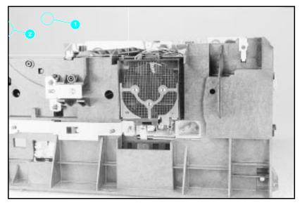
Figure 28 Grounding Spring screw location.
