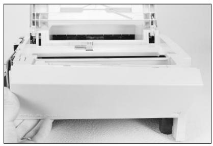
Figure 21 Removing Tray 1.
