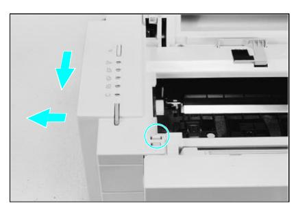
Figure 14 Left Side Cover Release Latch
