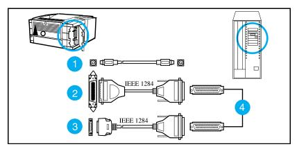
Figure 11 HP LaserJet 5P/5MP Printer Interface Connections
