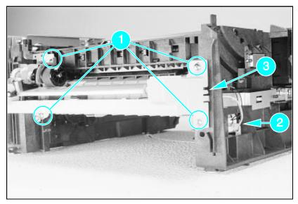
Figure 19 Tray 1 Pickup Assembly Locations.
