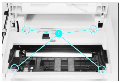
Figure 15 Removing the Top Cover Screws
