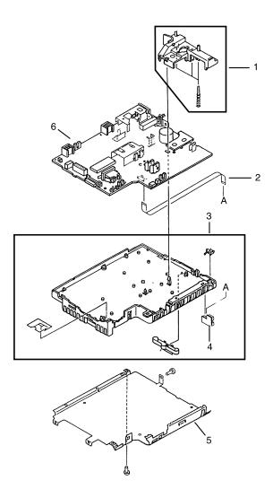
Figure 33. DC Controller Assembly
