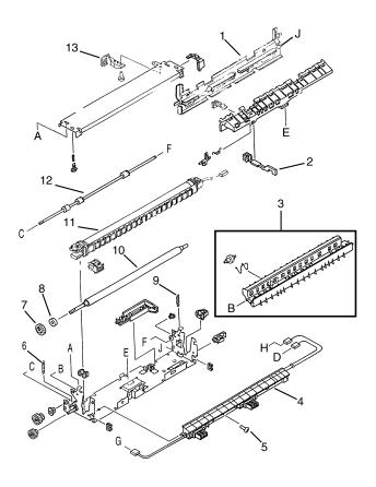
Figure 39. HP LaserJet 5P/6P Fusing Assembly
