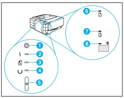
Figure 6 6P/6MP Status Panel Buttons and Lights
