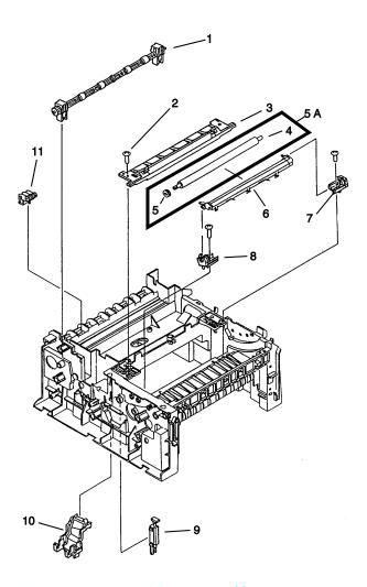
Figure 31. HP LaserJet 5P Internal Components (2)
