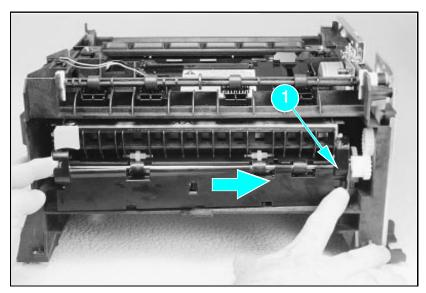
Figure 24 Removing the fuser cover.
