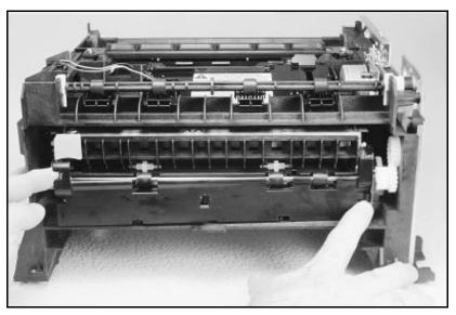
Figure 27 Removing the fuser cover.
