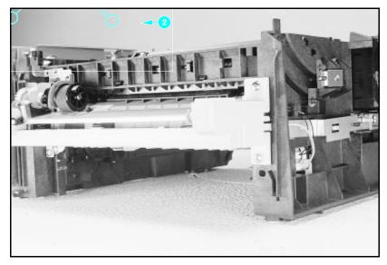
Figure 22 Tray 1 Pickup Assembly Locations.
