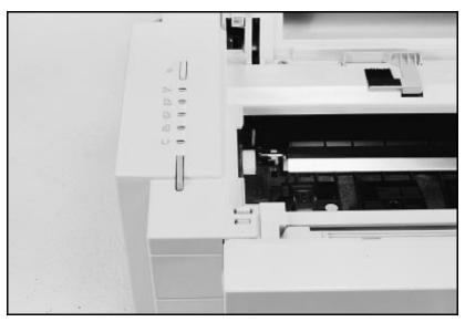
Figure 17 Left Side Cover Release Latch (5P/5MP shown)
