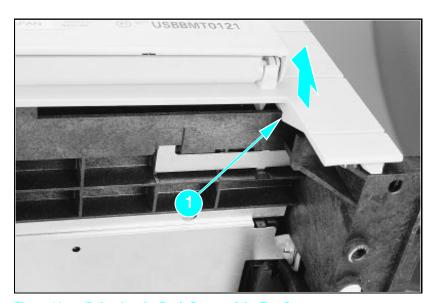
Figure 16 Releasing the Back Corner of the Top Cover.
