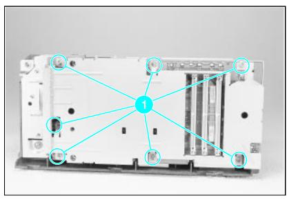
Figure 22 Removing the formatter screws.
