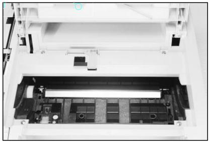
Figure 18 Removing the Top Cover Screws
