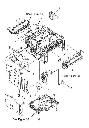
Figure 33. HP LaserJet 5P/6P Internal Components (1)
