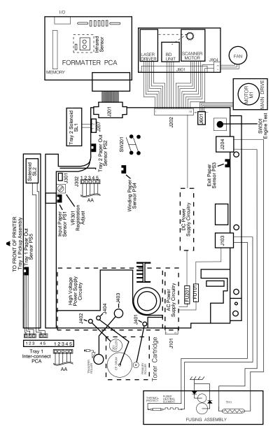
Figure 31 Main Wiring Diagram
