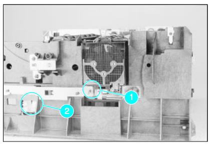
Figure 25 Grounding Spring screw location.
