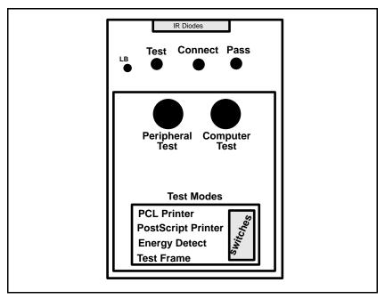
Figure 11 Infrared Test Tool
