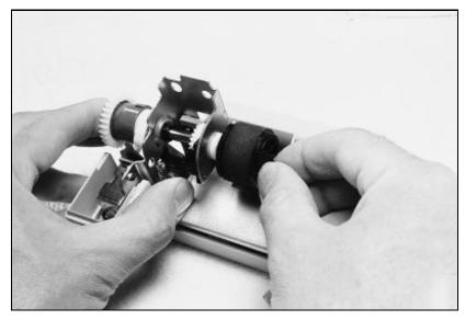
Figure 23 Replacing the Pickup Roller
