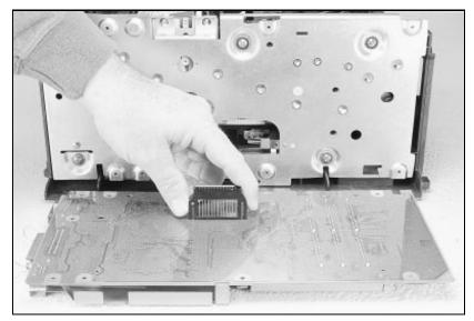
Figure 26 Removing the DC Controller Interconnect.
