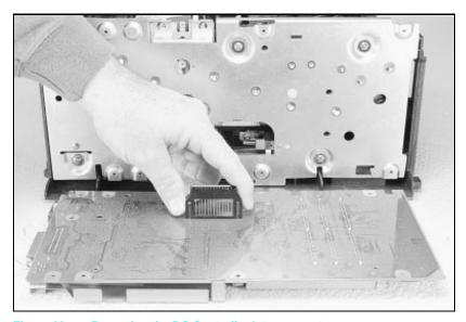
Figure 23 Removing the DC Controller Interconnect.
