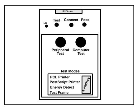
Figure 10 Infrared Test Tool
