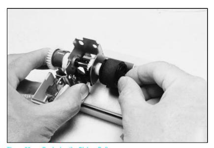
Figure 20 Replacing the Pickup Roller
