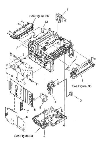
Figure 30. HP LaserJet 5P Internal Components (1)
