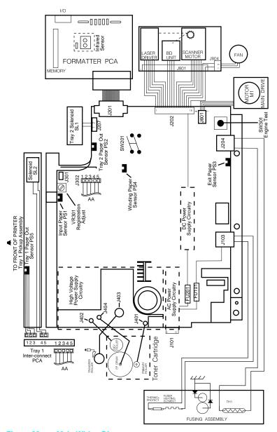
Figure 28 Main Wiring Diagram
