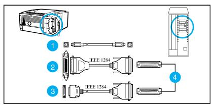
Figure 12 HP LaserJet 5P/5MP, 6P/6MP Printer Interface Connections
