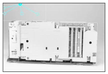
Figure 25 Removing the formatter screws.
