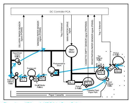
Figure 6 HP LaserJet 5P Printer Paper Path
