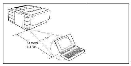
Figure 10 IRDA Port ranges (5P/5MP shown)
