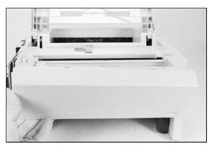
Figure 18 Removing Tray 1.
