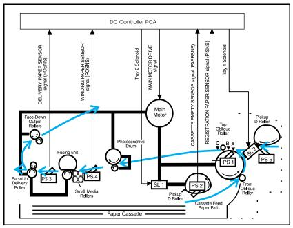
Figure 7 HP LaserJet 5P/6P Printer Paper Path
