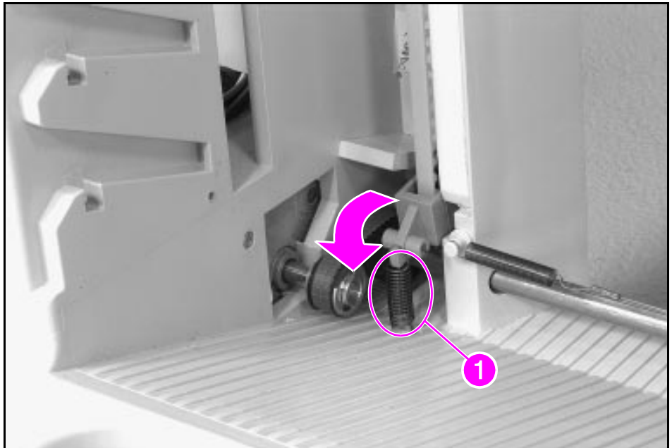
Multi-Bin Mailbox/Mailbox with Stapler, Elevator Pulley Tension Spring
