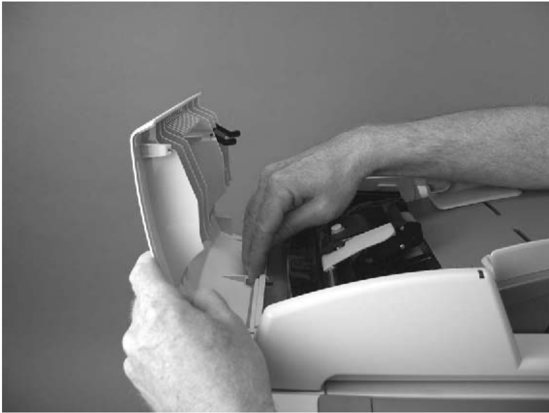
Figure 5-3 Reinstalling the ADF cover
