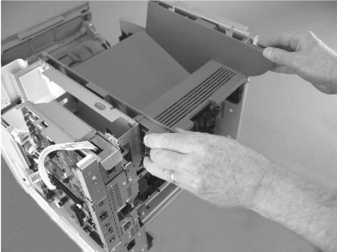
Figure 5-27 Removing the top cover (2 of 3)
