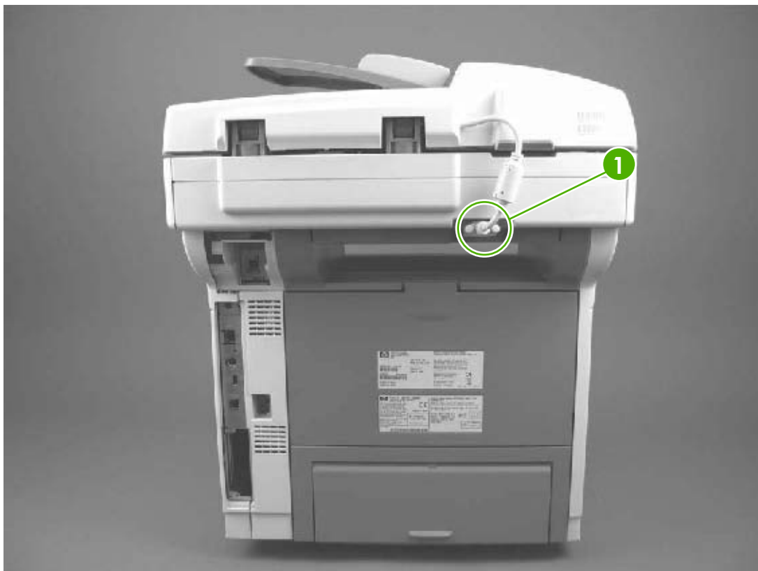
Figure 5-9 Removing the ADF (1 of 3)
