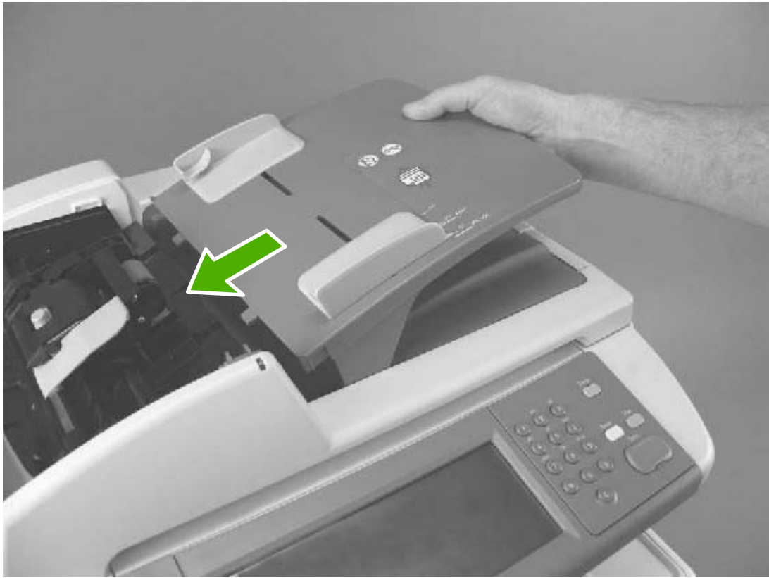
Figure 5-5 Reinstalling the ADF input tray
