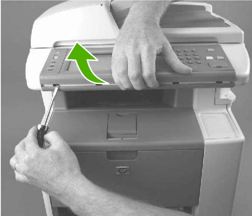
Figure 5-6 Removing the control panel (1 of 2)
