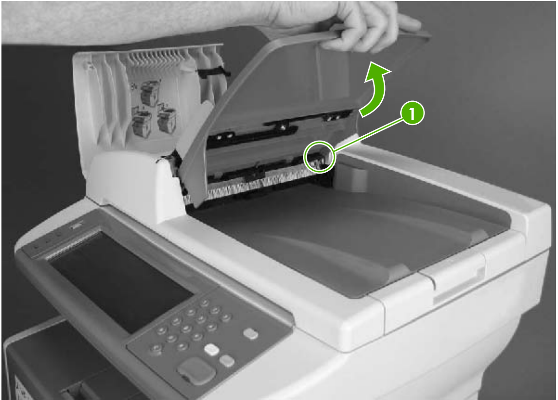
Figure 5-4 Removing the ADF input tray
