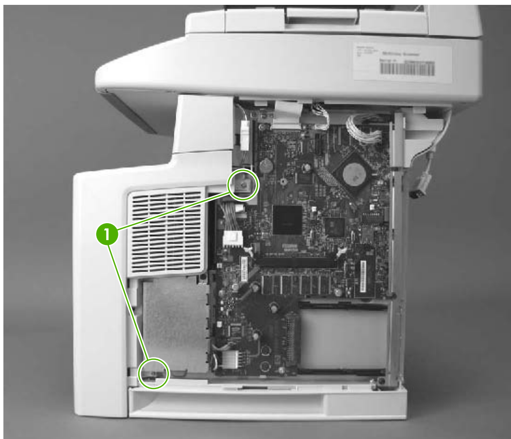
Figure 5-30 Removing the front, right cover (1 of 2)
