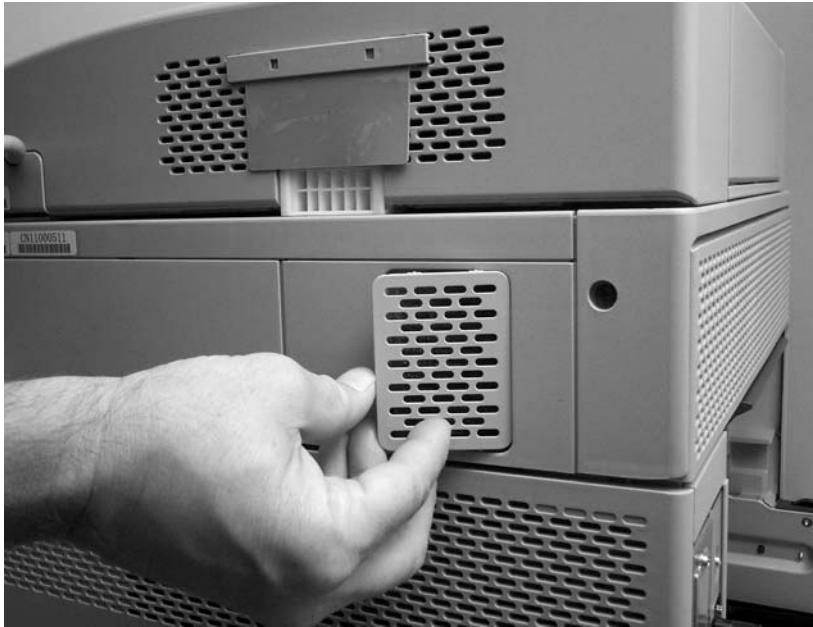
Figure 5-25 Remove the scanner filter (1 of 2)
