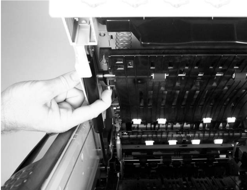
Figure 5-49 Remove the reversing-separation-guide assembly (1 of 2)
