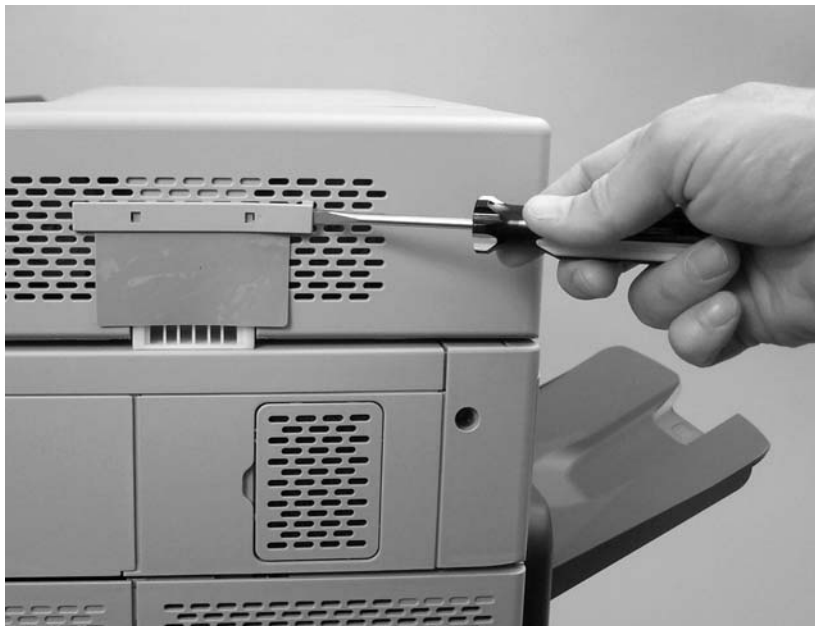
Figure 5-27 Remove the ADF-hinge flap (1 of 3)
