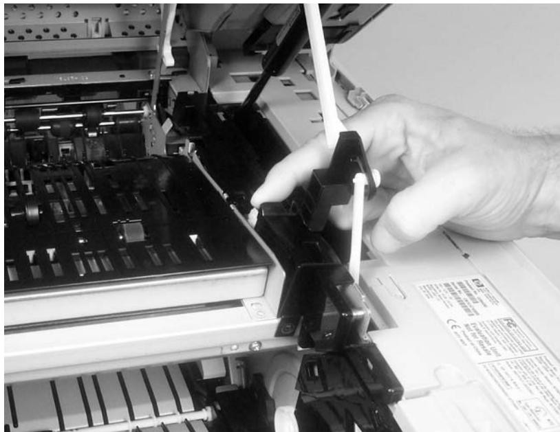
Figure 5-52 Remove the reversing assembly (2 of 8)
