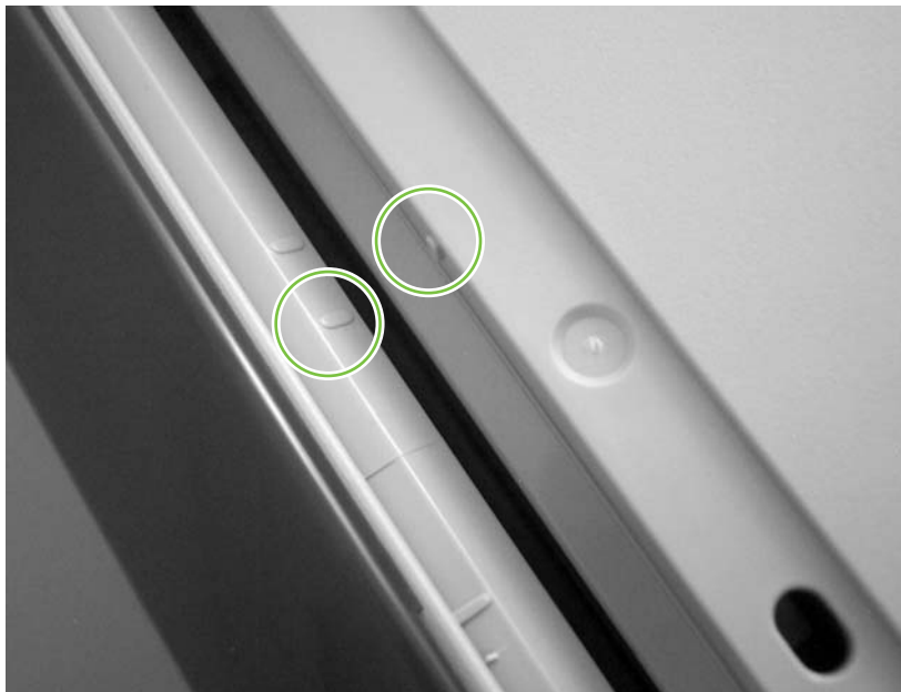
Figure 5-179 Correctly positioning the scanner assembly
