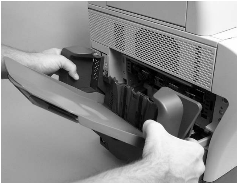
Figure 5-17 Remove the output-bin assembly (2 of 2)
