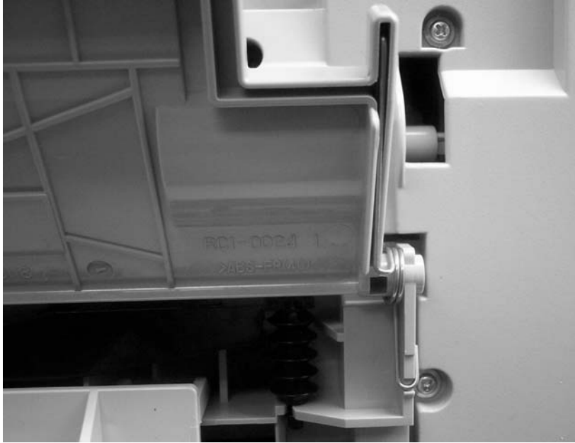
Figure 5-79 Correct tray 1 rear-hinge-spring placement
