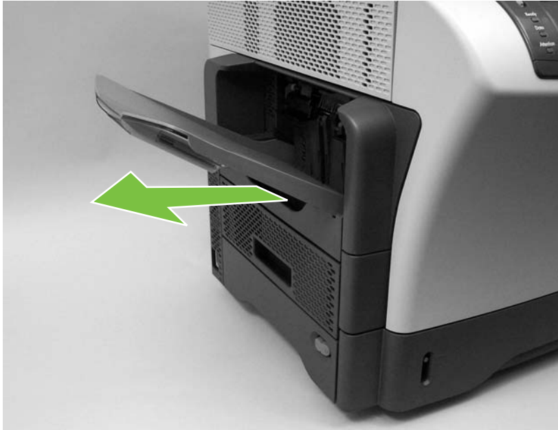
Figure 5-16 Remove the output-bin assembly (1 of 2)
