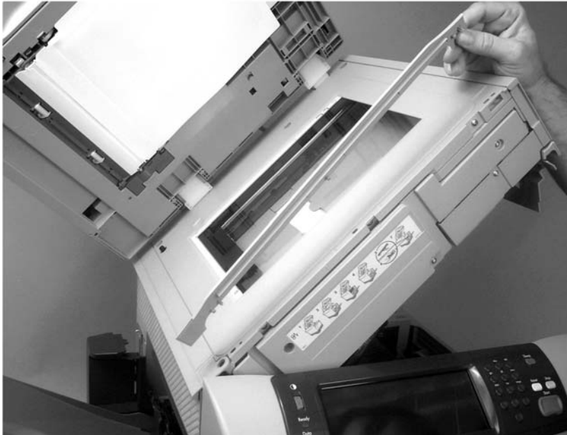
Figure 5-38 Remove the top-cover flatbed flange (2 of 2)
