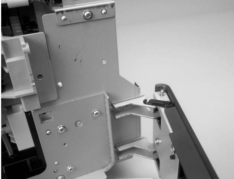
Figure 5-83 Remove the tray 1 feed-assembly (1 of 13)
