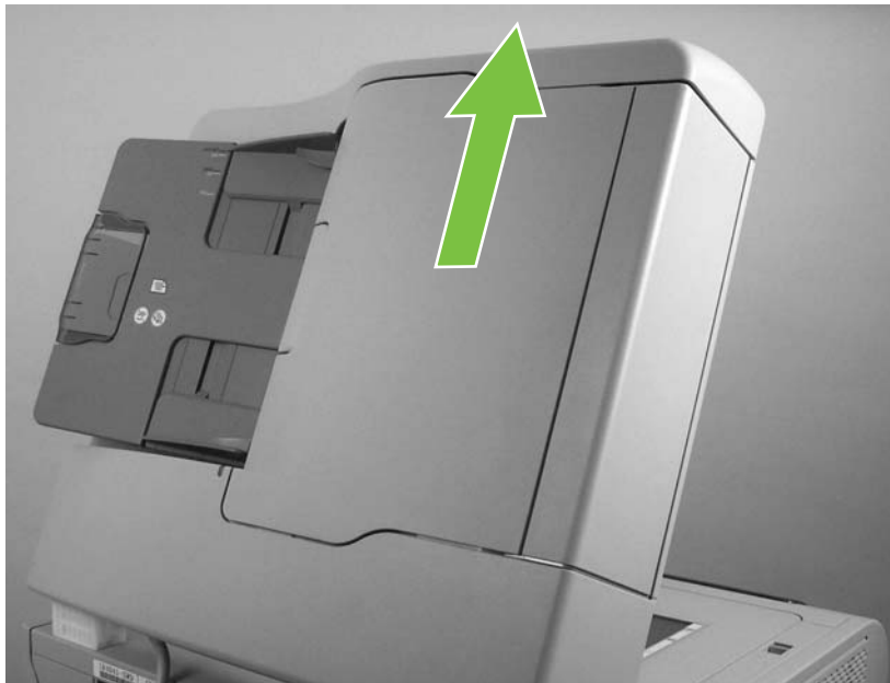
Figure 5-170 Remove the ADF assembly (3 of 3)
