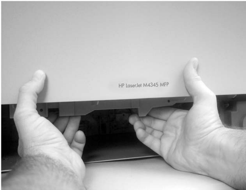
Figure 5-44 Remove the front cover (6 of 7)
