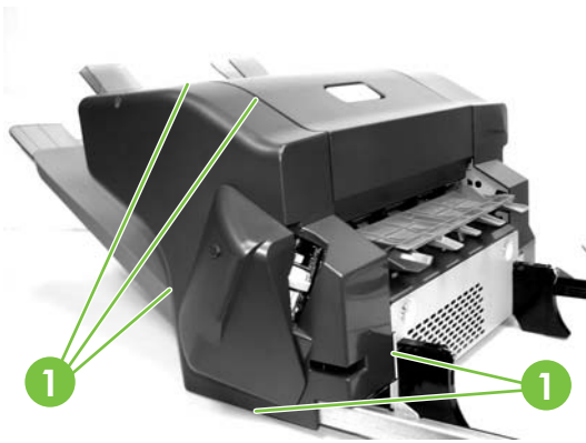
Figure 5-201 Claw locations on front cover
