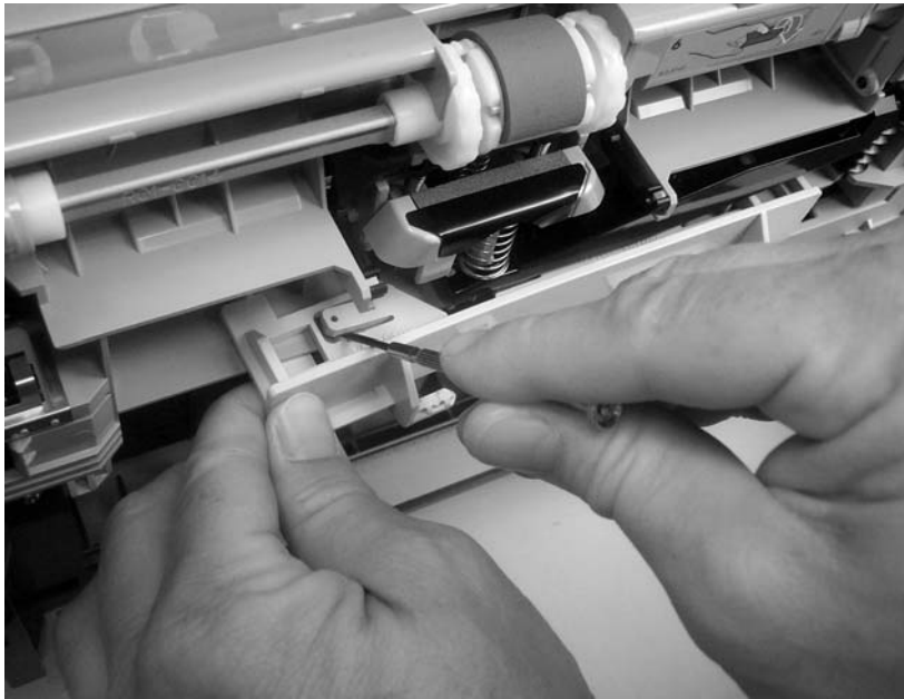
Figure 5-81 Remove the front-cover support (1 of 2)
