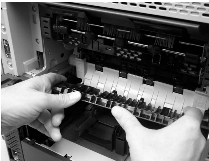
Figure 5-20 Remove the fuser-entrance guide
