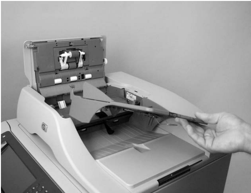
Figure 5-7 Remove the ADF input tray (3 of 3)
