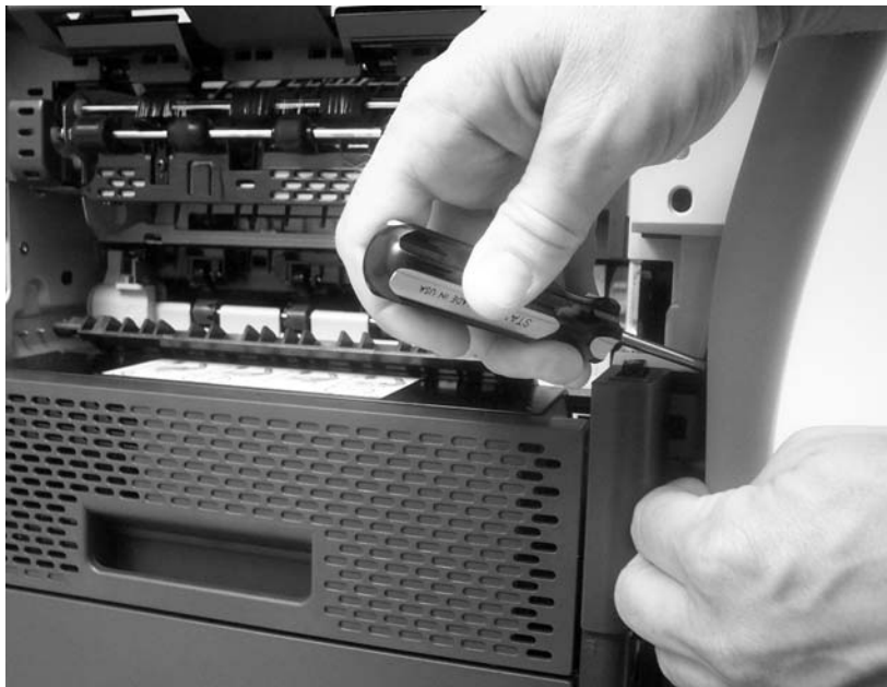
Figure 5-42 Remove the front cover (4 of 7)
