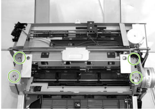
Figure 5-215 Remove the jogger unit (6 of 7)
