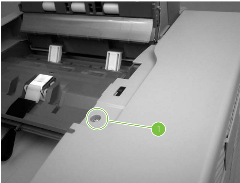
Figure 5-190 Remove the ADF rear cover (1 of 2)
