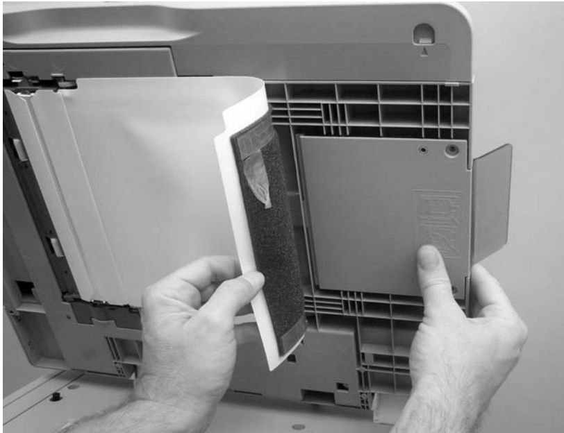
Figure 5-183 Remove the ADF output-bin extension (2 of 2)
