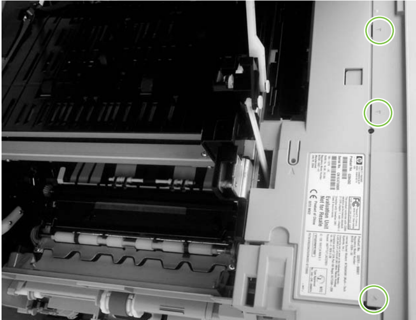
Figure 5-47 Remove the back cover (2 of 3)
