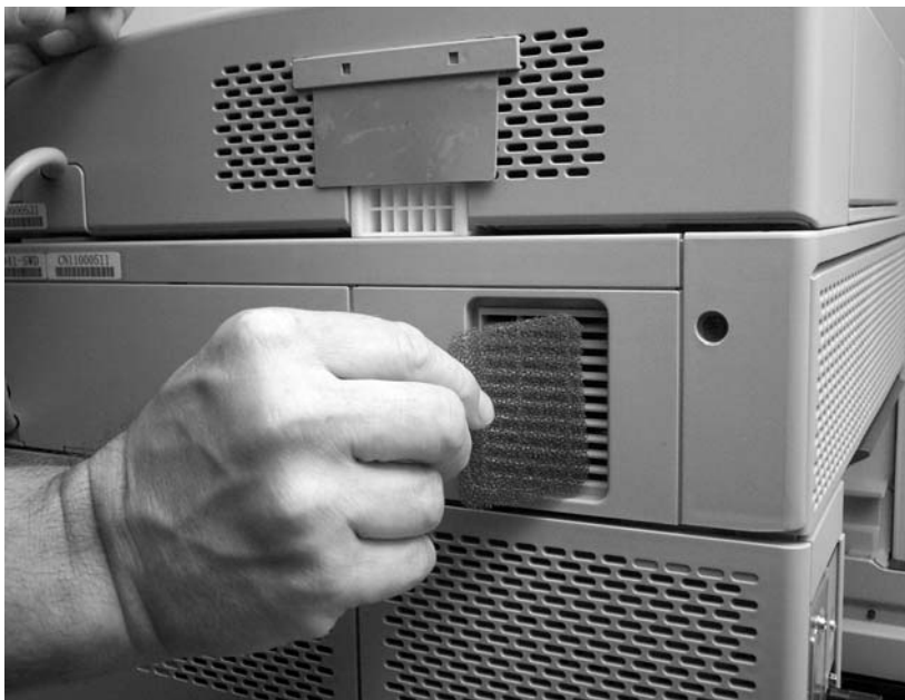
Figure 5-26 Remove the scanner filter (2 of 2)
