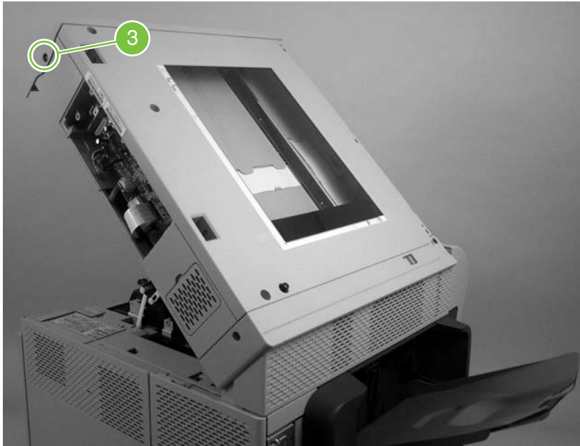
Figure 5-173 Remove the scanner assembly (3 of 8)
