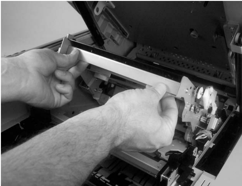
Figure 5-58 Remove the reversing assembly (8 of 8)
