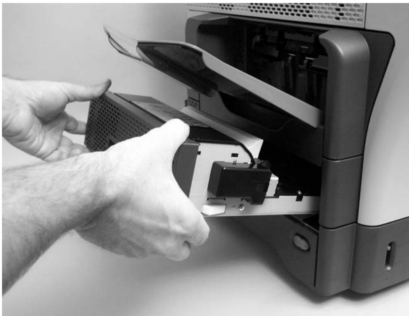
Figure 5-19 Remove the duplex-printing unit (2 of 2)
