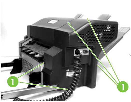
Figure 5-202 Claw locations on rear cover
