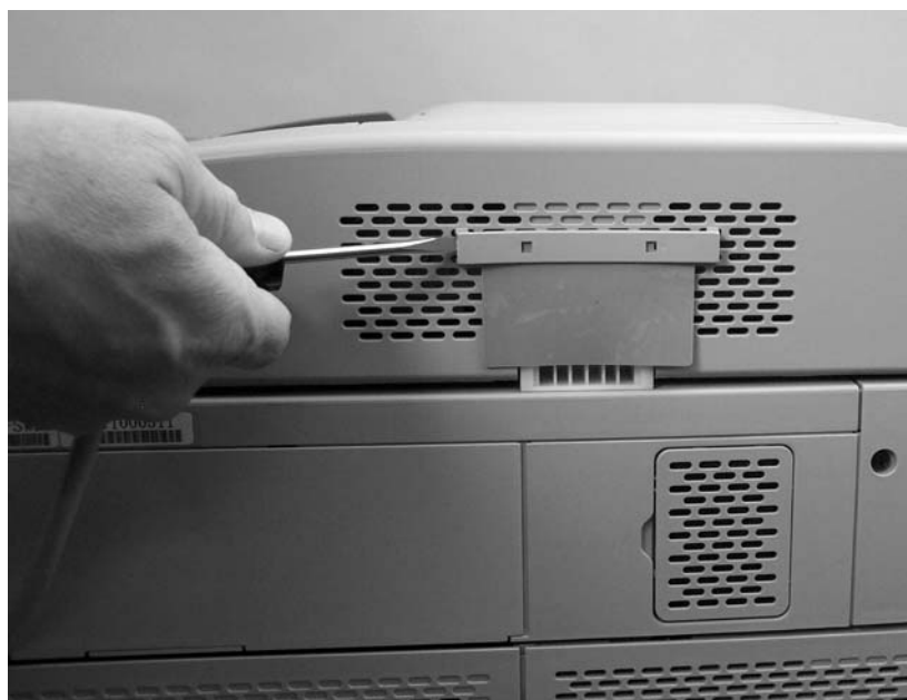
Figure 5-28 Remove the ADF-hinge flap (2 of 3)
