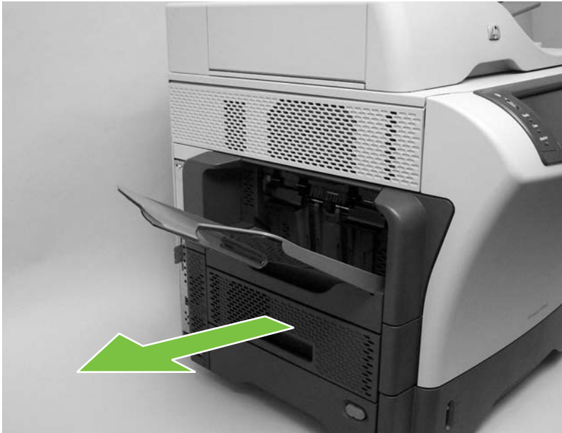
Figure 5-18 Remove the duplex-printing unit (1 of 2)
