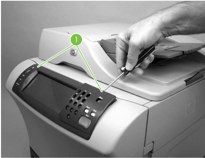
Figure 5-1 Remove the control-panel overlays
