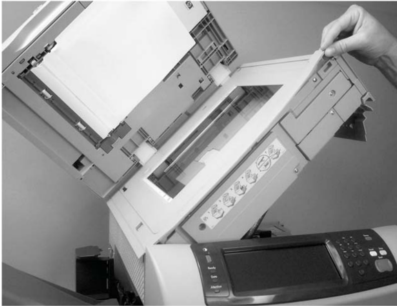
Figure 5-37 Remove the top-cover flatbed flange (1 of 2)
