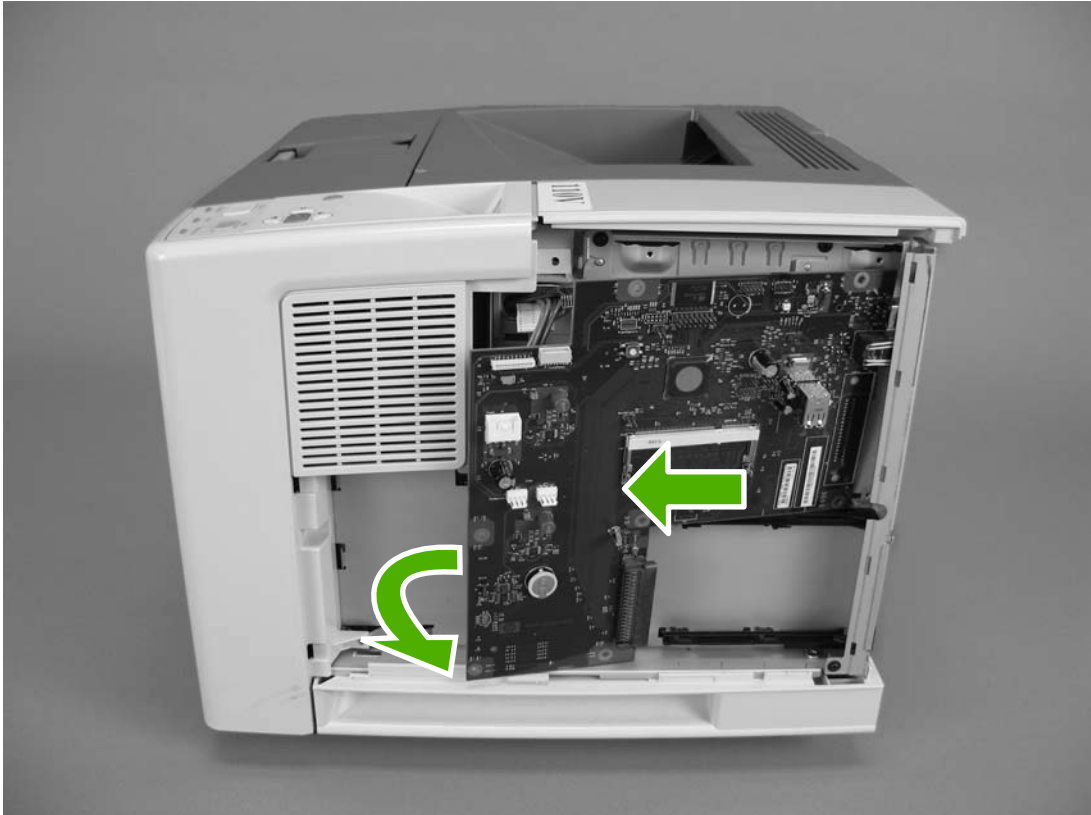
Figure 5-15 Removing the formatter (3 of 3)
